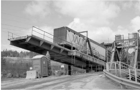
FIGURE 8.3 Biomass delivery truck tilted to unload at the gasification plant. (Source: Photograph by the author.)
