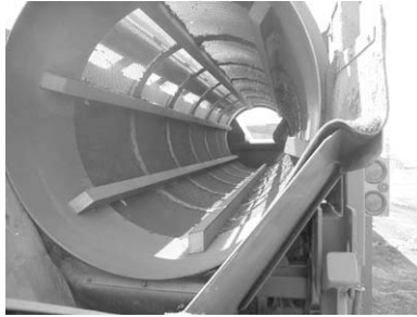
FIGURE 8.13 Portable trammel used in the fuel yard for size classification. (Source: Photograph by the author).
