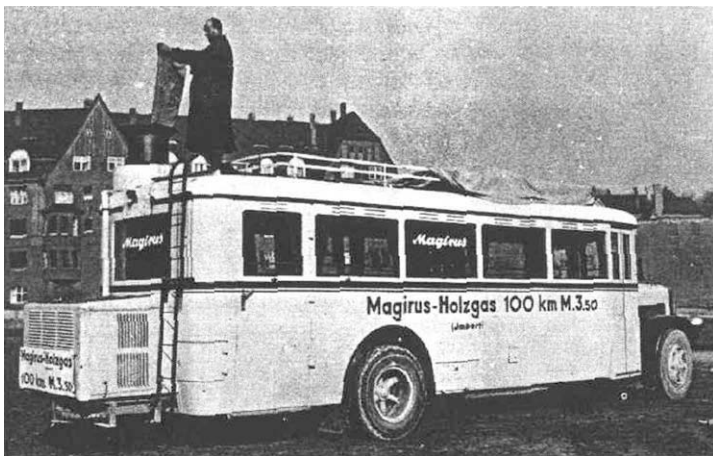
FIGURE 1.2 Bus with an onboard gasifier during the Second World War. (Source: http://www.woodgas.com/history.htm .)
