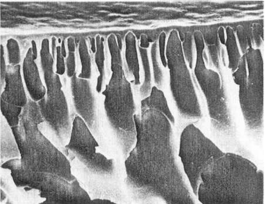
Figure 3.1: Cross-section photomicrograph of asymmetric UF membrane.
