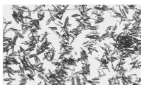
~100 m 2 g -1 1 μm Fe 2 O 3 by precipitation Sicotrans® Red L 2817
