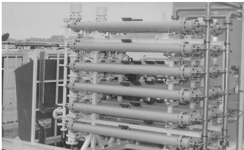
Fig. 2.7 Nitrogen generator for an offshore platform. (Used with permission of Air Products and Chemicals, Inc.).
