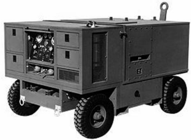
Fig. 2.6: Mobile nitrogen generator. (Used with permission of CvB Company.)
