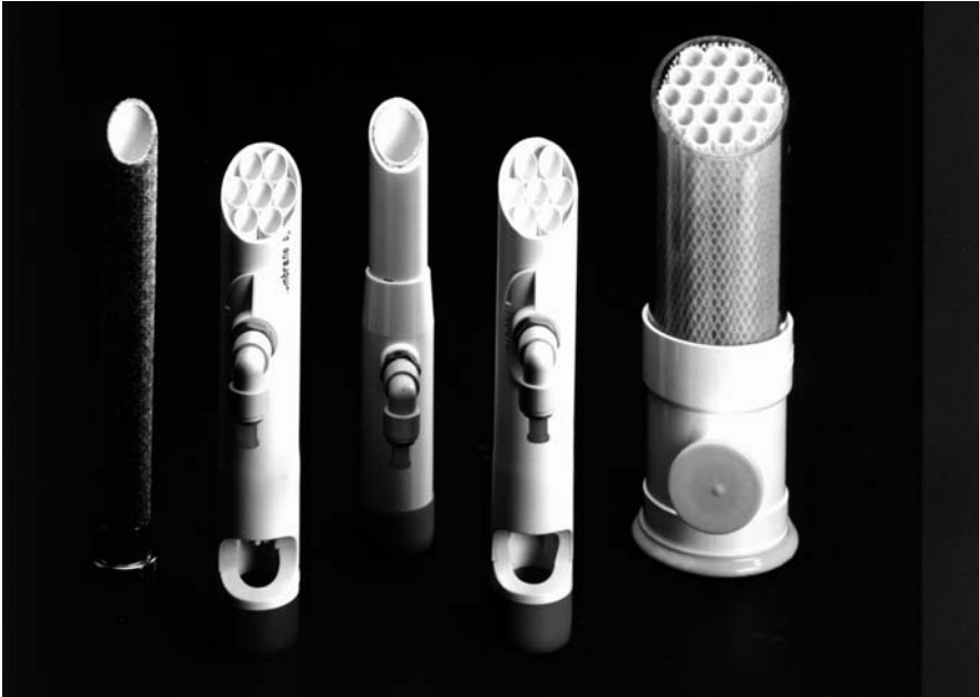
Figure 3.40 Typical tubular ultrafiltration module design. The membrane is usually cast on a porous fiberglass or paper support, which is then nested inside a plastic or steel support tube. In the past, each plastic housing contained a single 2- to 3-cm-diameter tube. More recently, several 0.5- to 1.0-cm-diameter tubes, nested inside single housings, have been introduced. (Courtesy of Koch Membrane Systems)
