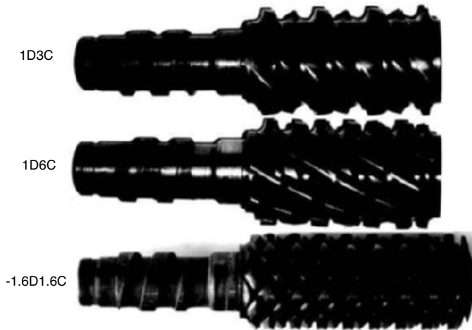
Figure 10.36: Rhomboidal mixing sections studied experimentally.
