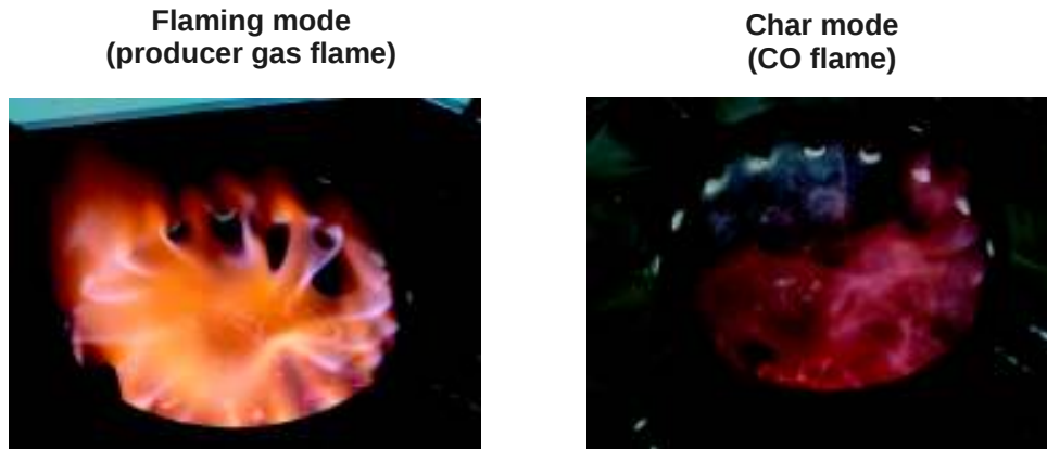
Figure 3.2: Gas phase flame in the stove. Left : Flaming mode. Right : Char mode
