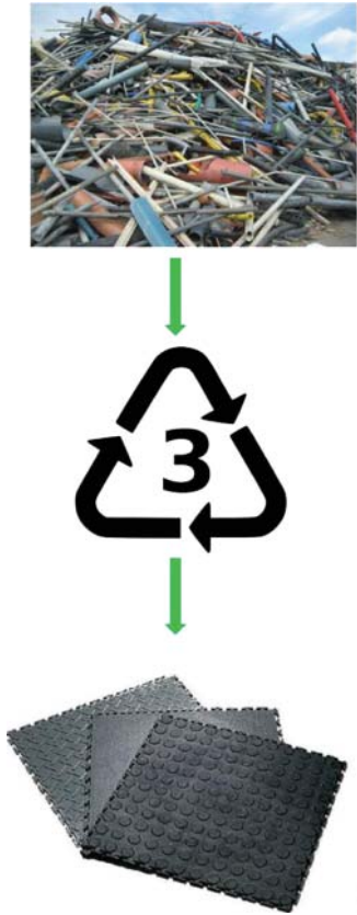
Figure 9.1.4 Recycled PVC used for making plastic floor tiles.
