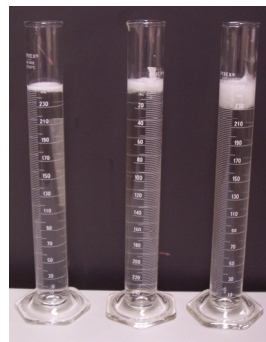
Fig. 18. Unstable test fluids after 1.0 hour test
