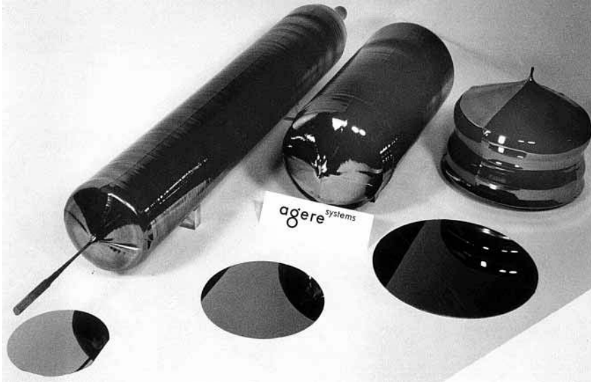
Figure 1.36 Typical silicon ingots. (Courtesy of Agere Systems.)
