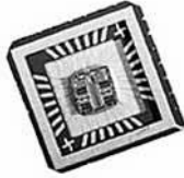
Figure 8.43 Leadless ceramic chip carrier (internal).
