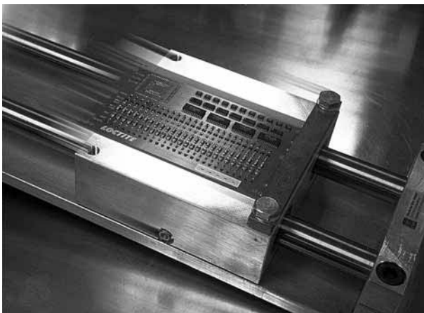
Figure 9.37 Sliding ramp for green strength test.
