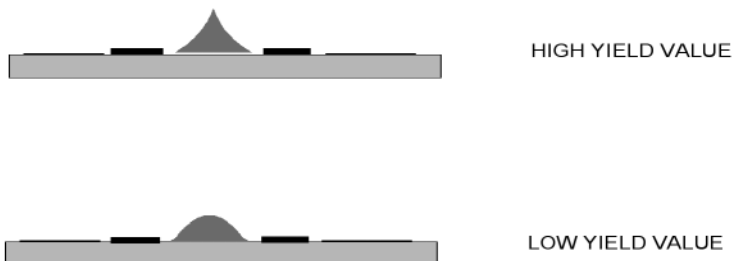
Figure 9.48 Effect of yield point on chip bonder dot profile.
