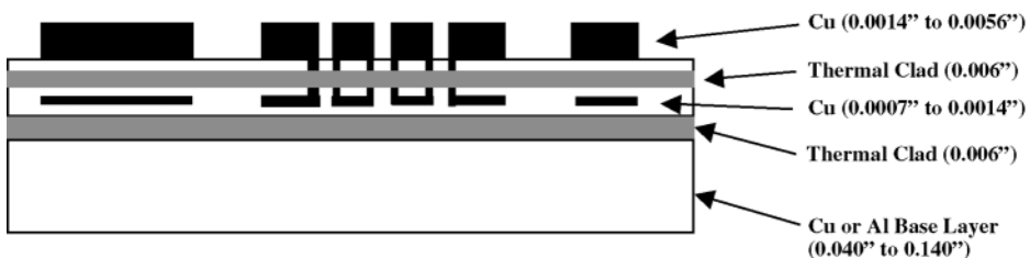
Figure 10.34 Two-layer insulated metal substrate cross section.
