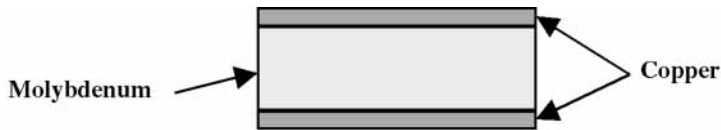
Figure 10.61 Copper-clad molybdenum construction.
