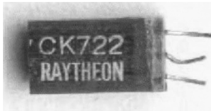
FIGURE 1.5 CK722 is one of the well-known transistors from the 1950s and 1960s. Raytheon introduced this device in early 1953. The CK722 was the first mass-produced germanium alloy junction transistor. Raytheon was the major manufacturer of hearing aid transistors, and those units that were not quite “good enough” for the demanding hearing aid market (i.e., not enough gain or too noisy) were sold to hobbyists as the CK722 (From the Transistor Museum, Jack Ward, curator. With permission. [35]).
