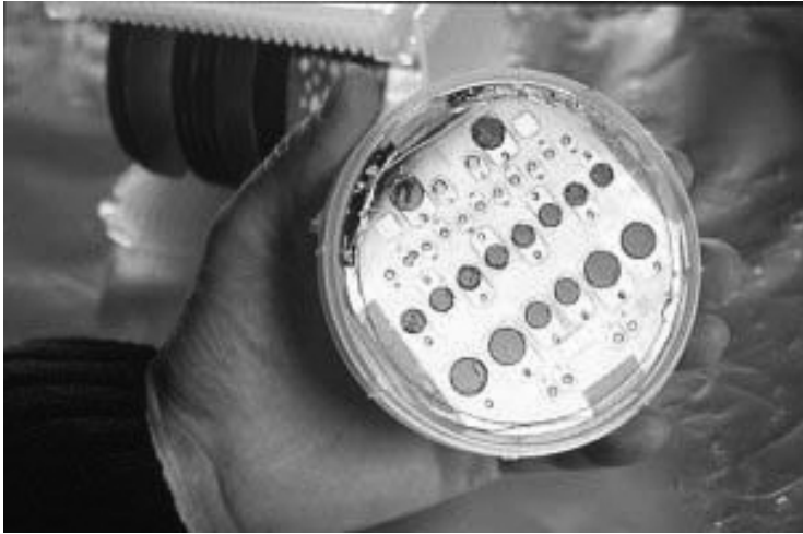
FIGURE 44.12 Fuel cell core architecture on silicon wafer. Each dark dot on the planar layout is a single fuel cell. (From CEA. With permission.)
