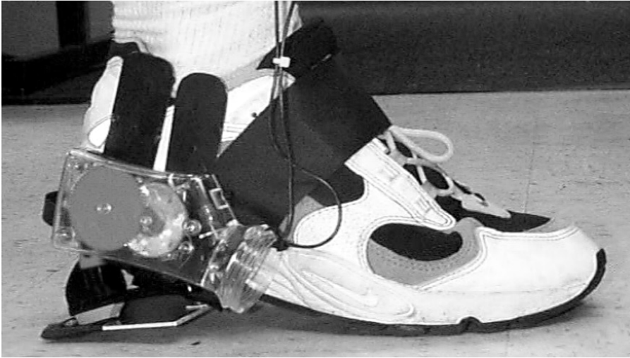
FIGURE 45.10 Rotary generator fit to a shoe for proof-of-concept studies at MIT.
