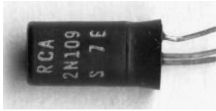
FIGURE 1.4 RCA introduced the 2N109 in 1955 (Germanium PNP Alloy Junction). It was an affordable and reliable germanium audio transistor used in many transistorized radios. In 1956, the 2N109 cost a little over $2 and had dropped to approximately $1 by the early 1960s (From the Transistor Museum, Jack Ward, curator. With permission. [35]).
