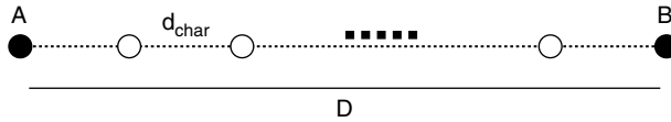
FIGURE 32.1 Relaying nodes are inserted between nodes A and B to reduce the energy of sending a packet from A to B.
