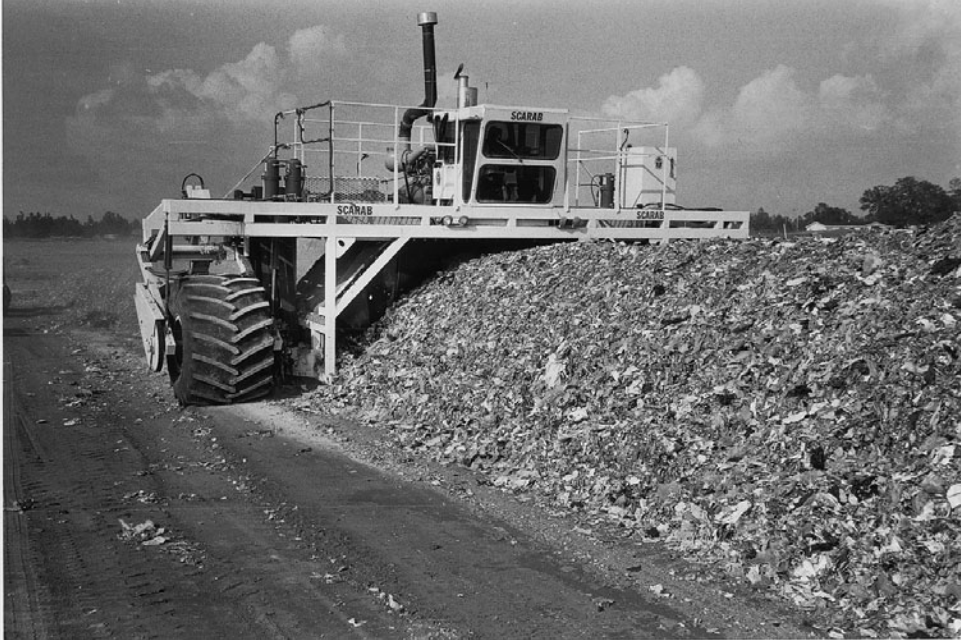
FIGURE 12.7 Self-propelled windrow-straddling composting machine. A rotary drum, not seen within the machine, picks up the material, throws it over the drum, and redeposits it into a windrow ready for subsequent turning.
