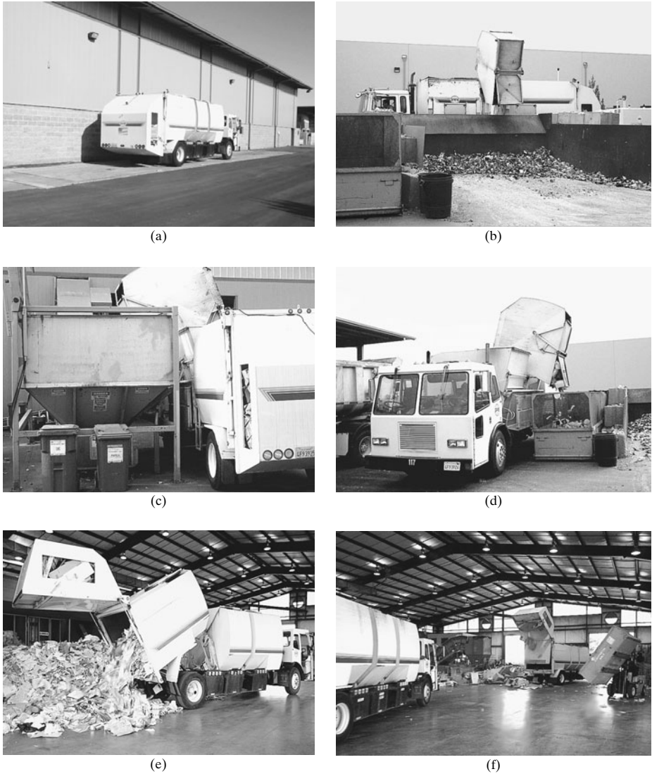
FIGURE 8.11 Procedures associated with vehicle unloading after collection of source-separated materials: (a) weighing of vehicle contents, (b) glass unloading, (c) mixed waste (plastics and cans) unloading into feed hopper, (d) mixed waste unloading into overflow bins if hopper is full, (e) unloading of mixed paper, and (f) unloading of cardboard.
