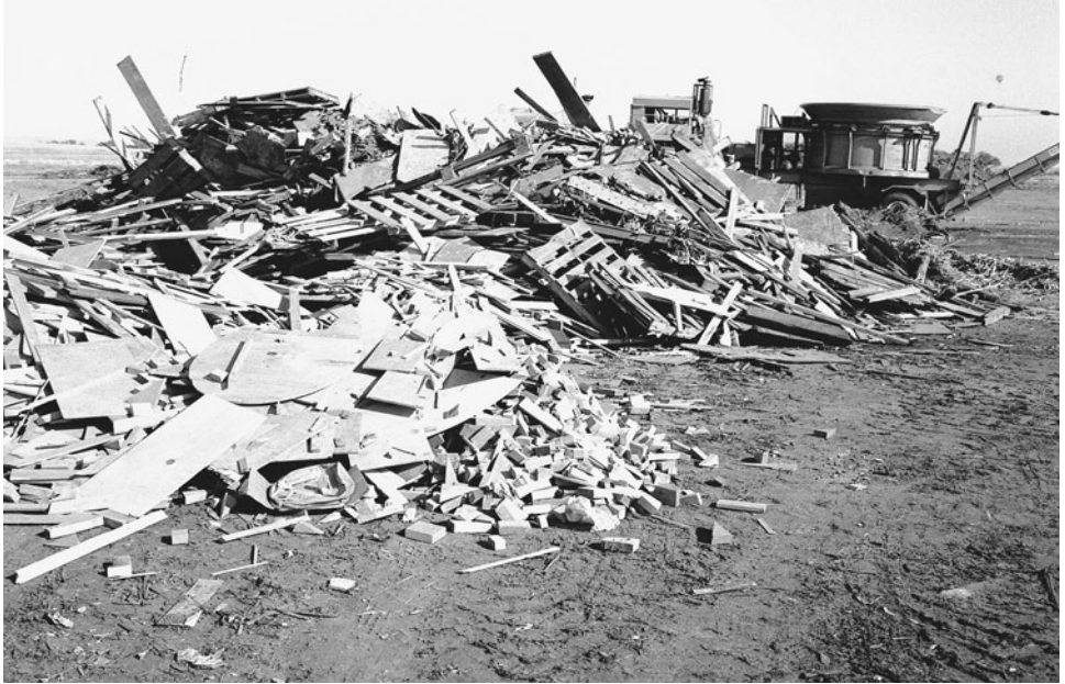
FIGURE 11D.2 Typical wood waste separated for processing. The wood waste in the foreground is from a cabinet shop and the larger pile is from a construction site. The tub grinder used to process the wood waste is shown in the background. The processed waste is sold as a boiler biomass fuel.
