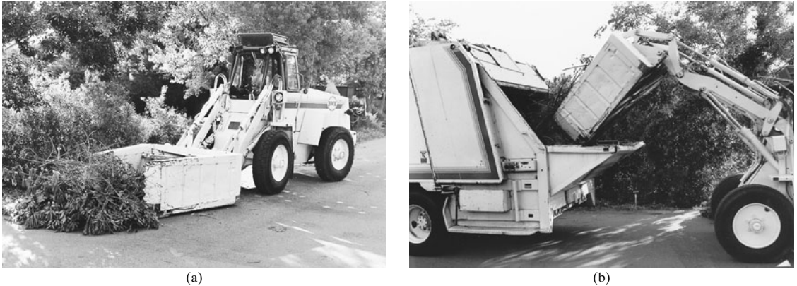
FIGURE 7.10 Collection of noncontainerized yard waste placed in the street by the homeowner. (a) View of claw device mounted on a wheeled tractor used to pick up yard wastes. (b) Modified-compaction-type collection vehicle used in conjunction with claw. The collected yard wastes are hauled to a processing facility to be composted.
