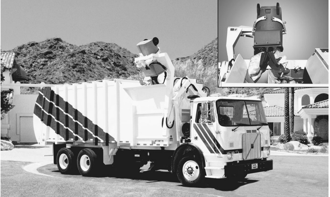
FIGURE 7.2 Typical example of mechanized collection vehicle with mechanical articulated pickup mechanism used for the collection of domestic source separated and comingled waste placed in a dual compartment container (see insert) (courtesy Heil Environmental Industries, Ltd.). The large containers equipped with wheels are brought to the curb by the homeowner. In some locations, helpers are used to bring the loaded containers to the curb, and the homeowner is responsible for returning the container to its storage location.
