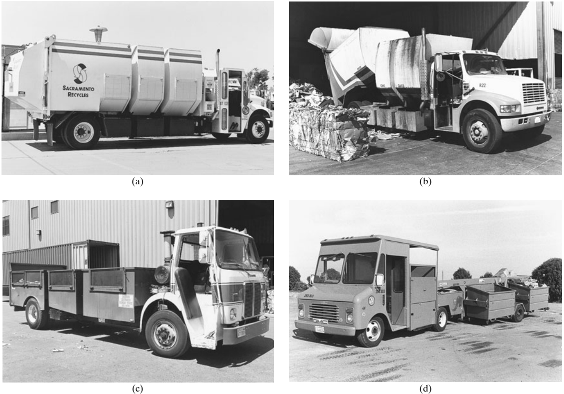
FIGURE 7.9 Typical collection vehicles used for the collection of source-separated waste: (a) stand-up right-hand-drive, side-loaded collection vehicle with three separate compartments, using low collection troughs that are emptied mechanically. (b) Stand-up right-hand-drive open-top side-loaded collection vehicle. (c) Stand-up right-hand-drive side-loaded collection vehicle with three low-loading height compartments. (d) Stand-up-drive collection vehicle with mobile containers. When the containers are filled, they are emptied with a forklift.
