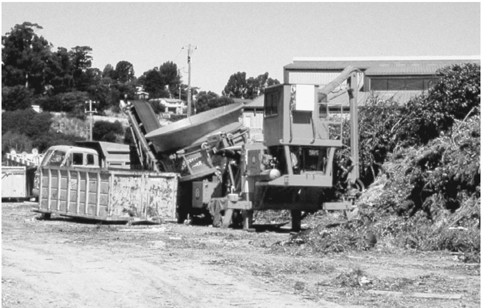
FIGURE 11D.3 Tub grinder used to process wood, trees, brush, and other green waste. Processed wood is sold as a boiler biomass fuel, and green waste is typically used for the production of compost.
