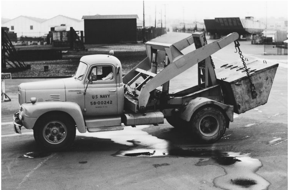
FIGURE 7.12 Hoist-truck mechanism mounted on truck frame. Photo was taken in the 1960s at a naval installation. Although the truck style has changed, the hoist mechanism is essentially unchanged and is still used today.
