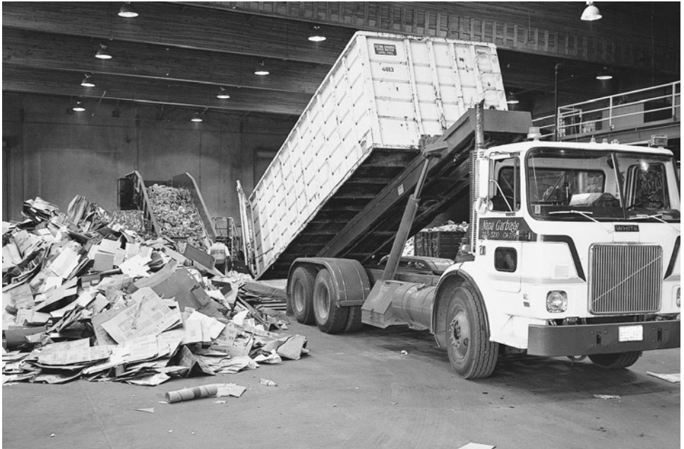
FIGURE 7.13 Truck with tilt-frame loading mechanism used with large debris boxes, sometimes called roll-off containers . Contents of debris box is being unloaded at a combined recycling and transfer facility.
