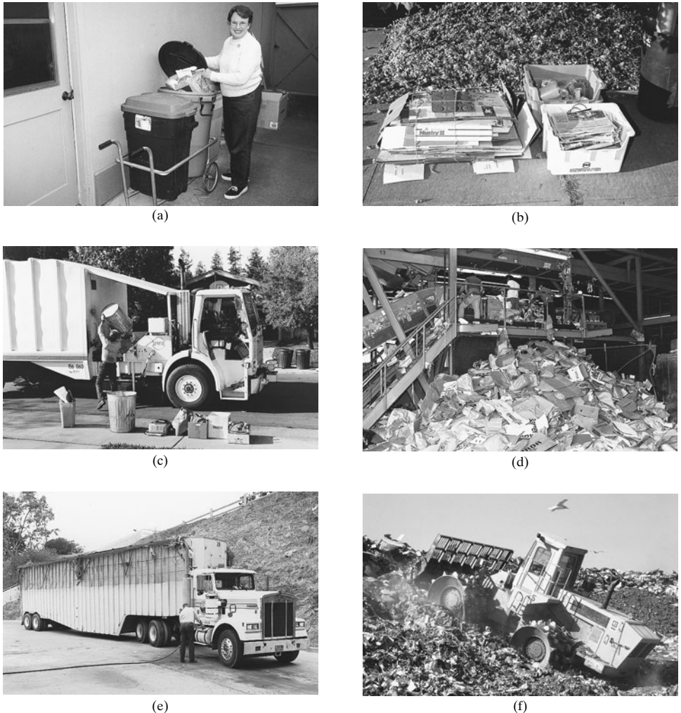
FIGURE 1.2 Views of the functional activities that comprise a solid waste management system: (a) waste generation; (b) waste handling and separation, storage, and processing at the source; (c) collection; (d) separation, processing, and transformation of solid waste; (e) transfer and transport; and (f) disposal.
