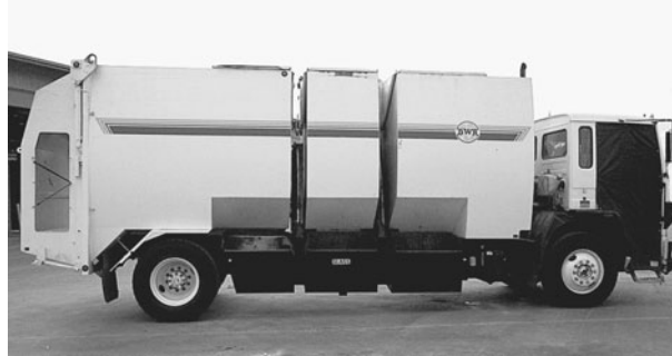
FIGURE 8.4 Collection vehicle used for the collection of residential source-separated materials. The first compartment behind the cab is for mixed plastics and cans, the middle compartment is for glass, and the last compartment is for mixed paper. The bubble behind the last compartment is for the collection of flattened and bundled cardboard.
