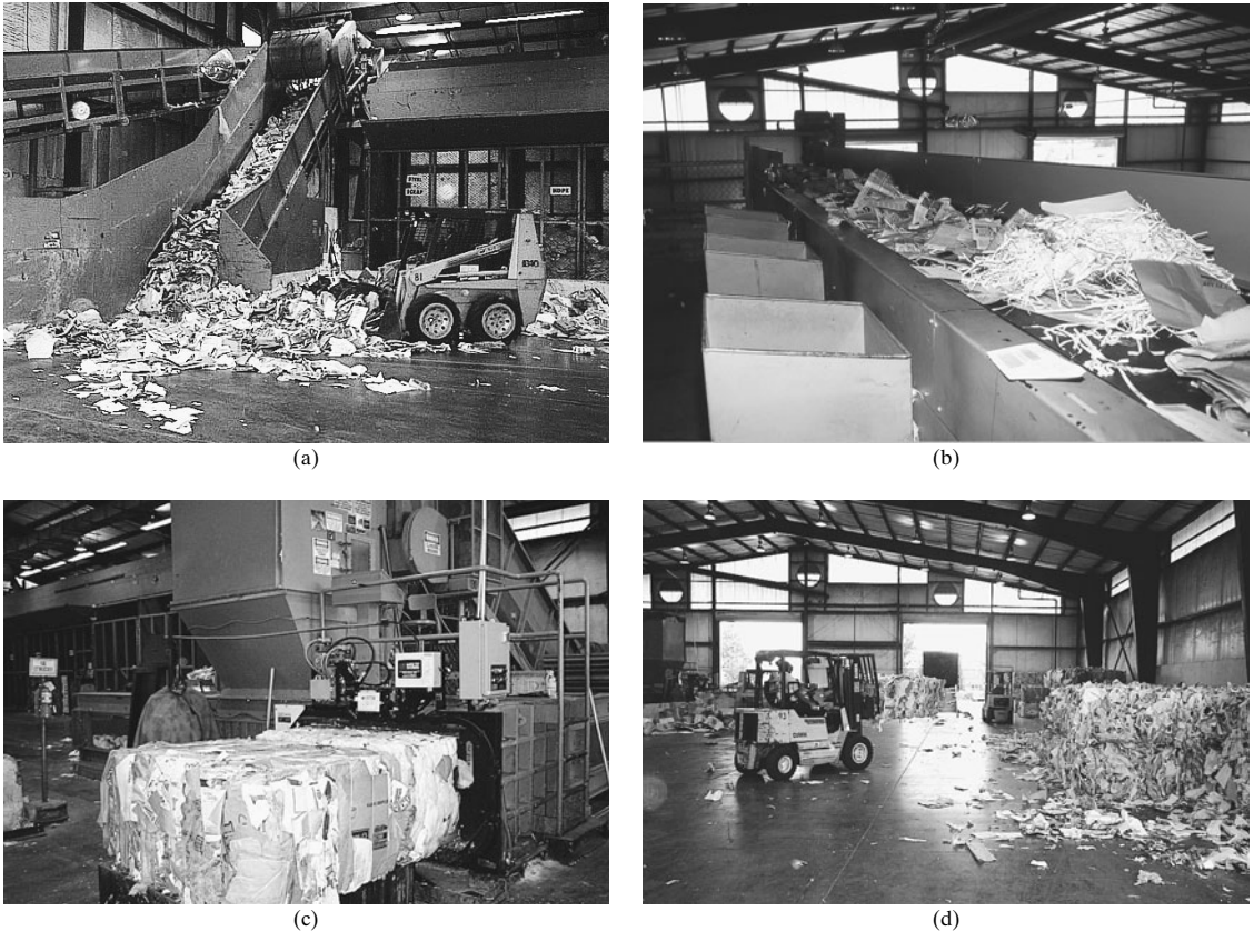
FIGURE 8.13 Steps in processing source-separated paper: (a) mixed paper being pushed onto inclined conveyor using skid steer loader, (b) elevated pull-back sorting belt and chutes leading to bulk material storage bins located below, (c) baler with paper bales being produced, and (d) paper bales being stored within the facility.
