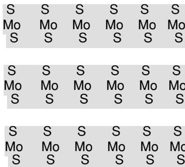
17.4. Molybdenum disulfide is composed of covalently bonded sheets that are weakly bonded to each other.
