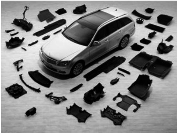
Figure 1. Environmentally friendly polymer materials in automobile manufacturing. (Reproduced with permission from Daimler © Daimler AG.)
