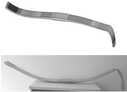
Figure 11. Tension leaf spring made from glass-fiber-reinforced plastics (Schürmann and Keller, 2010).
