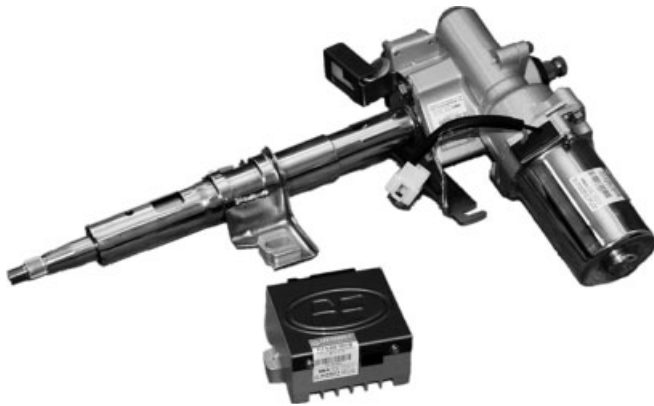
Figure 21. Production C-EPS system. (Reproduced with permission from Zhuzhou Elite Tech Corporation.)
