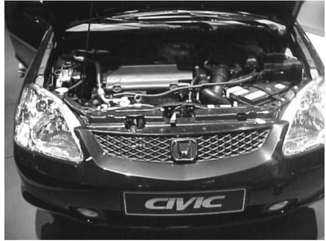
Figure 26. Increase distance from bonnet to still structures.
