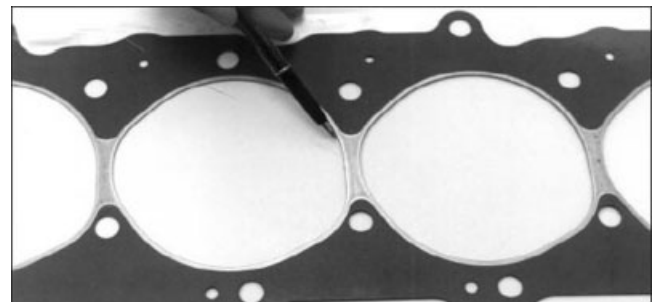
Figure 12. Typical cylinder head gasket used in a gasoline engine.
