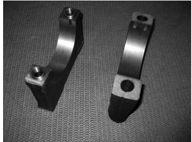
Figure 4. Heavy-duty diesel main bearing cap comparison: machined-ductile iron cap with ring dowel locators (left) and fractured-CGI cap (right).
