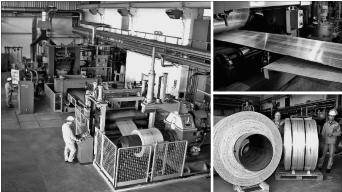
Figure 3. Twin-roll casting plant of the MgF Magnesium Flachprodukte GmbH in Freiberg. (From Kawalla et al. (2008). Reproduced by permission of Croatian Metallurgical Society.)
