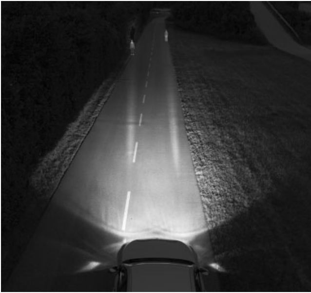
Figure 7. Far-infrared night vision systems with active light beam. (Reproduced by permission of BMW AG.)
