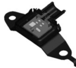
Figure 16. Electronic satellite sensor. (Reproduced by permission of Denso Corporation.)
