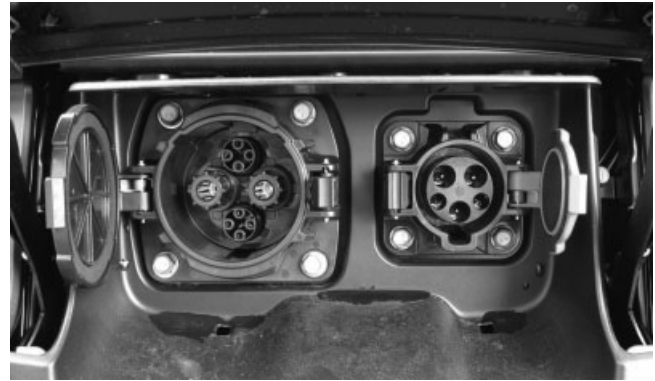
Figure 12. CHAdeMO DC (left) and type 1 AC (right) inlets on a Nissan Leaf vehicle. (Reproduced with permission from Peter Van den Bossche. © Peter Van den Bossche.)
