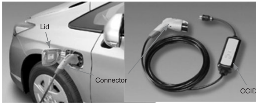
Figure 6. Charging system components. (Reproduced with permission from Society of Automotive Engineers Japan (2011). © Society of Automotive Engineers Japan.)
