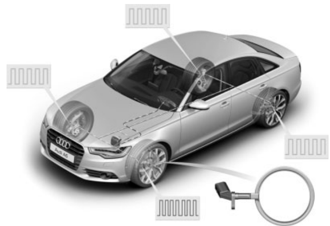
Figure 25. System configuration for second-generation indirect TPMS in an 2012 Audi A6.
