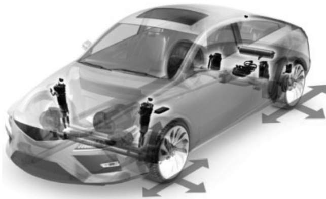
Figure 2. Vehicle with electronic air suspension and electronic adjustable damper. (Reproduced by permission of Continental.)
