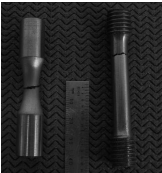
Figure 7. Example failed gray iron fatigue (left) and tensile (right) test specimens.
