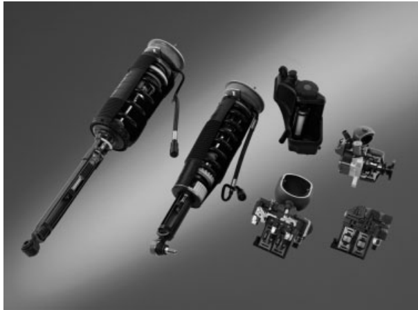
Figure 10. ABC chassis components (Wiesinger). (Reproduced by permission of Daimler.)
