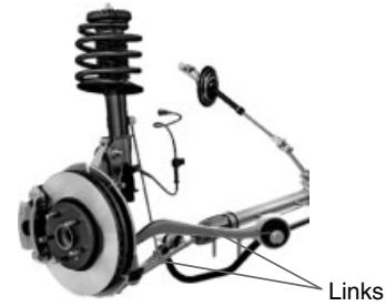
Figure 15. Strut front suspension with two lower suspension arms.
