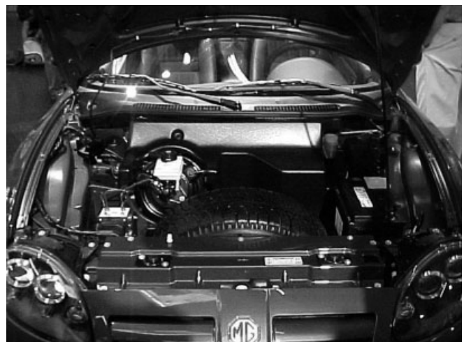
Figure 27. Engine at the back (trunk) would help to increase deformation distances.
