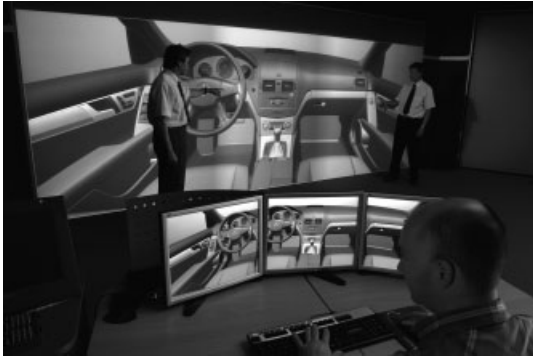
Figure 12. Virtual validation of the interior at the power wall. (Reproduced by permission of Daimler AG.)
