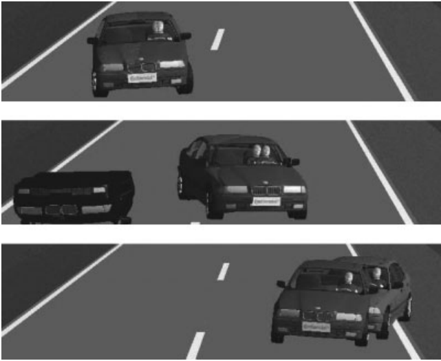
Figure 17. Animation of an emergency evading use case. The vehicle with conventional ESC is skidding off the track and the vehicle with ESC and ARK and predictive handling control remains on track. (Reproduced by permission of Continental.)
