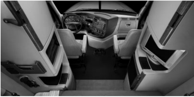
Figure 3. Injection molded storage compartments and dashboard, of a Freightliner Cascadia. (Reproduced with permission from Daimler © Daimler AG.)
