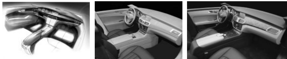
Figure 5. Rendering and clay models of the interior. (Reproduced by permission of Daimler AG.)
