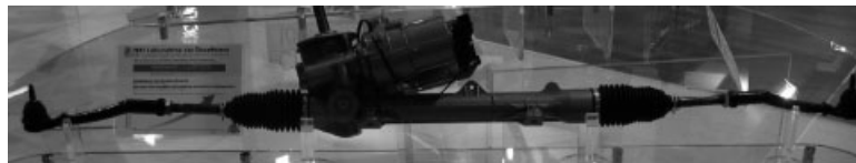
(c) Electric motor at the pinion
