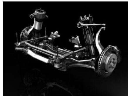
Figure 2. Four-corner air suspension system—Jaguar XJ front suspension. (Reproduced by permission of Jaguar Land Rover.)
