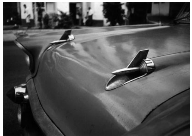
Figure 2. Example of vehicle designed without pedestrian protection requirements. (Photo reproduced by permission of Carlos Arregui.)
