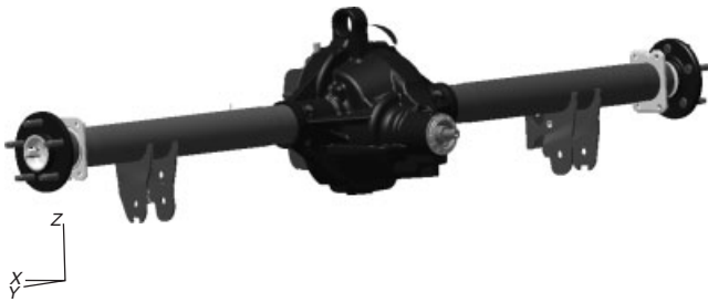
Figure 2. Cast center-style beam axle.
