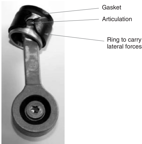
Figure 10. Articulated compressor piston. (Reproduced with permission from WABCO.)
