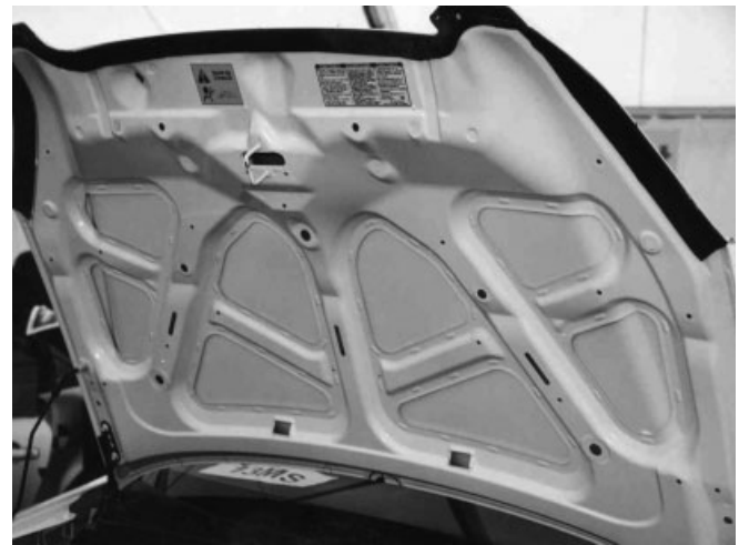
Figure 30. Energy management in bonnet structure.
