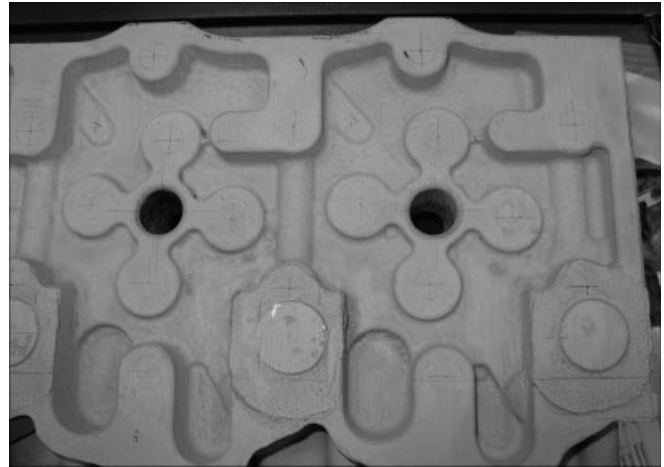
Figure 11. Conventional casting geometric qualification using markup technique.
