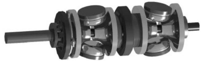
Figure 22. Speed ratio changing diagram: tilting the rollers changes the ratio between the outer driving disks and the center-driven disks. (From Tanaka, 2000. Reproduced by permission of Corona Publishing Co. Ltd.)
