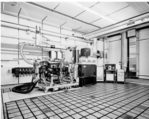
Figure 3. An AC dynamometer-equipped engine test cell containing a large cast-iron tee-slotted bedplate that is supported on air-springs, allowing multiple configurations of test equipment. Engine supported within a wheeled trolley allowing extensive prerigging outside the cell. Low level, rectangular “purge duct” can be seen on the right hand side of the photo next to an, circular section, exhaust dilution and extract duct. (Photograph reproduced by permission of AVL List GmbH.)
