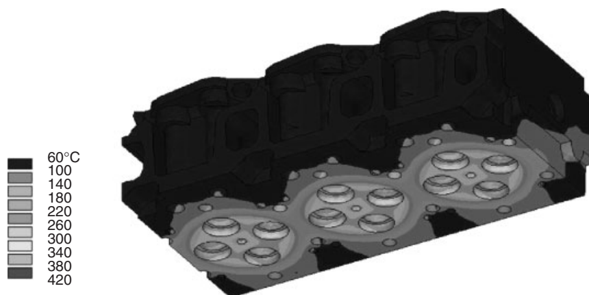
Figure 8. Example of cylinder head peak fire-deck temperature predictions from thermal FEA.
