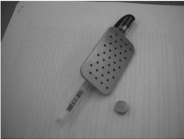
Figure 4. A 10-Ah rechargeable, Zn-air cell Revolt technology.
