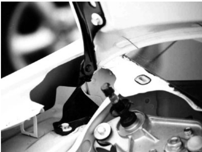
Figure 25. Deformable windshield wiper axis.
