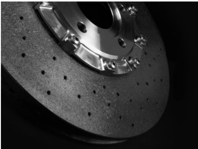
Figure 2. CF/SiC Brake disk. (Reproduced by permission of SGL Carbon GmbH.)
