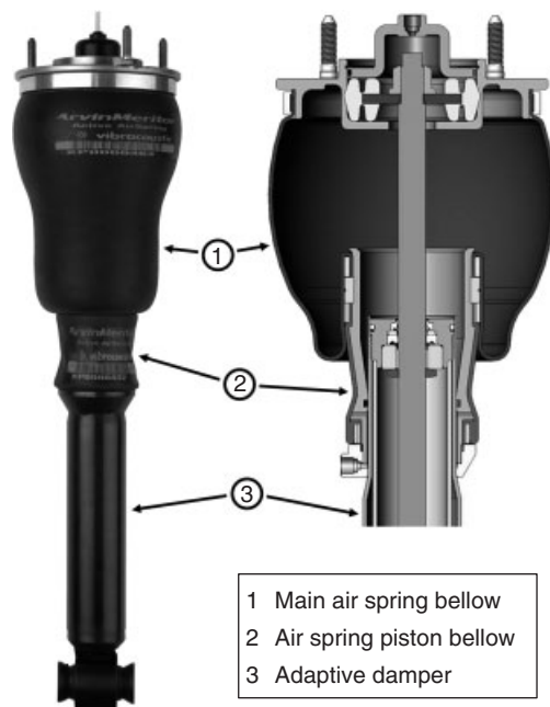
Figure 4. Continuously variable air spring module. (Reproduced by permission of Meritor, Inc.)
