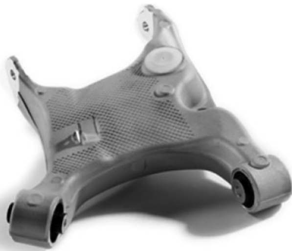
Figure 34. Example: BMW X5 RLCA: VRC/PRC with sand core (hollow cast).
