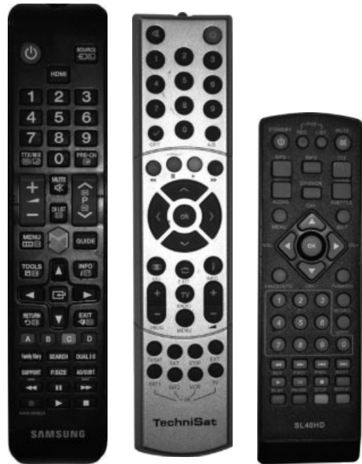
Figure 4. Examples of stereotypes with high affordance showing the “five-way toggle” stereotype of TV/Sat remote controls (Samsung, TechniSat; Comaq). (Reproduced with permission of Stefan Becker. © S. Becker.)
