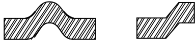
Figure 24. Embossed metal for added stress in the combustion area. (Courtesy of Federal Mogul.)
