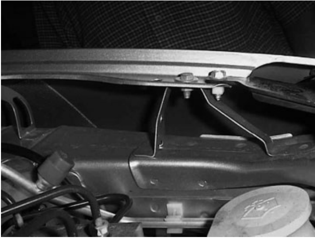
Figure 24. Deformable elements in case of wing impact.
