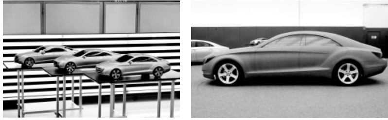
Figure 7. Samples of painted exterior clay models and the chosen model. (Reproduced by permission of Daimler AG.)
