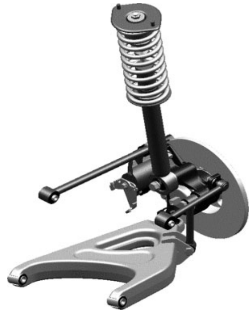
Figure 9. View of a multilink rear axle. (Reproduced from World Auto Steel. © World Auto Steel.)
