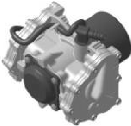
Figure 6. Securing boost vacuum by electric pump.
