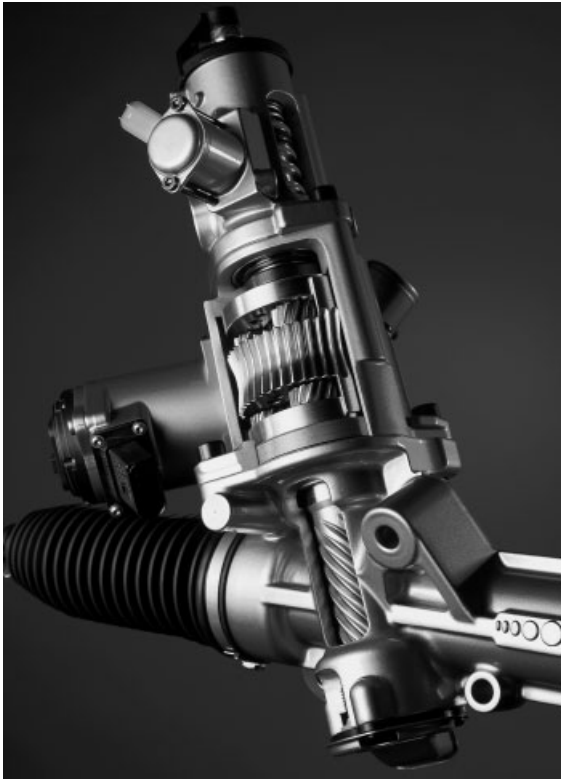
Figure 5. Electric superimposed steering. (Reproduced by permission of EBM-Papst.)
