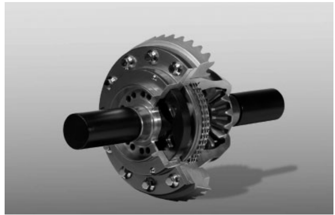
Figure 8. The hydraulic pump limited slip differential. (Reproduced by permission of Joe Palazzolo.)
