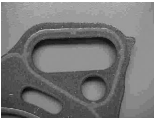
Figure 17. Screen printing. (Compliments of LFP Technologies.)
