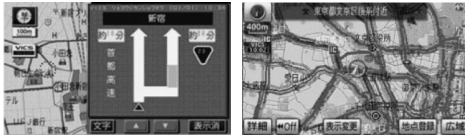
Figure 16. VICS simplified image and superimposition on the map. (Reproduced with permission from Aisin AW Co. Ltd.)
