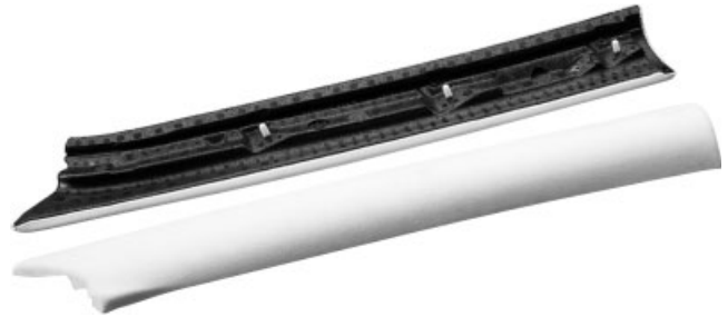
Figure 16. Polypropylene monomaterial composite with TPO skin. (Reproduced with permission from Taracell.)
