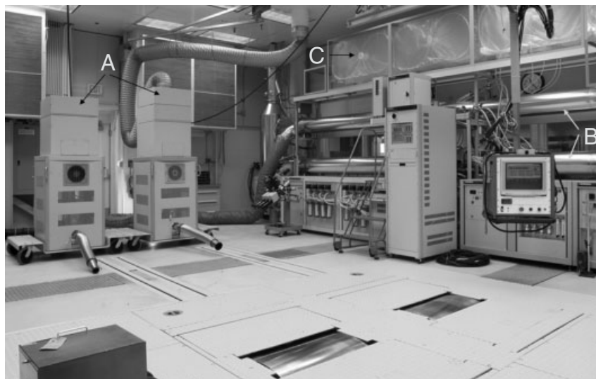
Figure 2. Chassis dynamometer test cell. “A” marks the remote mix “tees” for gasoline and diesel vehicles. “B” denotes the dilution tunnels that run along right-hand wall. And “C” shows the Teflon bags for integrated sampling.
