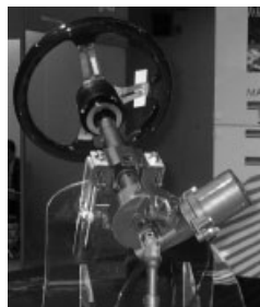
(e) Electric motor rectangular to the upper part of the steering column
