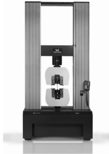
Figure 34. Instron with mechanical jaws set for tensile test. (Photo courtesy of Instron®.)
