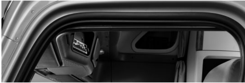
Figure 7. Exdruded elastomer door sealing of a Freightliner-Cascadia. (Reproduced with permission from Daimler © Daimler AG.)
