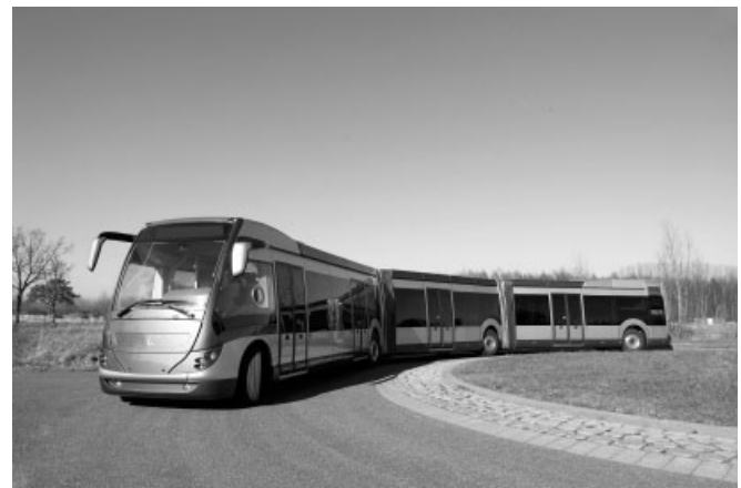
Figure 9. Phileas high tech bus on a dedicated guide way (Phileas, 2011). (Reproduced by permission of VDL Bus & Coach bv.)
