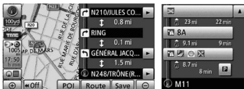
Figure 9. Turn by turn list and Simplified highway map. (Reproduced with permission from Aisin AW Co. Ltd.)
