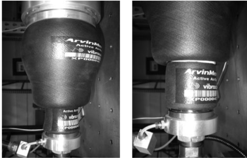
Figure 8. Air spring with variable effective area. (Reproduced by permission of Meritor.)
