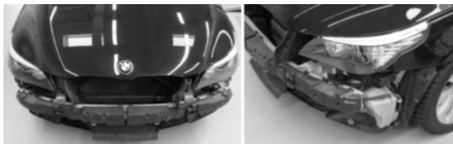
Figure 11. Energy-absorbing element front, cross beam bolted to the side member (BMW 5 series, type E60, European model).
