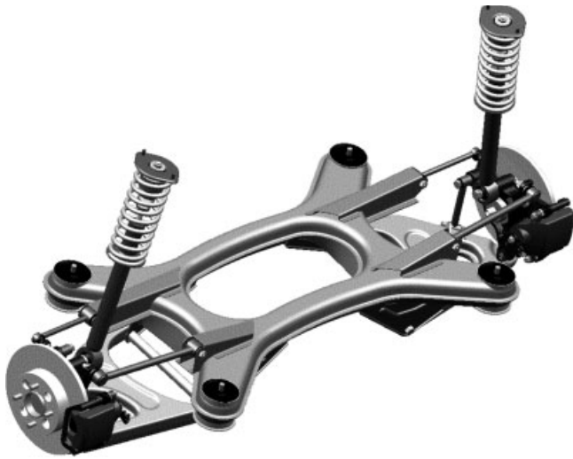
Figure 7. Multilink rear axle. (Reproduced from World Auto Steel. © World Auto Steel.)
