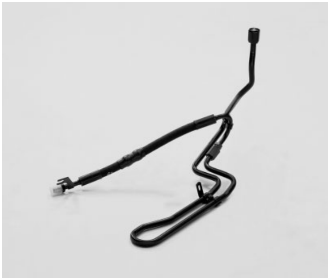
Figure 11. Typical expandable automotive line with average complexity (Johanning, Baum, and Wurmman, 2009). (Reproduced by permission of Heiko Baum.)
