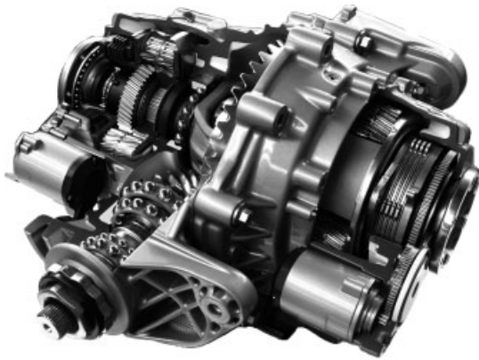
Figure 21. A cutaway display of an entire rear axle. (Reproduced by permission of Joe Palazzolo.)
