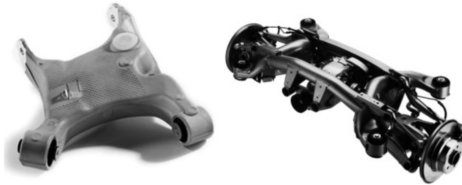
Figure 23. Four-point suspension arm. (Reproduced with permission from ZF.)
