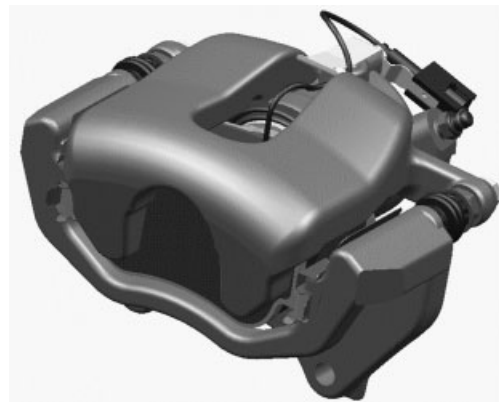
Figure 4. Asymmetrical disk brake. (Reproduced with permission from TRW.)
