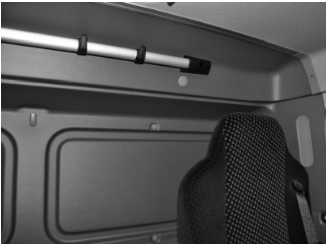
Figure 12. Mercedes Benz Atego thermoformed rear wall interior trim. (Reproduced with permission from Daimler © Daimler AG.)
