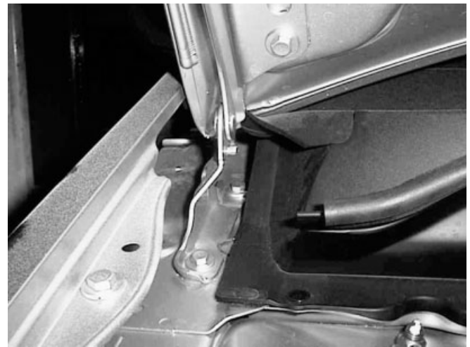
Figure 23. Deformable hinges in case of direct impact.
