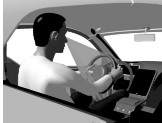
Figure 2. Model-based check of instrumentation readability (Lorenz and Remlinger, 2011). (Reproduced by permission of VDI Wissensforum GmbH.)
