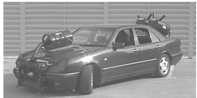
Figure 12. Vehicle with minimum or residual noise by means of the use of intake and exhaust jumbo mufflers and engine encapsulation. (Reproduced by permission of IDIADA.)
