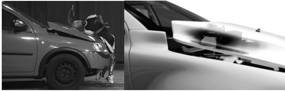
Figure 20. Pop-up bonnet. (Reproduced with permission from Autoliv. © Autoliv.)
