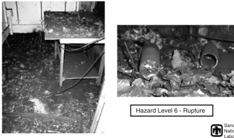
Figure 1. Battery failure testing at Sandia National Laboratory. (Reproduced from Roth, Wunsch, and Orendirff, Sandia National Laboratory.)
