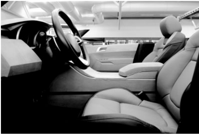
Figure 9. Interior seating buck clay model shown with seats partly dressed. (Image used with the kind permission of Jaguar Land Rover 2013.)
