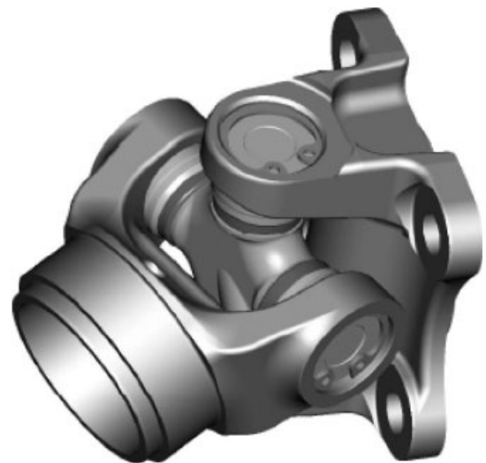
Figure 3. Cardan joint application example: propshaft for light commercial vehicle.
