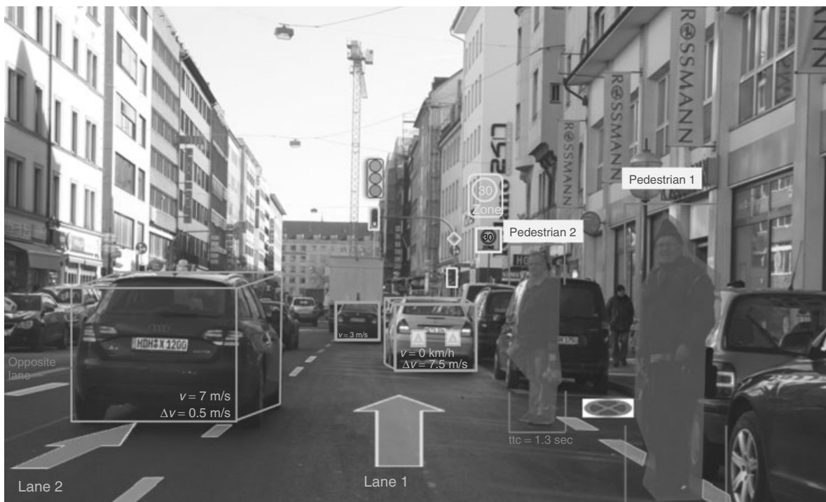
Figure 3. Detection and classification of objects via video camera. (Reproduced by permission of BMW AG.)
