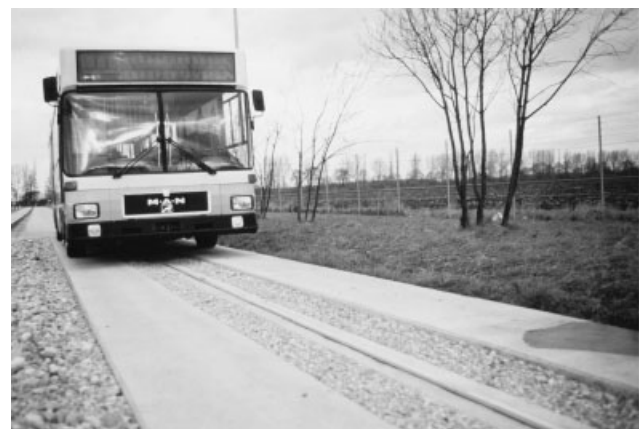
Figure 6. Automated driving bus using a guide wire in the ground of the driving way. (Reproduced by permission of MAN.)
