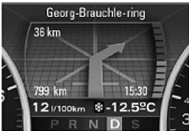
Figure 10. Route guidance example using a secondary display. (Reproduced with permission from Aisin AW Co. Ltd.)
