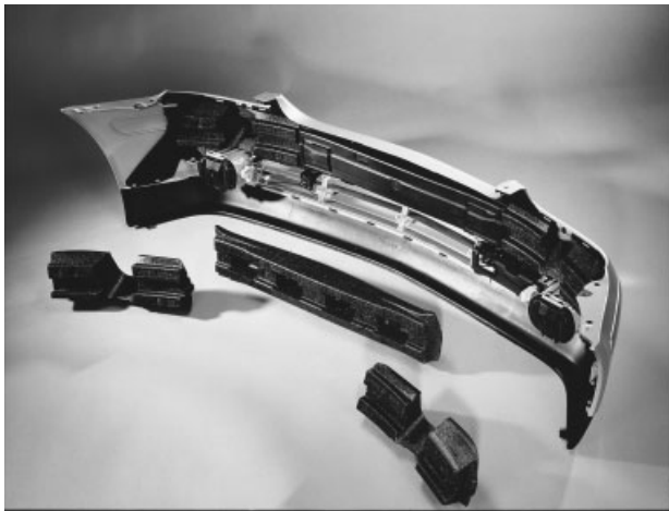
Figure 15. Bumper with EPP inserts. (Reproduced with permission from Ruch Novaplast © Ruch Novaplast.)
