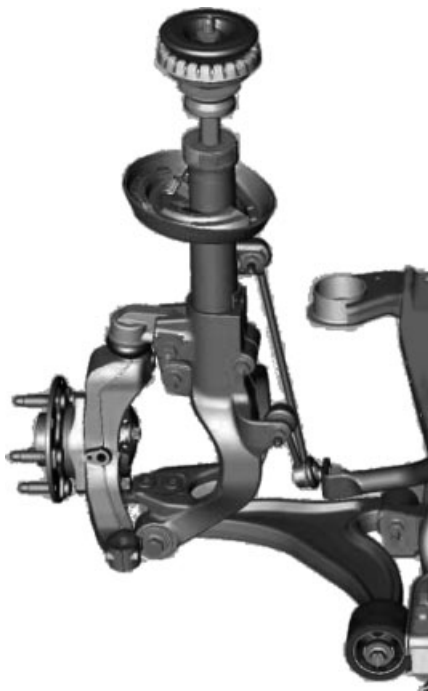
Figure 17. McPherson suspension with revolute joint.
