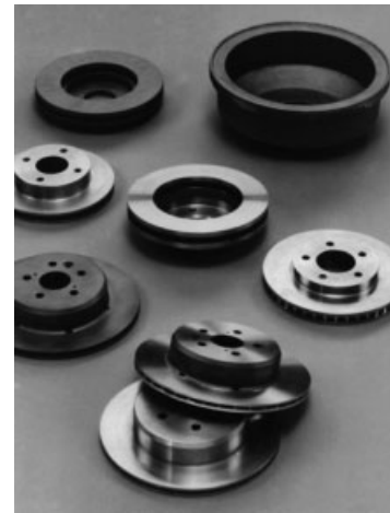
Figure 2. Particulate MMCs for use in brake drums and brake rotors, as a replacement for cast iron (courtesy of D. Miracle). The high wear resistance and thermal conductivity coupled with 50–60% weight savings, make MMCs quite attractive for this application. (Reproduced from Metal Matrix Composites , 2006, N. Chawla and K.K. Chawla. With kind permission of Springer Science+Business Media.)
