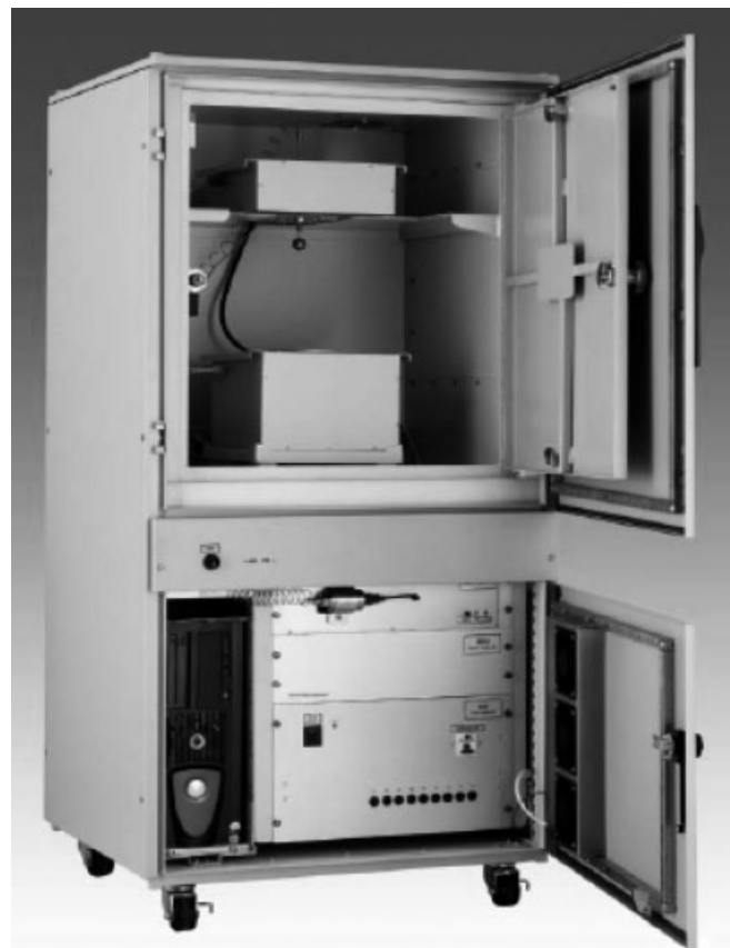
Figure 3. An accelerating rate calorimeter. (Reproduced by permission of Thermal Hazard Technology (2012).)
