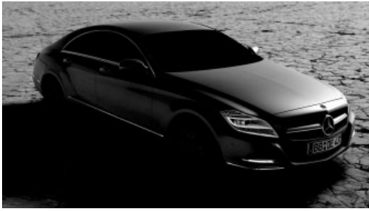
Figure 15. VR validation of Class-A surfaces, colors, and equipment versions. (Reproduced by permission of Daimler AG.)
