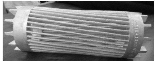
Figure 2. Rotor squirrel cage of an induction motor.
