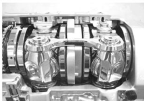
Linkage to hold power roller
