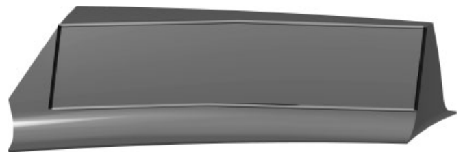
Figure 14. Face-hobbed tooth surface.
