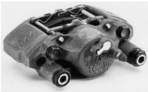
Figure 6. Semi-integrated disk brake. (Reproduced with permission from TRW.)
