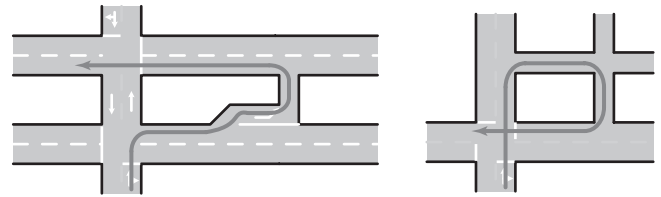
Figure 11. Michigan lefts and P-turns. (Reproduced with permission from Aisin AW Co. Ltd.)
