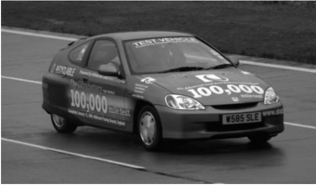
Figure 13. 100 k mile (160 k km) achievement in the UltraBattery demonstration by a Honda Insight HEV.
