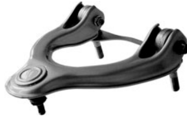
Single-shell sheet-metal design with press-in fit ball joint (Rover 400/Honda Theta)
