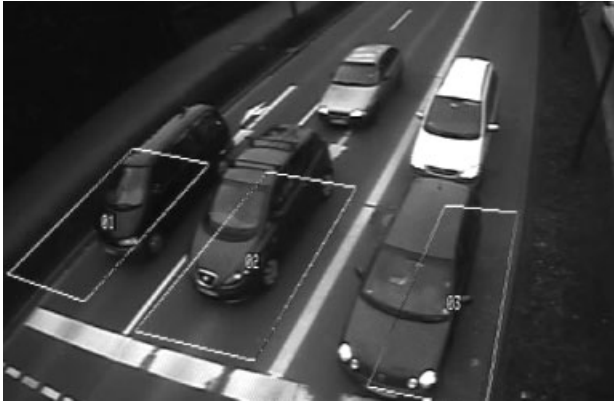
Figure 8. Image of a video detector with three detection zones.
