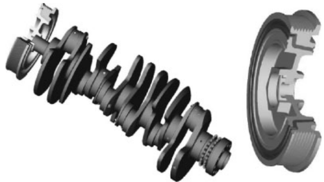
Figure 32. Torsional vibration damper in crankshaft.
