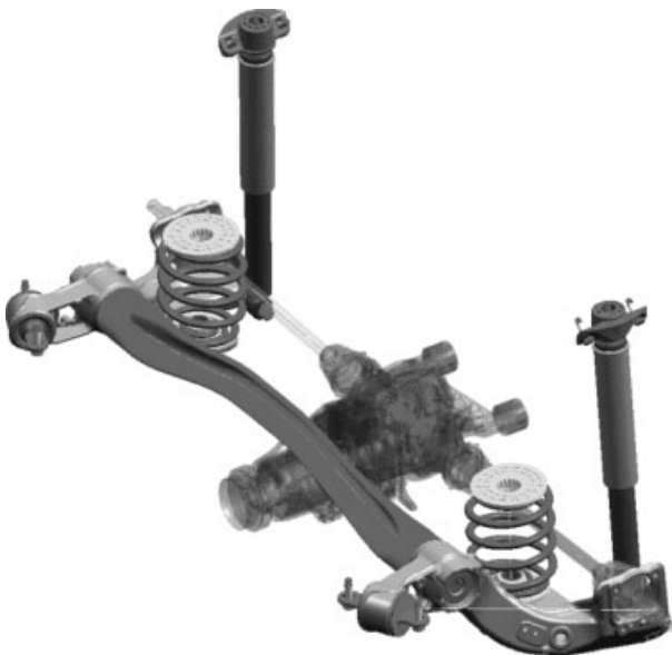
Figure 16. Four-wheel-drive-capable twist-beam axle. (Reproduced by permission of Adam Opel AG, Germany.)
