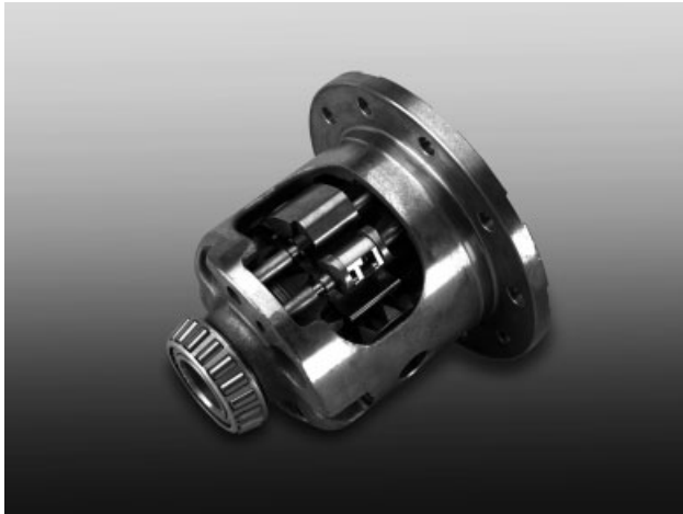
Figure 9. The governor lock limited slip differential. (Reproduced by permission of Joe Palazzolo.)
