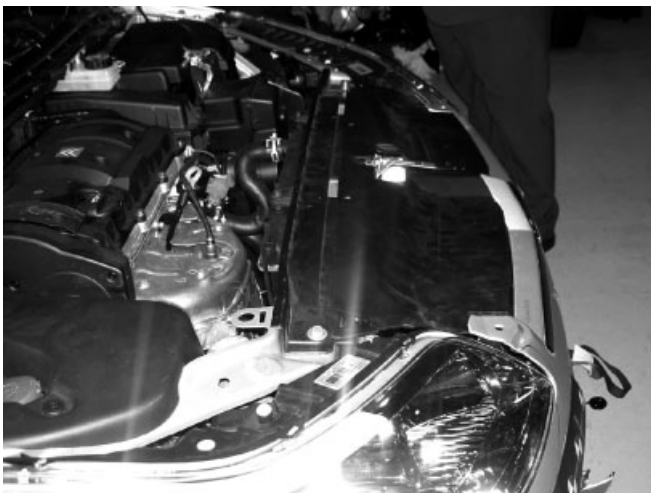
Figure 33. Plastic frontal elements, increase distance to stiff elements.
