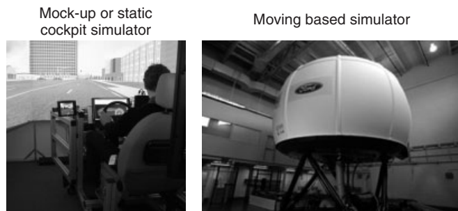
Figure 8. Examples of simulators used for validation of automotive HMIs. (Reproduced with permission from Ford. © Ford.)
