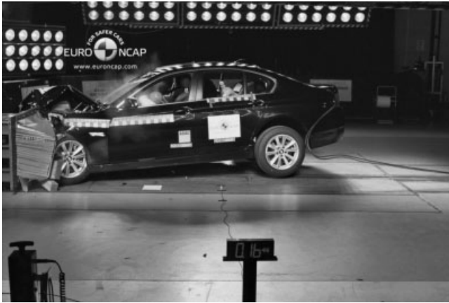
Figure 4. Example of 64 km/h ODB test. (From http://www.euroncap.com/results/bmw/5_series/2010/401.aspx . Reproduced by permission of Euro NCAP.)
