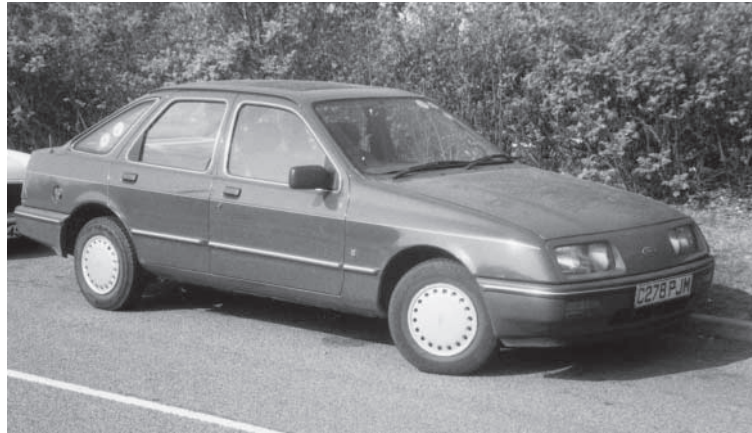
Figure 1.11 The Ford Sierra that introduced truly aerodynamic styling in the 1980s. The public took some time to adjust to the styling, which nevertheless set the trend for the next two decades.
