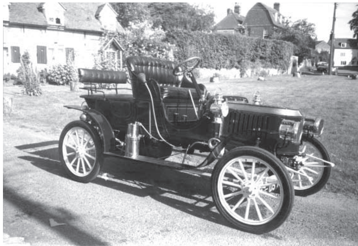
Figure 1.1 A Stanley steam car of 1905. This elegant vehicle is far removed from the lumbering smoky traction engines that nowadays chug their way to nostalgic steam rallies. Steam cars were much quieter and smoother-running than their petrol engined contemporaries, but took some time to fire up. They also needed frequent intakes of water.
