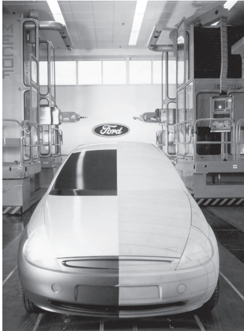
Figure 4.3 Electronic scan/mill system
