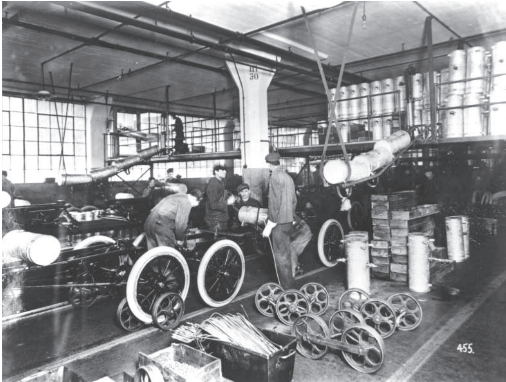
Figure 1.4 Early mass production at Ford's Highland Park plant in Detroit in 1914: the fuel tank assembly station. The chassis is moved on a track, and the cylindrical fuel tanks are supplied to the assemblers from an overhead store. The production techniques may look somewhat rudimentary by modern standards, but were innovative in their time. (Photo courtesy of Ford Motor Company Ltd.)
