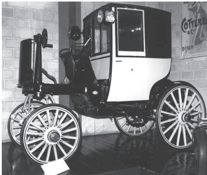
Figure 1.7 Early motor vehicles were often simply adaptations of horsedrawn vehicles, as may be seen in this 1897 Bersley electrically propelled cab. Only the absence of shafts for the horses betrays the fact that it is a motor vehicle. Note how the driver is totally exposed to the elements. (From the collection of the National Motor Museum, Beaulieu).
