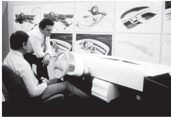
Figure 4.11 Example of Foamcore or card model
