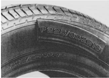
Fig. 2.17 ZR tyres manufactured specially for the American market and marked with a 'P' do not meet the European standard and are therefore not authorized here (photograph: Dunlop factory).
