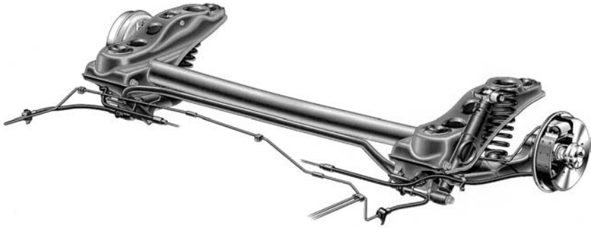
Fig. 1.13 Trailing-arm rear suspension of the Mercedes-Benz A class (1997). In order to minimize the amount of room required, the coil spring and monotube gas-pressure shock absorber are directly supported by the chassis subframe. The connecting tube is stress optimized oval shaped in order to withstand the high bending moments from longitudinal and lateral wheel forces which occur in the course of driving. The torsion-bar stabilizer proceeds directly from the shock-absorber attachment for reasons of weight and ease of assembly. When establishing the spring/shock-absorber properties, the line along which the forces act and which is altered by the lift of the wheel is to be taken into consideration, as a disadvantageous load-path can occur with jounce. The two front subframes are hydraulically damped in order to achieve a good level of comfort (hydromounts). The chassis subframe can make minor elastokinematic control movements. When designing subframe mounts, it is necessary to ensure that they retain their defined properties with regard to strength and geometry even with unfavourable conditions of use (e.g. low temperatures) and for a sufficiently long period of time, because variations in the configuration have a direct effect on vehicle performance. The longitudinal arms which run on tapered-roller bearings and which are subject to both flexural as well as torsional stress are designed in the form of a parallelogram linkage. In this way, the inherent disadvantage of a trailing arm axle – unwanted toe-in as a result of the deformation of the link when subject to a lateral force – is reduced by 75%, according to works specifications.
