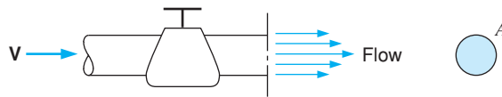
FIGURE 4.3 The flow across a control volume surface with a flow cross-sectional area of A . Average velocity is shown to the left of the valve, and a distributed flow across the area is shown to the right of the valve.
