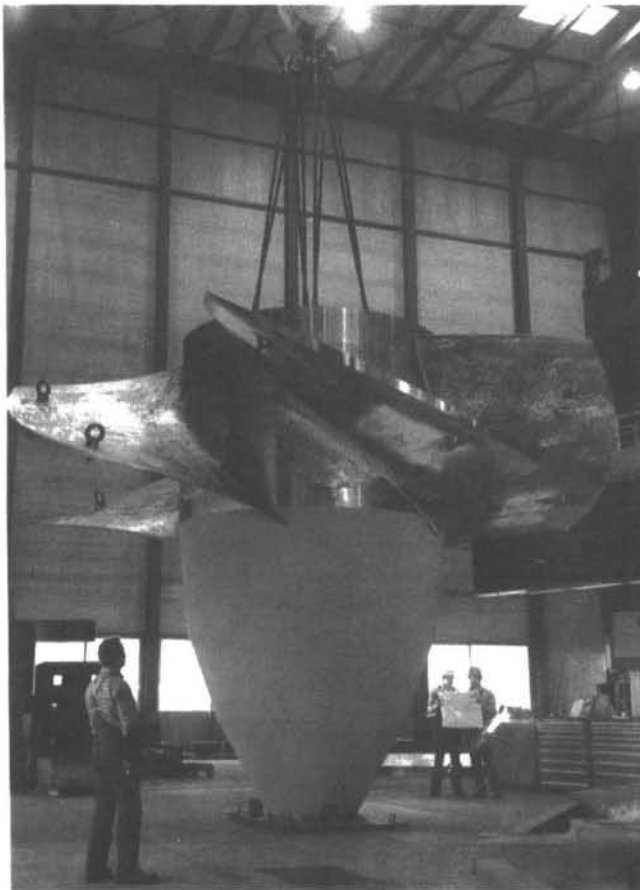
Photograph of fixed blade runner in workshop assembly. Courtesy: Sulzer Escher Wyss, Zurich, Switzerland.
