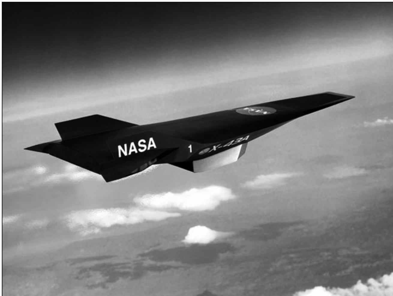
Fig. 9.30 The proposed X-43A hypersonic airplane. The scramjet engine is underneath. Air passing through the engine remains fully supersonic. (Courtesy of the X-43A Development Team, DFRC, NASA.)
