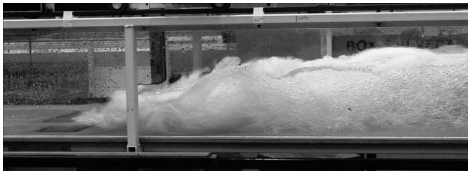
Fig. 10.11 Hydraulic jump in a laboratory open channel. Note the extreme, dissipative turbulence in the downstream flow. Data are given in Prob. P10.94. (Courtesy of Prof. Hubert Chanson, University of Queensland.)
