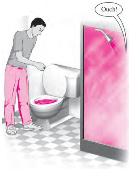
FIGURE 8-50 Flow rate of cold water through a shower may be affected significantly by the flushing of a nearby toilet.
