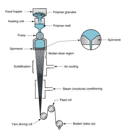
FIGURE 13.18 Melt spinning of continuous filaments.
