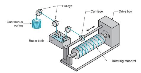
**FIGURE 15.8** Filament winding.
