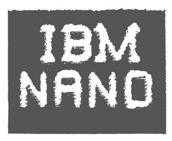
FIGURE 37.3 An atomic force microscope image of silicon dioxide letters on a silicon substrate. The oxide lines of the letters are about 20 nm wide. (Image courtesy of IBM Corporation.)
