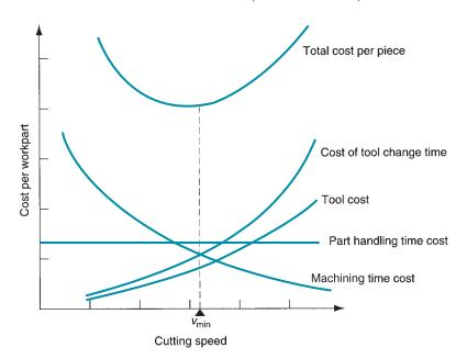
FIGURE 24.4 Cost components in a machining operation plotted as a function of cutting speed. Total cost per piece is minimized at a certain value of cutting speed. This is the speed for minimum cost per piece.
