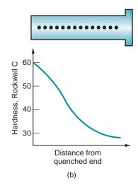
FIGURE 27.4 The Jominy end-quench test: (a) setup of the test, showing end quench of the test specimen; and (b) typical pattern of hardness readings as a function of distance from quenched end.
