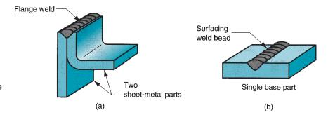
FIGURE 29.7 (a) Flange weld; and (b) surfacing weld.
