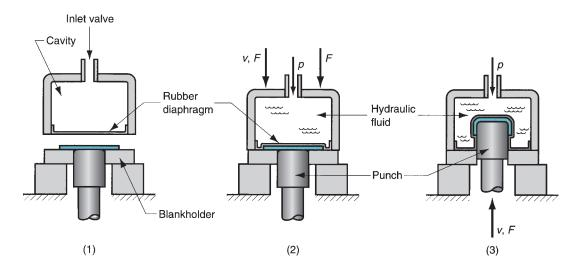
**FIGURE 20.29** Hydroform process: (1) start-up, no fluid in cavity; (2) press closed, cavity pressurized with hydraulic fluid; (3) punch pressed into work to form part. Symbols: v = velocity, F = applied force, p = hydraulic pressure.
