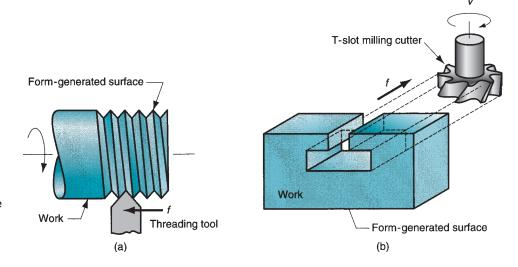
FIGURE 22.4 Combination of forming and generating to create shape: (a) thread cutting on a lathe, and (b) slot milling.
