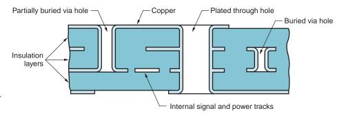
FIGURE 35.8 Typical cross section of a multilayer printed circuit board.
