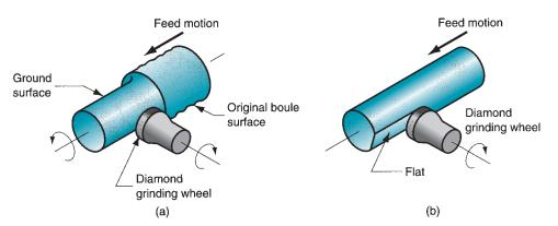
FIGURE 34.6 Grinding operations used in shaping the silicon ingot: (a) a form of cylindrical grinding provides diameter and roundness control, and (b) a flat ground on the cylinder.
