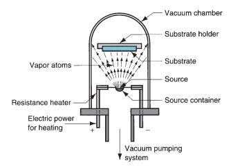
FIGURE 28.6 Setup for vacuum evaporation physical vapor deposition.
