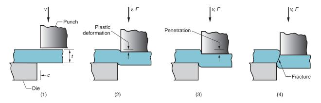
**FIGURE 20.1** Shearing of sheet metal between two cutting edges: (1) just before the punch contacts work; (2) punch begins to push into work, causing plastic deformation; (3) punch compresses and penetrates into work causing a smooth cut surface; and (4) fracture is initiated at the opposing cutting edges that separate the sheet. Symbols v and F indicate motion and applied force, respectively, t = stock thickness, c = clearance.
