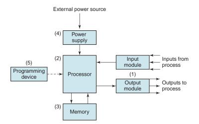
FIGURE 38.6 Major components of a programmable logic controller.
