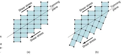
FIGURE 2.13 Twinning involves the formation of an atomic mirror image (i.e., a "twin") on the opposite side of the twinning plane: (a) before, and (b) after twinning.
