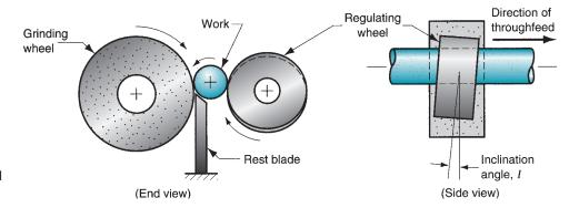
FIGURE 25.11 External centerless grinding.
