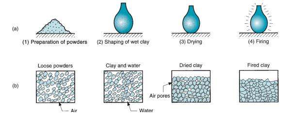
**FIGURE 17.1** Usual steps in traditional ceramics processing: (1) preparation of raw materials, (2) shaping, (3) drying, and (4) firing. Part (a) shows the workpart during the sequence, whereas (b) shows the condition of the powders.
