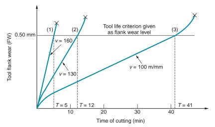
FIGURE 23.4 Effect of cutting speed on tool flank wear (FW) for three cutting speeds.
