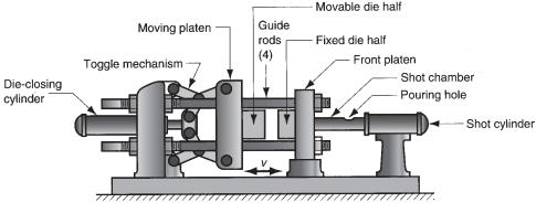
FIGURE 11.12 General configuration of a (cold-chamber) die casting machine.
