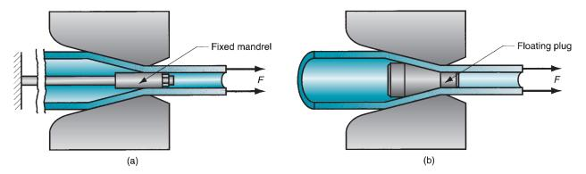
FIGURE 19.45 Tube drawing with mandrels: (a) fixed mandrel, (b) floating plug.
