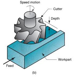
FIGURE 22.17 Two basic types of milling operations: (a) peripheral or plain milling and (b) face milling.
