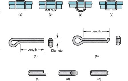
FIGURE 32.16 Cotter pins: (a) offset head, standard point; (b) symmetric head, hammerlock point; (c) square point; (d) mitered point; and (e) chisel point.
