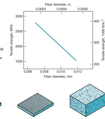
FIGURE 9.2 Relationship between tensile strength and diameter for a carbon fiber. (Source: [1]). Other filament materials show similar relationships.
