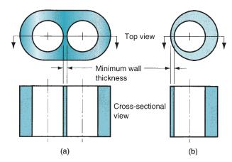
recommended wall thickness (a) between holes or (b) between a hole and an outside wall should be 1.5 mm (0.060 in).
