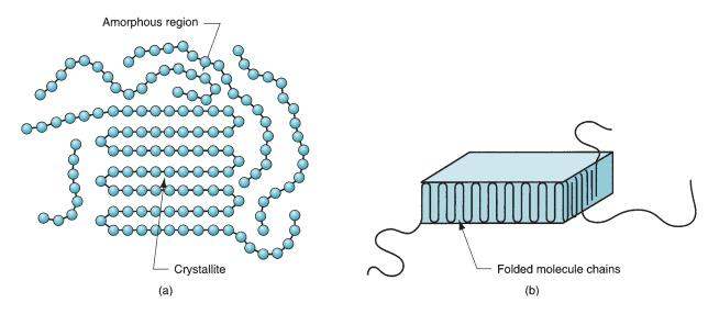
**FIGURE 8.9** Crystallized regions in a polymer: (a) long molecules forming crystals randomly mixed in with the amorphous material; and (b) folded chain lamella, the typical form of a crystallized region.
