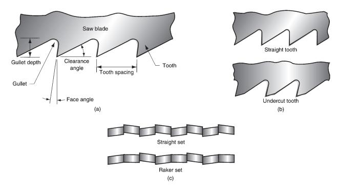
**FIGURE 23.19** Features of saw blades: (a) nomenclature for saw blade geometries, (b) two common tooth forms, and (c) two types of tooth set.
