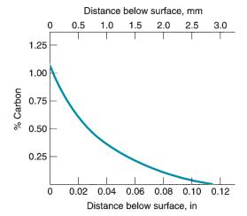
FIGURE 28.3 Characteristic profile of diffused element as a function of distance below surface in diffusion. The plot given here is for carbon diffused into iron. (Source: [6].)
