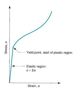
**FIGURE 3.8** Typical engineering stress–strain curve for a compression test.
