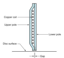
FIGURE 36.5 Thin-film magnetic read-write head (simplified).
