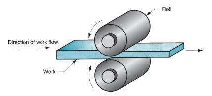
FIGURE 19.1 The rolling process (specifically, flat rolling).
