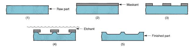
**FIGURE 26.16** Sequence of processing steps in chemical milling: (1) clean raw part, (2) apply maskant, (3) scribe, cut, and peel the maskant from areas to be etched, (4) etch, and (5) remove maskant and clean to yield finished part.
