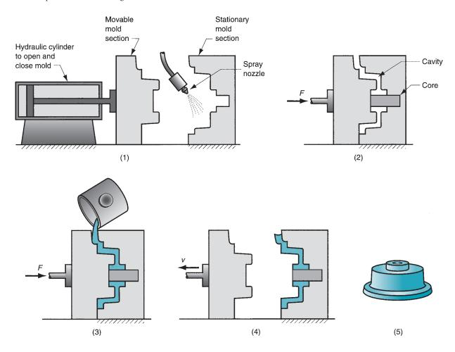
**FIGURE 11.10** Steps in permanent-mold casting: (1) mold is preheated and coated; (2) cores (if used) are inserted, and mold is closed; (3) molten metal is poured into the mold; and (4) mold is opened. Finished part is shown in (5).
