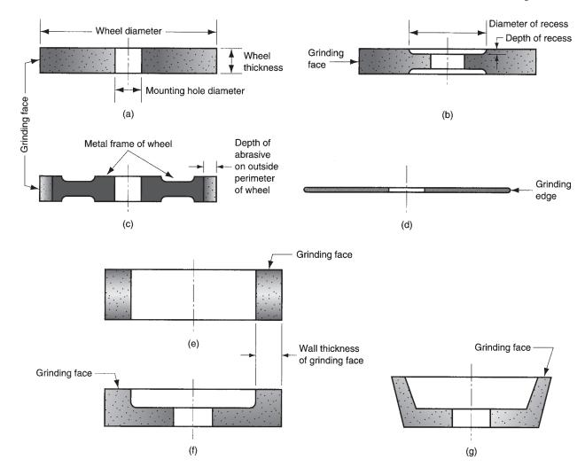
**FIGURE 25.2** Some of the standard grinding wheel shapes: (a) straight, (b) recessed two sides, (c) metal wheel frame with abrasive bonded to outside circumference, (d) abrasive cutoff wheel, (e) cylinder wheel, (f) straight cup wheel, and (g) flaring cup wheel.
