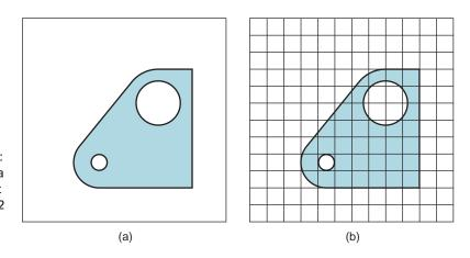
FIGURE 42.9 Image acquisition and digitizing: (a) the scene consists of a dark-colored part against a light background; (b) a 12 × 12 matrix of pixels imposed on the scene.
