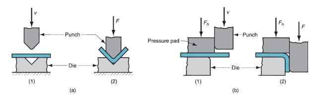
**FIGURE 20.12** Two common bending methods: (a) V-bending and (b) edge bending; (1) before and (2) after bending. Symbols: v = motion, F = applied bending force,  $F_h = \text{blank}$ .
