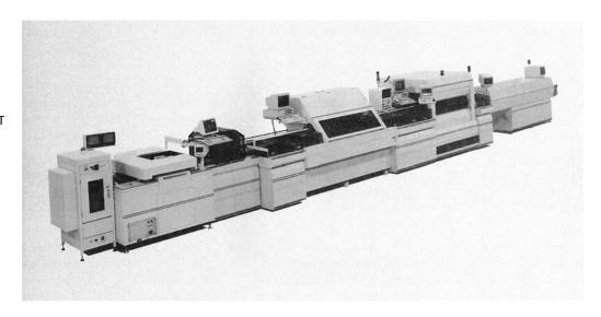
FIGURE 35.13 SMT production line. Stations include board launching, screen printing of solder paste, several component placement operations, and solder reflow oven. (Photo courtesy of Universal Instruments Corp.)
