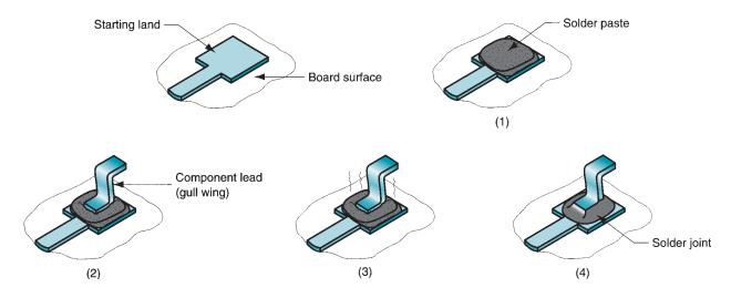
**FIGURE 35.12** Solder paste and reflow method: (1) apply solder paste to desired land areas, (2) place components onto board, (3) bake paste, and (4) solder reflow.
