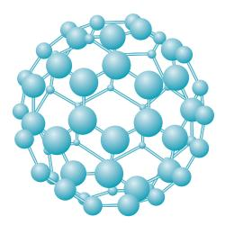
$C_{60}$ , the 60 atoms are arranged symmetrically into 12 pentagonal faces and 20 hexagonal faces to form a ball. These molecular balls can be bonded together by van der Waals forces (Section 2.2) to form crystals whose lattice structure is face-centered cubic (Figure 2.8(b), Section 2.3.1). The separation between any molecule and its closest neighbor in the  $C_{60}$  lattice structure is 1 nm.
