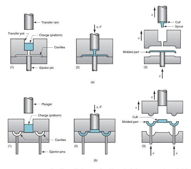
**FIGURE 13.29** (a) Pottransfer molding, and (b) plunger transfer molding. Cycle in both processes is: (1) charge is loaded into pot, (2) softened polymer is pressed into mold cavity and cured, and (3) part is ejected.
