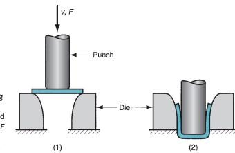
FIGURE 20.23 Drawing without a blankholder: (1) start of process, (2) end of stroke. Symbols *v* and *F* indicate motion and applied force, respectively.
