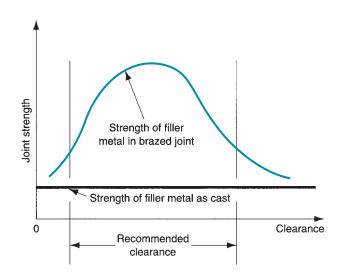
**FIGURE 31.3** Joint strength as a function of joint clearance.
