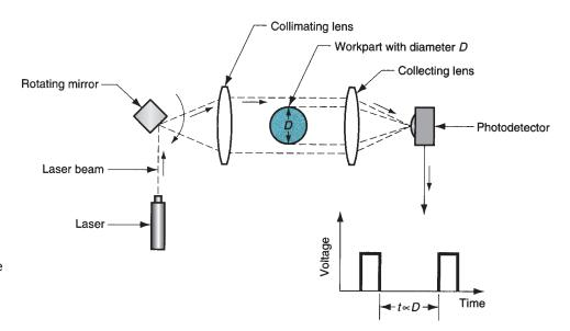
FIGURE 42.6 Scanning laser system for measuring diameter of cylindrical workpart; time of interruption of light beam is proportional to diameter *D*.
