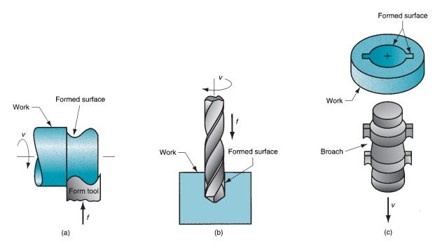
FIGURE 22.3 Forming to create shape in machining: (a) form turning, (b) drilling, and (c) broaching.
