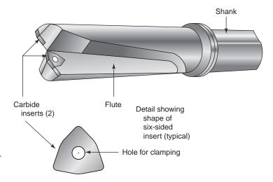
FIGURE 23.13 Straightflute drill that uses indexable inserts.
