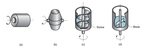
Several blending and mixing devices: (a) rotating drum, (b) rotating double-cone, **FIGURE 16.8** (c) screw mixer, and (d) blade mixer.
