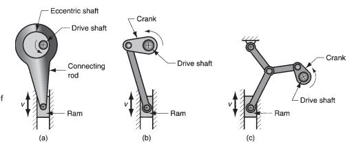
FIGURE 20.38 Types of drives for sheet-metal presses: (a) eccentric, (b) crankshaft, and (c) knuckle joint.
