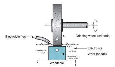
FIGURE 26.6 Electrochemical grinding (ECG).
