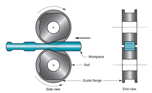
FIGURE 19.26 Roll forging.
