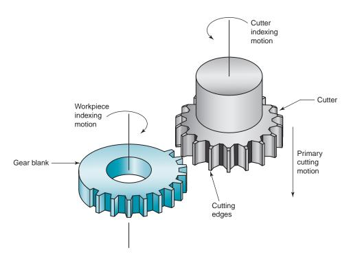
**FIGURE 22.41** Gear shaping.
