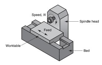
**FIGURE 22.25** Simplex bedtype milling machine horizontal spindle.
