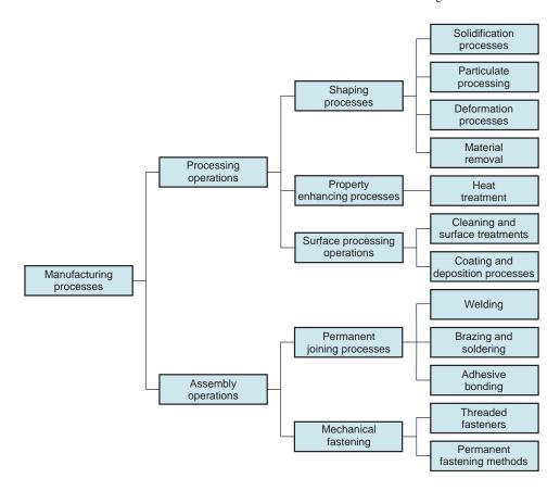
FIGURE 1.4 Classification of manufacturing processes.
