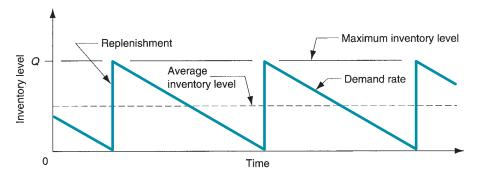
FIGURE 41.2 Model of inventory level over time in the typical make-to-stock situation.
