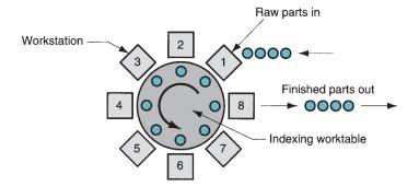
FIGURE 39.5 Configuration of a dial-indexing machine.
