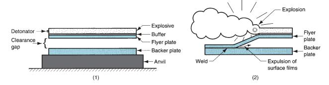
**FIGURE 30.27** Explosive welding (EXW): (1) setup in the parallel configuration, and (2) during detonation of the explosive charge.
