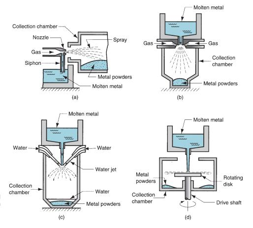
atomization methods for producing metallic powders: (a) and (b) two gas atomization methods; (c) water atomization; and (d) centrifugal atomization by the rotating disk method.
