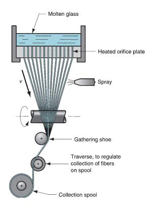
**FIGURE 12.9** Drawing of continuous glass fibers.
