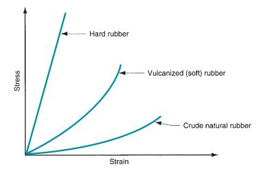
FIGURE 8.13 Increase in stiffness as a function of strain for three grades of rubber: natural rubber, vulcanized rubber, and hard rubber.
