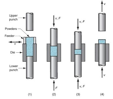
FIGURE 16.9 Pressing, the conventional method of compacting metal powders in PM: (1) filling the die cavity with powder, done by automatic feed in production, (2) initial, and (3) final positions of upper and lower punches during compaction, and (4) ejection of part.
