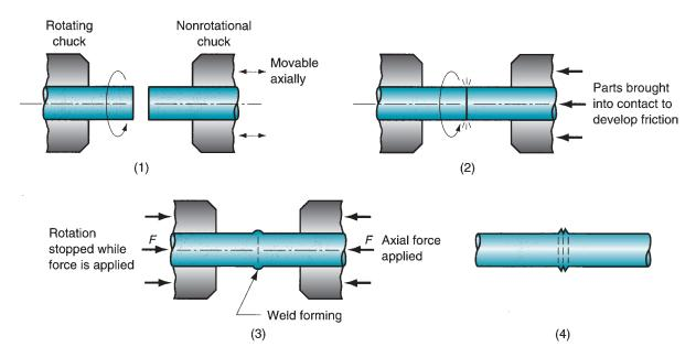
**FIGURE 30.28** Friction welding (FRW): (1) rotating part, no contact; (2) parts brought into contact to generate friction heat; (3) rotation stopped and axial pressure applied; and (4) weld created.
