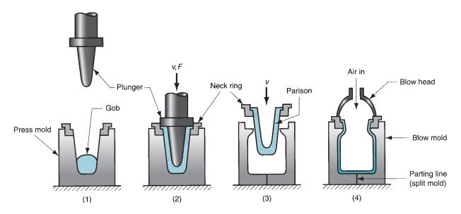
**FIGURE 12.4** Press-and-blow forming sequence: (1) molten gob is fed into mold cavity; (2) pressing to form a *parison*; (3) the partially formed parison, held in a neck ring, is transferred to the blow mold; and (4) blown into final shape. Symbols v and F indicate motion (v = velocity) and applied force, respectively.
