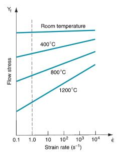
**FIGURE 18.6** Effect of temperature on flow stress for a typical metal. The constant C in Eq. (18.4), indicated by the intersection of each plot with the vertical dashed line at strain rate = 1.0, decreases, and m (slope of each plot) increases with increasing temperature.
