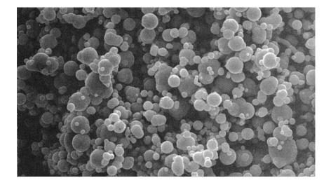
FIGURE 16.6 Iron powders produced by decomposition of iron pentacarbonyl; particle sizes range from about 0.25 to 3.0  $\mu$ m (10–125  $\mu$ -in). (Photo courtesy of GAF Chemicals Corporation, Advanced Materials Division.)
