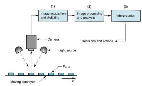
**FIGURE 42.8** Operation of a machine vision system.
