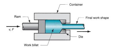
FIGURE 19.30 Direct extrusion.
