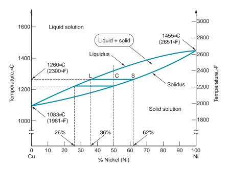
**FIGURE 6.2** Phase diagram for the coppernickel alloy system.
