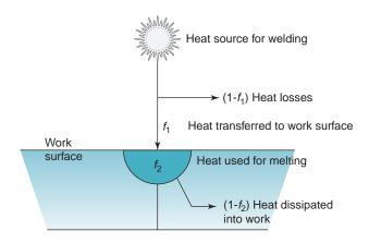
FIGURE 29.8 Heat transfer mechanisms in fusion welding.
