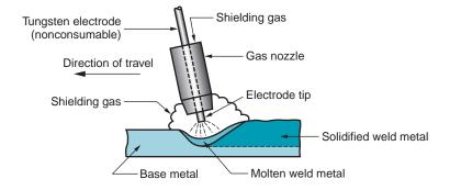
**FIGURE 30.9** Gas tungsten arc welding (GTAW).
