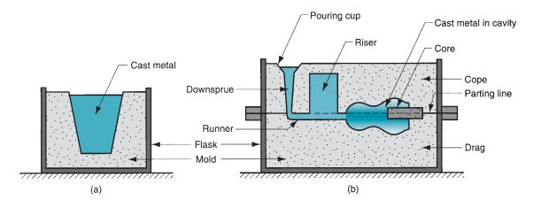
**FIGURE 10.2** Two forms of mold: (a) open mold, simply a container in the shape of the desired part; and (b) closed mold, in which the mold geometry is more complex and requires a gating system (passageway) leading into the cavity.
