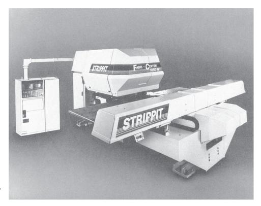
FIGURE 20.36 Computer numerical control turret press. (Photo courtesy of Strippet, Inc., Akron, New York.)
