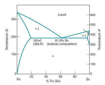
**FIGURE 6.3** Phase diagram for the tin–lead alloy system.
