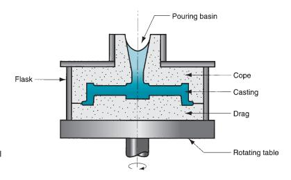
**FIGURE 11.16** Semicentrifugal casting.
