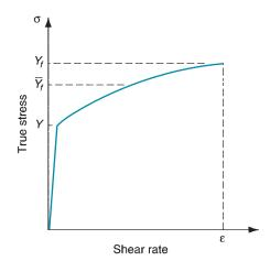
**FIGURE 18.4** Stress–strain curve indicating location of average flow stress  $\overline{Y}_f$  in relation to yield strength Y and final flow stress  $Y_f$ .
