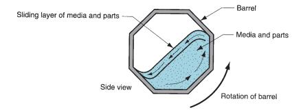
FIGURE 28.1 Diagram of tumbling (barrel finishing) operation showing "landslide" action of parts and abrasive media to finish the parts.
