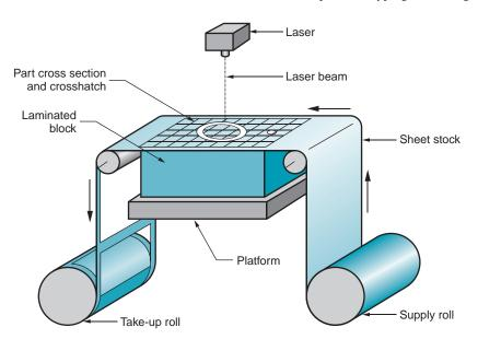
FIGURE 33.5 Laminated-object manufacturing.
