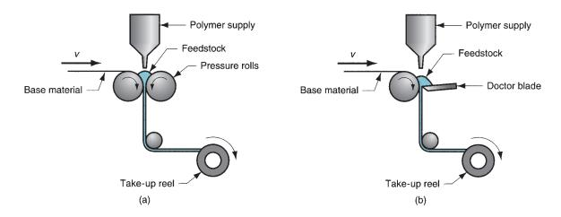
FIGURE 13.19 Planar coating processes: (a) roll method, and (b) doctor-blade method.
