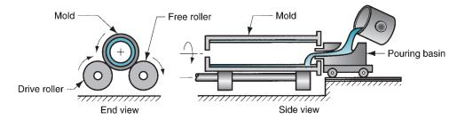
FIGURE 11.15 Setup for true centrifugal casting.
