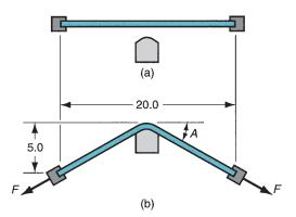
**FIGURE P20.31** Stretch forming operation: (a) before, and (b) after (dimensions in inches).
