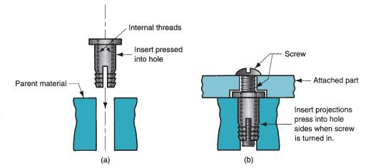
FIGURE 32.6 Screw thread inserts: (a) before insertion, and (b) after insertion into hole and screw is turned into the insert.
