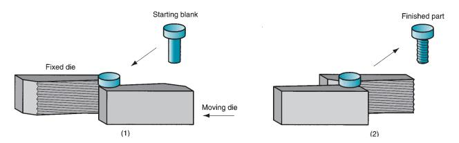
FIGURE 19.6 Thread rolling with flat dies: (1) start of cycle and (2) end of cycle.
