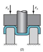
**FIGURE 20.22** Reverse drawing: (1) start and (2) completion. Symbols: v = punch velocity, F = applied punch force,  $F_h = \text{blankholder force}$ .
