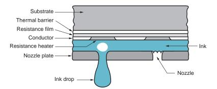
**FIGURE 36.4** Diagram of an ink-jet printing head.
