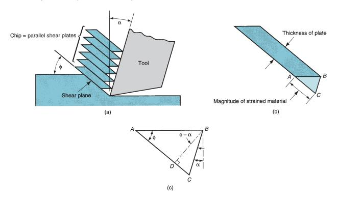
**FIGURE 21.7** Shear strain during chip formation: (a) chip formation depicted as a series of parallel plates sliding relative to each other; (b) one of the plates isolated to illustrate the definition of shear strain based on this parallel plate model; and (c) shear strain triangle used to derive Eq. (21.4).
