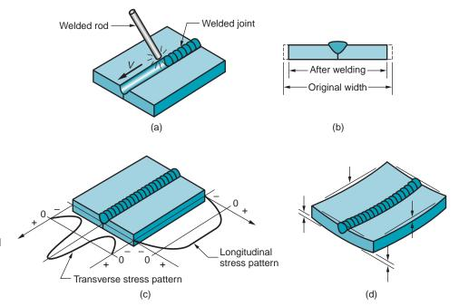
FIGURE 30.31 (a) Butt welding two plates; (b) shrinkage across the width of the welded assembly; (c) transverse and longitudinal residual stress pattern; and (d) likely warping in the welded assembly.
