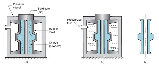
**FIGURE 16.14** Cold isostatic pressing: (1) powders are placed in the flexible mold; (2) hydrostatic pressure is applied against the mold to compact the powders; and (3) pressure is reduced and the part is removed.
