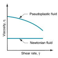
**FIGURE 13.1** Viscosity relationships for Newtonian fluid and typical polymer melt.
