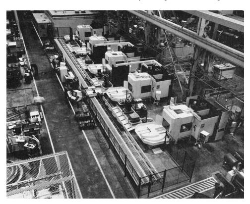
FIGURE 39.13 A fivestation flexible manufacturing system. (Photo courtesy of Cincinnati Milacron, Batavia, Ohio.)
