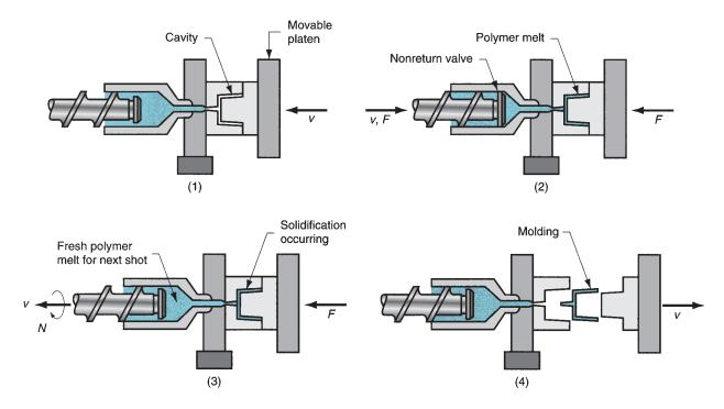
**FIGURE 13.22** Typical molding cycle: (1) mold is closed, (2) melt is injected into cavity, (3) screw is retracted, and (4) mold opens, and part is ejected.
