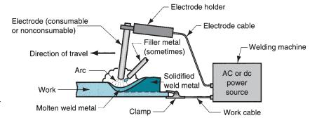
FIGURE 30.1 The basic configuration and electrical circuit of an arcwelding process.
