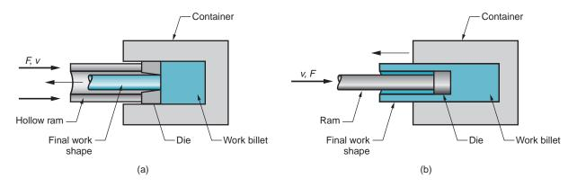
FIGURE 19.32 Indirect extrusion to produce (a) a solid cross section and (b) a hollow cross section.
