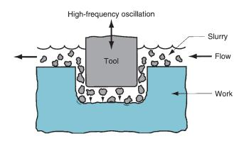
FIGURE 26.1 Ultrasonic machining.
