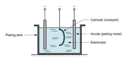
**FIGURE 28.5** Setup for electroplating.
