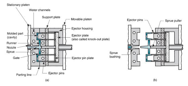
**FIGURE 13.23** Details of a two-plate mold for thermoplastic injection molding: (a) closed and (b) open. Mold has two cavities to produce two cup-shaped parts (cross section shown) with each injection shot.
