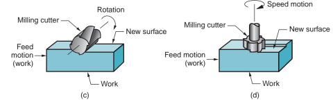
FIGURE 21.3 The three most common types of machining processes:
