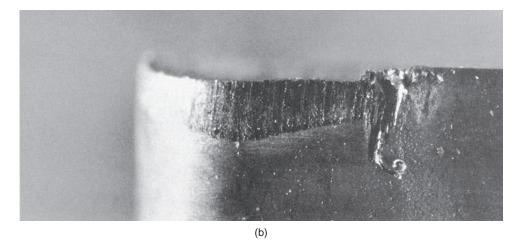
FIGURE 23.2 (a) Crater wear and (b) flank wear on a cemented carbide tool, as seen through a toolmaker's microscope. (Courtesy of Manufacturing Technology Laboratory, Lehigh University, photos by J. C. Keefe.)
