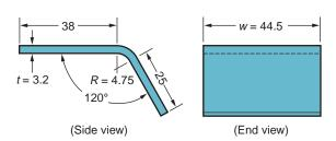
**FIGURE 20.15** Sheet-metal part of Example 20.220.2 (dimensions in mm).
