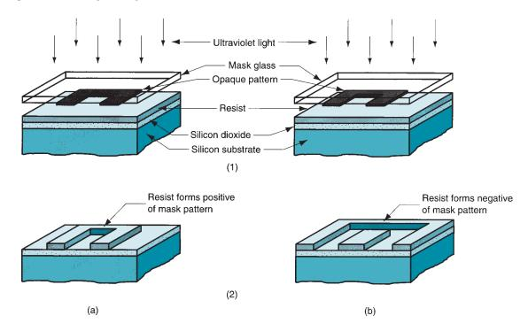
Application of (a) positive resist and (b) negative resist in photolithography; for both types, the sequence shows: (1) exposure through the mask and (2) remaining resist after developing.
