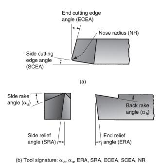
FIGURE 23.7 (a) Seven elements of single-point tool geometry, and (b) the tool signature convention that defines the seven elements.
