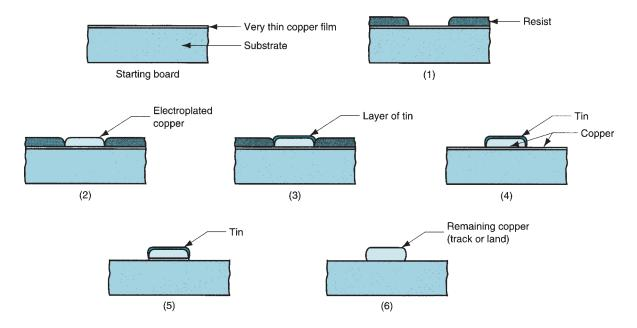
**FIGURE 35.7** The semiadditive method of circuitization in PCB fabrication: (1) Apply resist to areas that will not be plated; (2) electroplate copper, using the thin copper film for conduction; (3) apply tin on top of plated copper; (4) strip resist; (5) etch remaining thin film of copper on the surface, while the tin serves as a resist for the electroplated copper; and (6) strip tin from copper.
