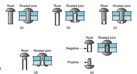
FIGURE 32.10 Five basic rivet types, also shown in assembled configuration: (a) solid, (b) tubular, (c) semitubular, (d) bifurcated, and (e) compression.
