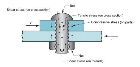
FIGURE 32.9 Typical stresses acting on a bolted joint.
