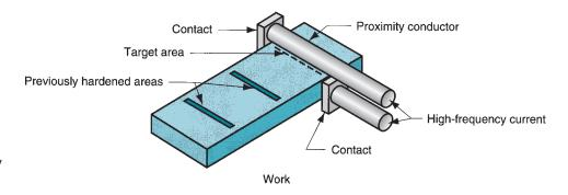
**FIGURE 27.8** Typical setup for high-frequency resistance heating.
