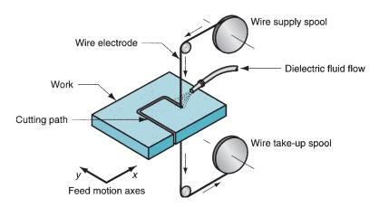
FIGURE 26.9 Electric discharge wire cutting (EDWC), also called wire EDM.
