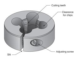
FIGURE 22.36 Threading die.
