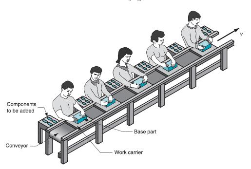
FIGURE 39.3 A portion of a manual assembly line. Each worker performs a task at his/her workstation. A conveyor moves parts on work carriers from one station to the next.
