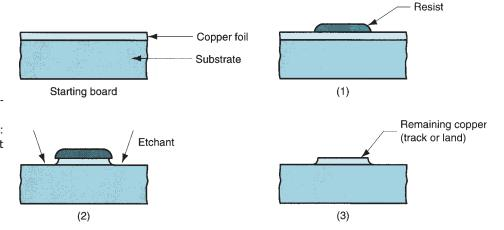
FIGURE 35.5 The subtractive method of circuitization in PCB fabrication: (1) apply resist to areas not to be etched, using photolithography to expose the areas that are to be etched, (2) etch, and (3) strip resist.
