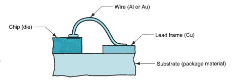
FIGURE 34.21 Typical wire connection between chip contact pad and lead.
