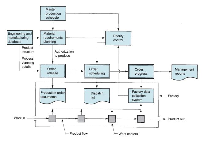
**FIGURE 41.6** Three modules in a shop floor control system, and interconnections with other production planning and control functions.
