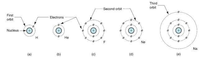
**FIGURE 2.2** Simple model of atomic structure for several elements: (a) hydrogen, (b) helium, (c) fluorine, (d) neon, and (e) sodium.
