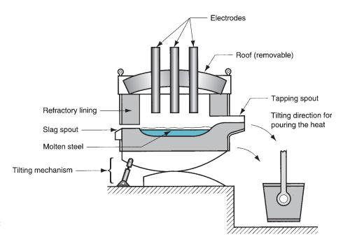
**FIGURE 6.9** Electric arc furnace for steelmaking.
