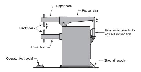
FIGURE 30.14 Rockerarm spot-welding machine.
