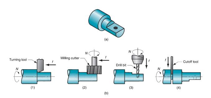
**FIGURE 22.28** Operation of a mill-turn center: (a) example part with turned, milled, and drilled surfaces; and (b) sequence of operations on a mill-turn center: (1) turn second diameter, (2) mill flat with part in programmed angular position, (3) drill hole with part in same programmed position, and (4) cutoff.
