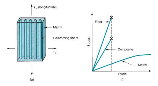
**FIGURE 9.5** (a) Model of a fiber-reinforced composite material showing direction in which elastic modulus is being estimated by the rule of mixtures. (b) Stress–strain relationships for the composite material and its constituents. The fiber is stiff but brittle, while the matrix (commonly a polymer) is soft but ductile. The composite's modulus is a weighted average of its components' moduli. But when the reinforcing fibers fail, the composite does likewise.
