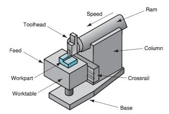
FIGURE 22.30 Components of a shaper.
