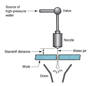
FIGURE 26.2 Water jet cutting.
