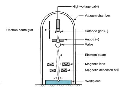
FIGURE 26.12 Electron beam machining (EBM).
