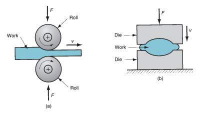
FIGURE 18.2 Basic bulk deformation processes: (a) rolling, (b) forging, (c) extrusion, and (d) drawing. Relative motion in the operations is indicated by v; forces are indicated by F.
