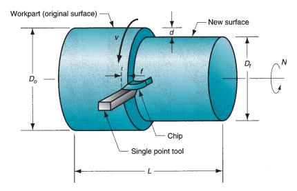
FIGURE 22.5 Turning operation.
