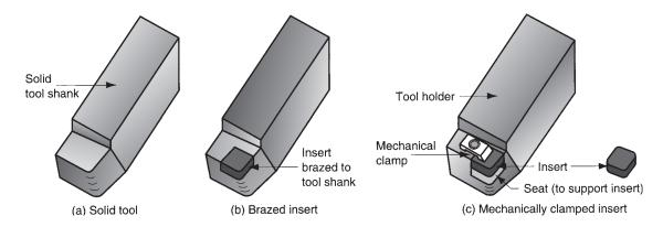
**FIGURE 23.9** Three ways of holding and presenting the cutting edge for a single-point tool: (a) solid tool, typical of HSS; (b) brazed insert, one way of holding a cemented carbide insert; and (c) mechanically clamped insert, used for cemented carbides, ceramics, and other very hard tool materials.
