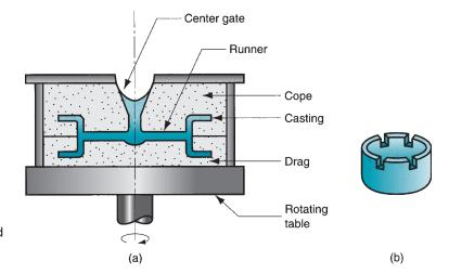
FIGURE 11.17 (a) Centrifuge casting—centrifugal force causes metal to flow to the mold cavities away from the axis of rotation; and (b) the casting.
