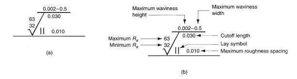
**FIGURE 5.16** Surface texture symbols in engineering drawings: (a) the symbol, and (b) symbol with identification labels. Values of  $R_a$  are given in microinches; units for other measures are given in inches. Designers do not always specify all of the parameters on engineering drawings.
