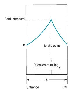
**FIGURE 19.4** Typical variation in pressure along the contact length in flat rolling. The peak pressure is located at the neutral point. The area beneath the curve, representing the integration in Eq. (19.9), is the roll force *F*.
