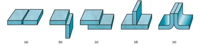
FIGURE 29.2 Five basic types of joints: (a) butt, (b) corner, (c) lap, (d) tee, and (e) edge.
