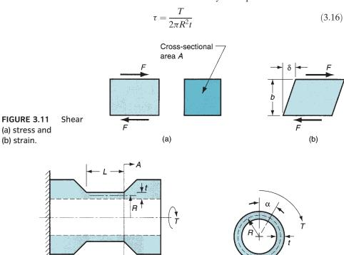
FIGURE 3.12 Torsion test setup.
