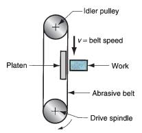
FIGURE 25.15 Abrasive belt grinding.
