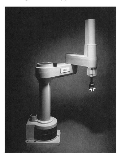
FIGURE 38.13 The manipulator of a modern industrial robot. (Photo courtesy of Adept Technology, Inc., Pleasanton, California.)
