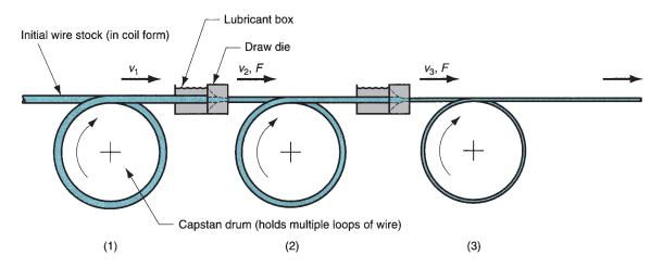
FIGURE 19.42 Continuous drawing of wire.
