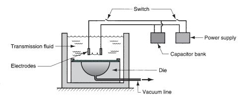
FIGURE 20.46 Electrohydraulic forming setup.
