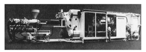
FIGURE 13.20 A large (3000-ton capacity) injection molding machine. (Courtesy of Cincinnati Milacron.)
