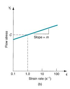
FIGURE 18.5 (a) Effect of strain rate on flow stress at an elevated work temperature. (b) Same relationship plotted on log-log coordinates.
