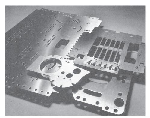
sheet-metal parts produced on a turret press, showing variety of possible hole shapes. (Photo courtesy of Strippet, Inc., Akron, New York.)
