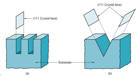
structures that can be formed in single-crystal silicon substrate by bulk micromachining: (a) (110) silicon and (b) (100) silicon.
