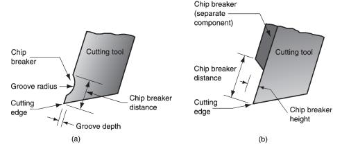
FIGURE 23.8 Two methods of chip breaking in single-point tools:
