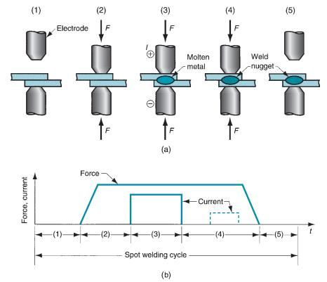
FIGURE 30.13 (a) Steps in a spot-welding cycle, and (b) plot of squeezing force and current during cycle. The sequence is: (1) parts inserted between open electrodes, (2) electrodes close and force is applied, (3) weld timecurrent is switched on, (4) current is turned off but force is maintained or increased (a reduced current is sometimes applied near the end of this step for stress relief in the weld region), and (5) electrodes are opened, and the welded assembly is removed.
