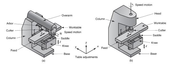
FIGURE 22.23 Two basic types of knee-and-column milling machine: (a) horizontal and (b) vertical.
