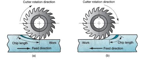
FIGURE 22.19 Two forms of peripheral milling operation with a 20-teeth cutter: (a) up milling, and (b) down milling.
