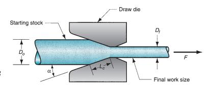
FIGURE 19.40 Drawing of bar, rod, or wire.
