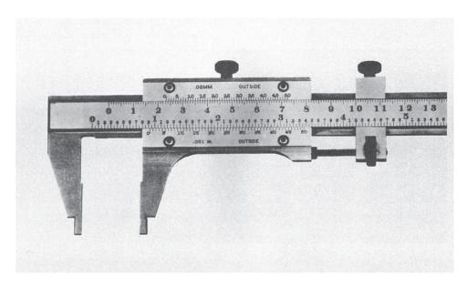
FIGURE 5.4 Vernier caliper. (Courtesy of L.S. Starrett Co.)
