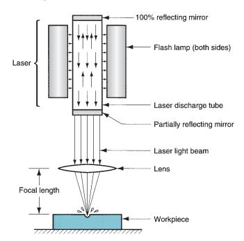
FIGURE 26.13 Laser beam machining (LBM).
