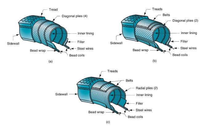
FIGURE 14.5 Three principal tire constructions: (a) diagonal ply, (b) belted bias, and (c) radial ply.
