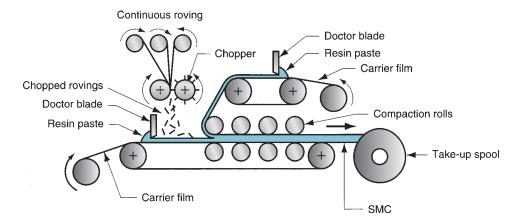
FIGURE 15.2 Process for producing sheet molding compound (SMC).
