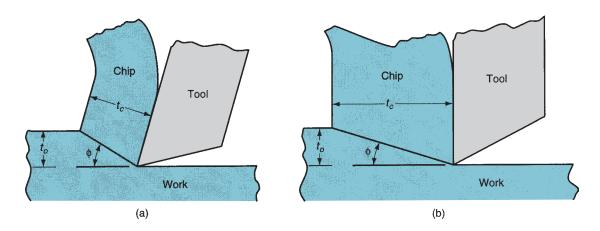
**FIGURE 21.12** Effect of shear plane angle  $\phi$ : (a) higher  $\phi$  with a resulting lower shear plane area; (b) smaller  $\phi$  with a corresponding larger shear plane area. Note that the rake angle is larger in (a), which tends to increase shear angle according to the Merchant equation.
