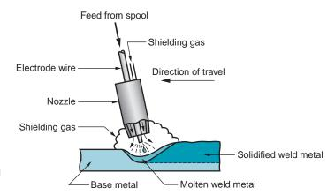
**FIGURE 30.4** Gas metal arc welding (GMAW).
