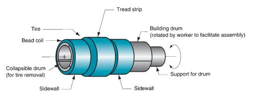
FIGURE 14.6 Tire just before removal from building drum, before molding and curing.
