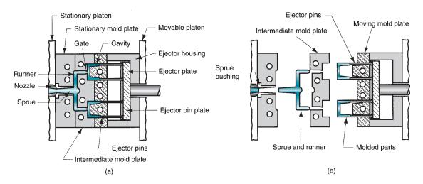
FIGURE 13.24 Three-plate mold: (a) closed, and (b) open.
