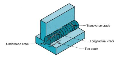
**FIGURE 30.32** Various forms of welding cracks.
