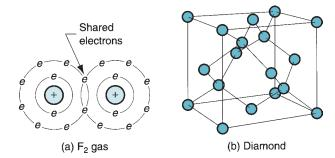
**FIGURE 2.5** Two examples of covalent bonding: (a) fluorine gas F<sub>2</sub>, and (b) diamond.
