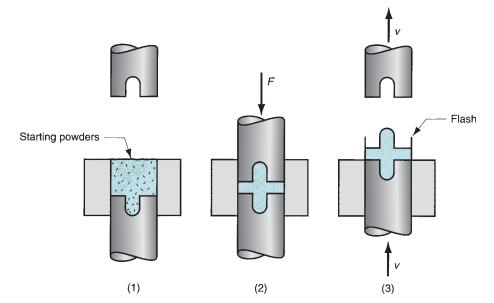
FIGURE 17.7 Semi-dry pressing: (1) depositing moist powder into die cavity, (2) pressing, and (3) opening the die sections and ejection. Symbols *v* and *F* indicate motion (*v* = velocity) and applied force, respectively.
