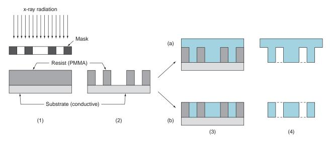
FIGURE 36.12 LIGA processing steps: (1) thick layer of resist applied and x-ray exposure through mask, (2) exposed portions of resist removed, (3) electrodeposition to fill openings in resist, (4) resist stripped to provide (a) a mold or (b) a metal part.
