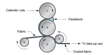
of fabric with rubber using a calendering process.
