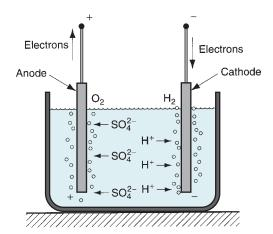
**FIGURE 4.3** Example of electrolysis: decomposition of water.
