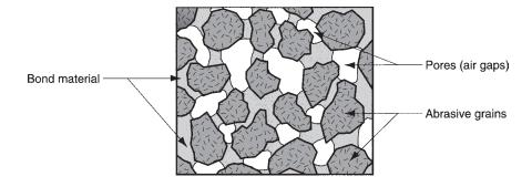
FIGURE 25.1 Typical structure of a grinding wheel.
