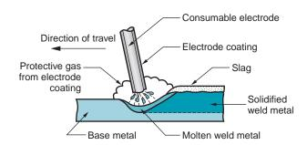
FIGURE 30.3 Shielded metal arc welding (SMAW).
