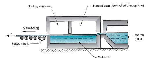
FIGURE 12.7 The float process for producing sheet glass.
