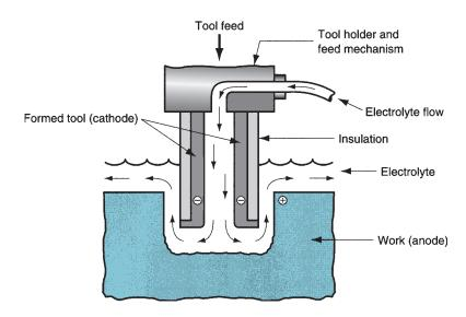
FIGURE 26.4 Electrochemical machining (ECM).
