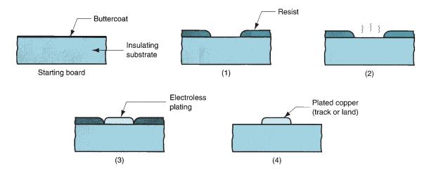
**FIGURE 35.6** The additive method of circuitization in PCB fabrication: (1) a resist film is applied to the surface using photolithography to expose the areas to be copper plated; (2) the exposed surface is chemically activated to serve as a catalyst for electroless plating; (3) copper is plated on exposed areas; and (4) resist is stripped.
