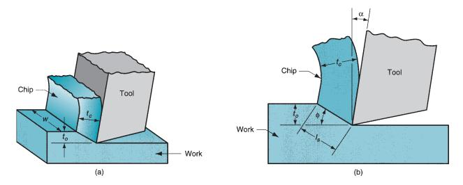
**FIGURE 21.6** Orthogonal cutting: (a) as a three-dimensional process, and (b) how it reduces to two dimensions in the side view.
