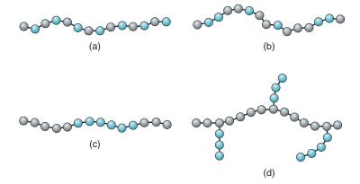
FIGURE 8.8 Various structures of copolymers: (a) alternating, (b) random, (c) block, and (d) graft.
