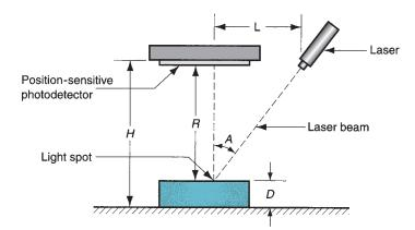
FIGURE 42.7 Laser triangulation to measure part dimension *D*.
