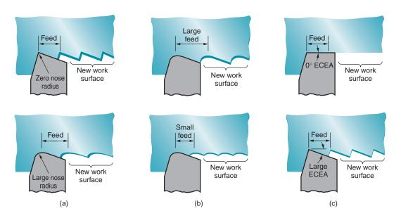
**FIGURE 24.1** Effect of geometric factors in determining the theoretical finish on a work surface for single-point tools: (a) effect of nose radius, (b) effect of feed, and (c) effect of end cutting-edge angle.
