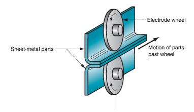
FIGURE 30.15 Resistance seam welding (RSEW).
