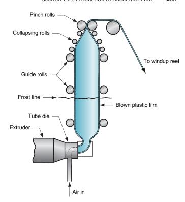
FIGURE 13.16 Blownfilm process for high production of thin tubular film.
