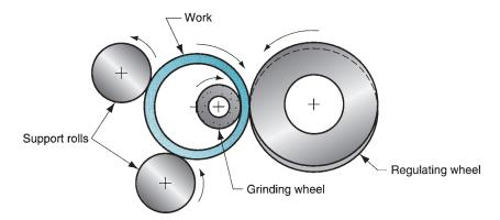
FIGURE 25.12 Internal centerless grinding.
