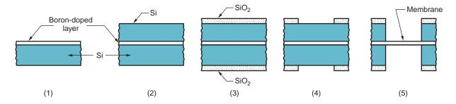
**FIGURE 36.9** Formation of a thin membrane in a silicon substrate: (1) silicon substrate is doped with boron, (2) a thick layer of silicon is applied on top of the doped layer by epitaxial deposition, (3) both sides are thermally oxidized to form a  $SiO_2$  resist on the surfaces, (4) the resist is patterned by lithography, and (5) anisotropic etching is used to remove the silicon except in the boron-doped layer.
