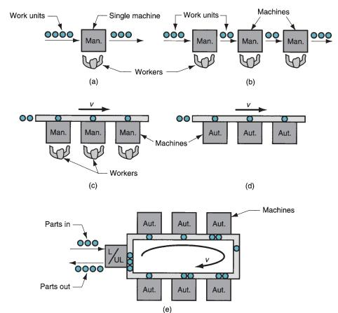
FIGURE 39.10 Types of group technology machine cells: (a) single machine, (b) multiple machines with manual handling, (c) multiple machines with mechanized handling, (d) flexible manufacturing cell, and (e) flexible manufacturing system. Key: Man = manual operation; Aut = automated station.
