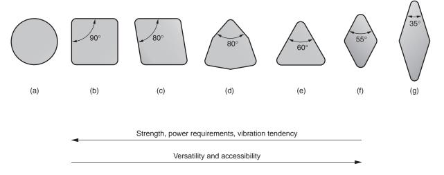
**FIGURE 23.10** Common insert shapes: (a) round, (b) square, (c) rhombus with two 80° point angles, (d) hexagon with three 80° point angles, (e) triangle (equilateral), (f) rhombus with two 55° point angles, (g) rhombus with two 35° point angles. Also shown are typical features of the geometry. Strength, power requirements, and tendency for vibration increase as we move to the left; whereas versatility and accessibility tend to be better with the geometries at the right.
