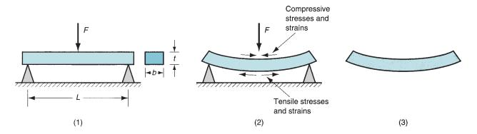
**FIGURE 3.10** Bending of a rectangular cross section results in both tensile and compressive stresses in the material: (1) initial loading; (2) highly stressed and strained specimen; and (3) bent part.
