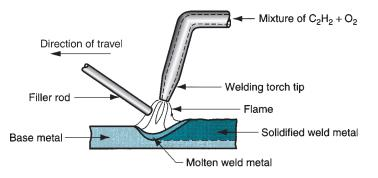
FIGURE 30.21 A typical oxyacetylene welding operation (OAW).
