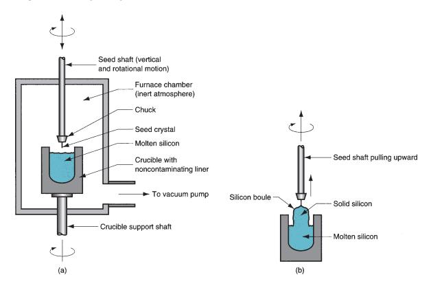
**FIGURE 34.5** The Czochralski process for growing single-crystal ingots of silicon: (a) initial setup prior to start of crystal pulling, and (b) during crystal pulling to form the boule.
