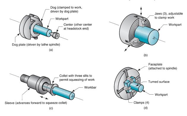
**FIGURE 22.8** Four workholding methods used in lathes: (a) mounting the work between centers using a dog, (b) three-jaw chuck, (c) collet, and (d) faceplate for noncylindrical workparts.
