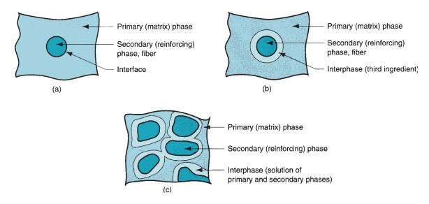
**FIGURE 9.4** Interfaces and interphases between phases in a composite material: (a) direct bonding between primary and secondary phases; (b) addition of a third ingredient to bond the primary and secondary phases and form an interphase; and (c) formation of an interphase by solution of the primary and secondary phases at their boundary.
