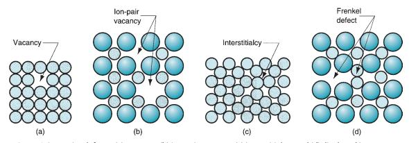
FIGURE 2.9 Point defects: (a) vacancy, (b) ion-pair vacancy, (c) interstitialcy, and (d) displaced ion.
