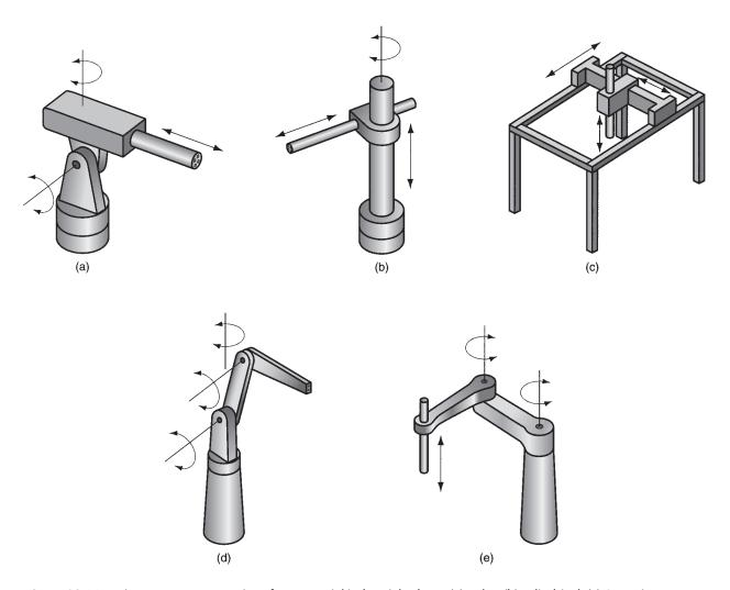
**FIGURE 38.14** Five common anatomies of commercial industrial robots: (a) polar, (b) cylindrical, (c) Cartesian coordinate, (d) jointed-arm, and (e) SCARA, or selectively compliant assembly robot arm.
