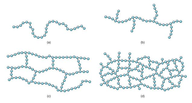
**FIGURE 8.7** Various structures of polymer molecules: (a) linear, characteristic of thermoplastics; (b) branched; (c) loosely cross-linked as in an elastomer; and (d) tightly cross-linked or networked structure as in a thermoset.
