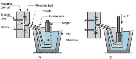
FIGURE 11.13 Cycle in hotchamber casting: (1) with die closed and plunger withdrawn, molten metal flows into the chamber; (2) plunger forces metal in chamber to flow into die, maintaining pressure during cooling and solidification; and (3) plunger is withdrawn, die is opened, and solidified part is ejected. Finished part is shown in (4).
