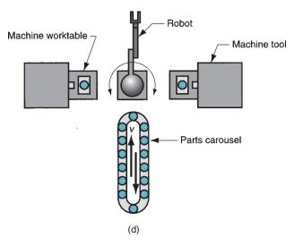
FIGURE 39.11 Four of the five FMS layout types: (a) in-line, (b) ladder, (c) open field, and (d) robot-centered cell. Key: Aut = automated station; L/UL = load/unload station; Insp = inspection station; AGV = automated guided vehicle; AGVS = automated guided vehicle system.
