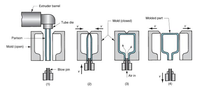
**FIGURE 13.30** Extrusion blow molding: (1) extrusion of parison; (2) parison is pinched at the top and sealed at the bottom around a metal blow pin as the two halves of the mold come together; (3) the tube is inflated so that it takes the shape of the mold cavity; and (4) mold is opened to remove the solidified part.
