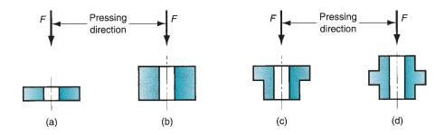
**FIGURE 16.16** Four classes of PM parts—side view shown; cross section is circular: (a) Class I—simple thin shapes that can be pressed from one direction; (b) Class II—simple but thicker shapes that require pressing from two directions; (c) Class III—two levels of thickness, pressed from two directions; and (d) Class IV—multiple levels of thickness, pressed from two directions, with separate controls for each level to achieve proper densification throughout the compact.
