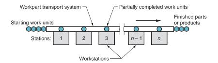
FIGURE 39.2 General configuration of a production line.
