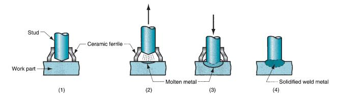
**FIGURE 30.11** Stud arc welding (SW): (1) stud is positioned; (2) current flows from the gun, and stud is pulled from base to establish arc and create a molten pool; (3) stud is plunged into molten pool; and (4) ceramic ferrule is removed after solidification.
