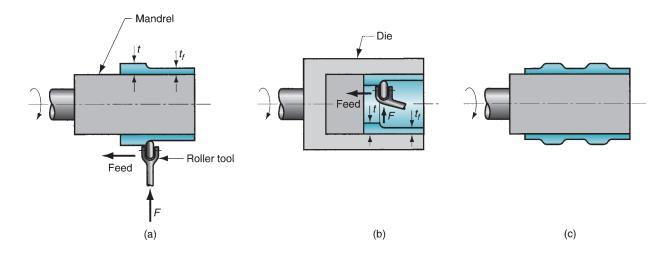
FIGURE 20.44 Tube spinning: (a) external; (b) internal; and (c) profiling.
