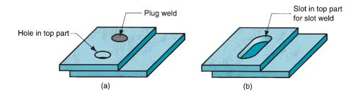
FIGURE 29.5 (a) Plug weld; and (b) slot weld.
