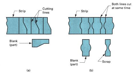
**FIGURE 20.8** (a) Cutoff and (b) parting.
