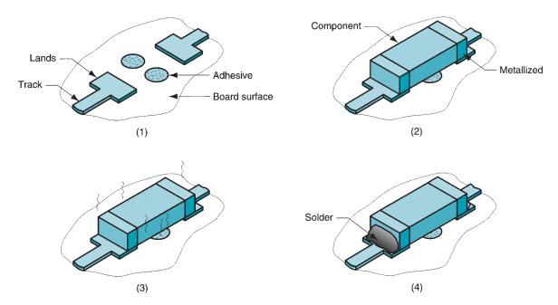
**FIGURE 35.11** Adhesive bonding and wave soldering, shown here for a discrete capacitor or resistor component: (1) adhesive is applied to areas on the board where components are to be placed; (2) components are placed onto adhesive-coated areas; (3) adhesive is cured; and (4) solder joints are made by wave soldering.
