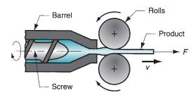
**FIGURE 14.2** Roller die process rubber extrusion followed by rolling.
