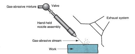
**FIGURE 26.3** Abrasive jet machining (AJM).
