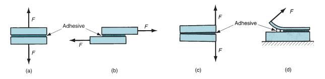
**FIGURE 31.10** Types of stresses that must be considered in adhesive bonded joints: (a) tension, (b) shear, (c) cleavage, and (d) peeling.
