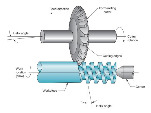
FIGURE 22.37 Thread milling using a form-milling cutter.
