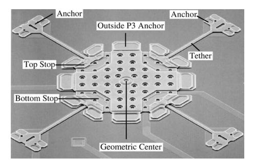
FIGURE 36.2 Micrograph of a microaccelerometer. (Photo courtesy of A. A. Tseng, Arizona State University [4].)
