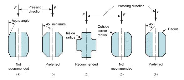
**FIGURE 16.19** Chamfers and corner radii are accomplished but certain rules should be observed: (a) avoid acute chamfer angles; (b) larger angles are preferred for punch rigidity; (c) small inside radius is desirable; (d) full outside corner radius is difficult because punch is fragile at corner's edge; (e) outside corner problem can be solved by combining radius and chamfer.
