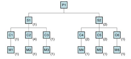
FIGURE 41.4 Product structure for assembled product P1. (Based on data in [3].)
