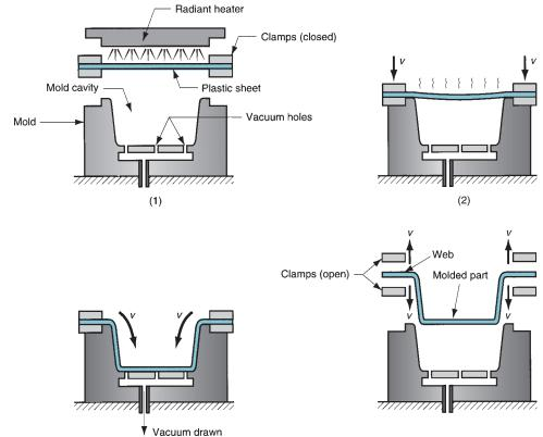
FIGURE 13.35 Vacuum thermoforming: (1) a flat plastic sheet is softened by heating; (2) the softened sheet is placed over a concave mold cavity; (3) a vacuum draws the sheet into the cavity; and (4) the plastic hardens on contact with the cold mold surface, and the part is removed and subsequently trimmed from the web.
