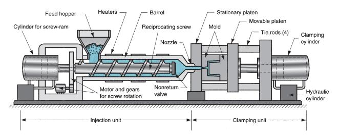
**FIGURE 13.21** Diagram of an injection molding machine, reciprocating screw type (some mechanical details are simplified).
