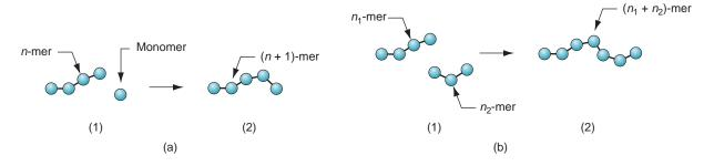
**FIGURE 8.4** Model of step polymerization showing the two types of reactions occurring: (a) n-mer attaching a single monomer to form a (n + 1)-mer; and (b)  $n_1$ -mer combining with  $n_2$ -mer to form a  $(n_1 + n_2)$ -mer. Sequence is shown by (1) and (2).
