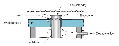
FIGURE 26.5 Electrochemical deburring (ECD).
