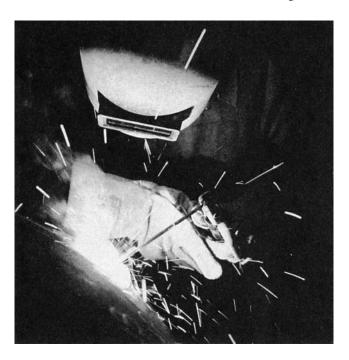
FIGURE 30.2 Shielded metal arc welding (stick welding) performed by a (human) welder. (Photo courtesy of Hobart Brothers, Troy, Ohio.)
