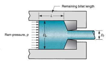
FIGURE 19.33 Pressure and other variables in direct extrusion.
