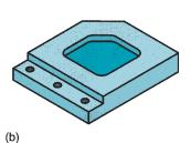
**FIGURE 22.1** Machined parts are classified as (a) rotational, or (b) nonrotational, shown here by block and flat parts.
