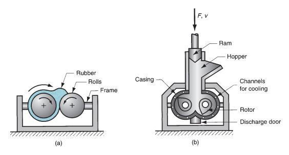
**FIGURE 14.1** Mixers used in rubber processing: (a) two-roll mill and (b) Banbury-type internal mixer. These machines can also be used for mastication of natural rubber.
