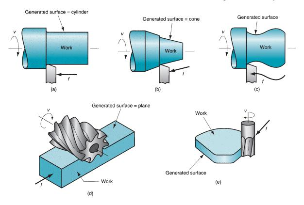
**FIGURE 22.2** Generating shape in machining: (a) straight turning, (b) taper turning, (c) contour turning, (d) plain milling, and (e) profile milling.
