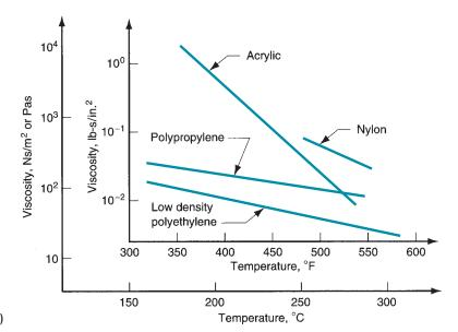
FIGURE 13.2 Viscosity as a function of temperatures for selected polymers at a shear rate of 10<sup>3</sup> s<sup>-1</sup>. (Data compiled from [12].)
