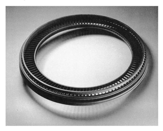
**FIGURE 11.9** A one-piece compressor stator with 108 separate airfoils made by investment casting. (Courtesy of Howmet Corp.).
