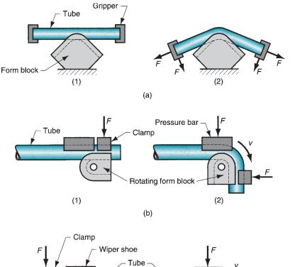
FIGURE 20.49 Tube bending methods: (a) stretch bending, (b) draw bending, and (c) compression bending. For each method: (1) start of process, and (2) during bending. Symbols *v* and *F* indicate motion and applied force, respectively.
