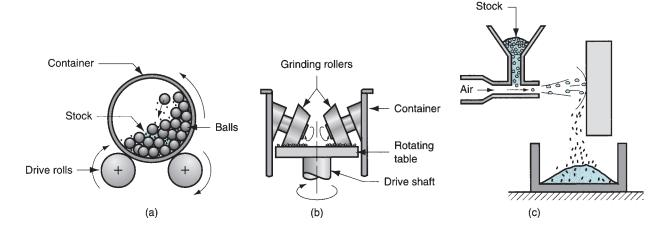
**FIGURE 17.3** Mechanical methods of producing ceramic powders: (a) ball mill, (b) roller mill, and (c) impact grinding.
