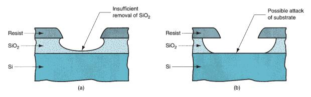
FIGURE 34.14 Two problems in etching: (a) under-etching and (b) over-etching.
