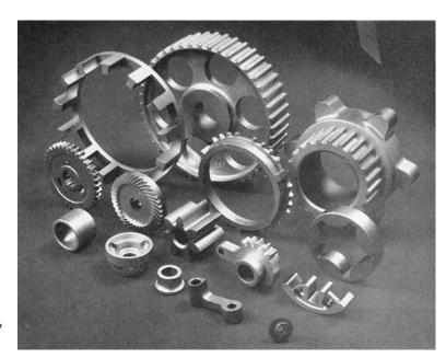
FIGURE 16.1 A collection of powder metallurgy parts. (Courtesy of Dorst America, Inc.)
