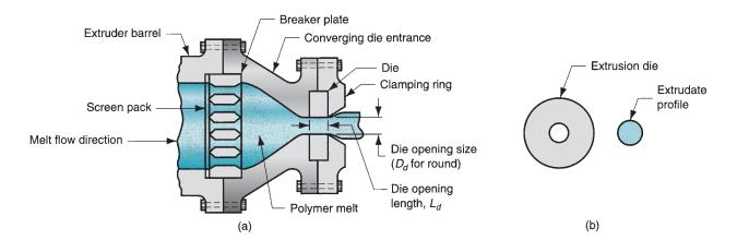
**FIGURE 13.8** (a) Side view cross section of an extrusion die for solid regular shapes, such as round stock; (b) front view of die, with profile of extrudate. Die swell is evident in both views. (Some die construction details are simplified or omitted for clarity.)
