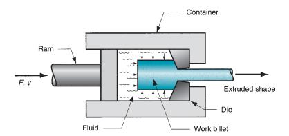
FIGURE 19.38 Hydrostatic extrusion.
