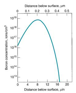
FIGURE 28.4 Profile of surface chemistry as treated by ion implantation. (Source: [17].) Shown here is a typical plot for boron implanted in silicon. Note the difference in profile shape and depth of altered layer compared to diffusion in Figure 28.3.
