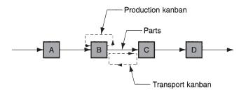
**FIGURE 41.5** Operation of a kanban system between workstations.
