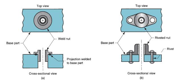
FIGURE 32.7 Captive threaded fasteners: (a) weld nut and (b) riveted nut.
