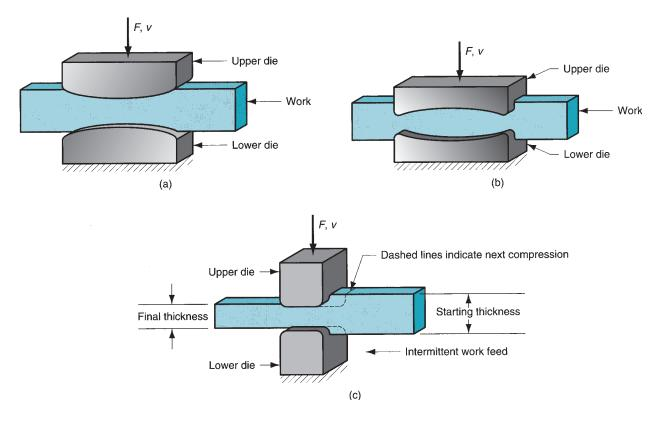
FIGURE 19.13 Several open-die forging operations: (a) fullering, (b) edging, and (c) cogging.
