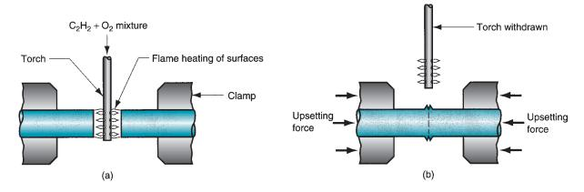
**FIGURE 30.23** An application of pressure gas welding: (a) heating of the two parts, and (b) applying pressure to form the weld.
