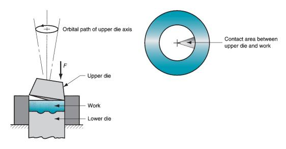
FIGURE 19.27 Orbital forging. At end of deformation cycle, lower die lifts to eject part.
