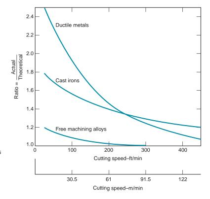
FIGURE 24.2 Ratio of actual surface roughness to ideal surface roughness for several classes of materials. (Source: General Electric Co. data [14].)
