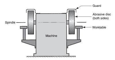
**FIGURE 25.14** Typical configuration of a disk grinder.
