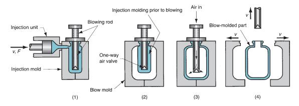
**FIGURE 13.32** Injection blow molding: (1) parison is injected molded around a blowing rod; (2) injection mold is opened and parison is transferred to a blow mold; (3) soft polymer is inflated to conform to the blow mold; and (4) blow mold is opened, and blown product is removed.
