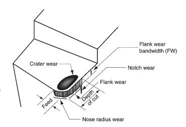
of worn cutting tool, showing the principal locations and types of wear that occur.
