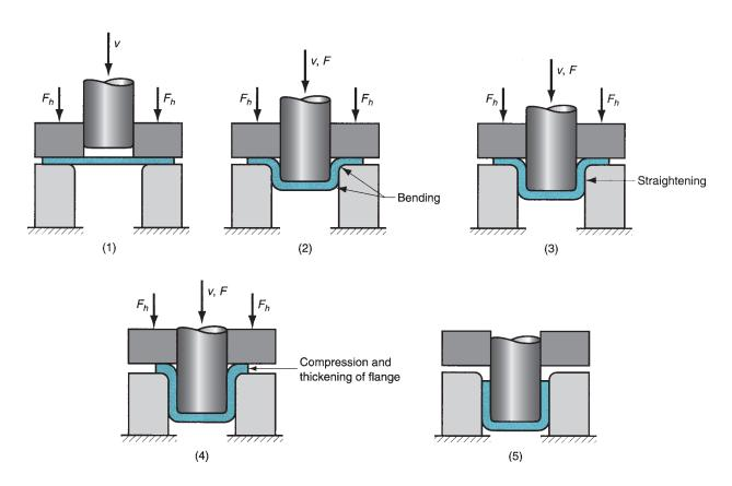
**FIGURE 20.20** Stages in deformation of the work in deep drawing: (1) punch makes initial contact with work, (2) bending, (3) straightening, (4) friction and compression, and (5) final cup shape showing effects of thinning in the cup walls. Symbols: v = motion of punch, F = punch force, F = blankholder force.
