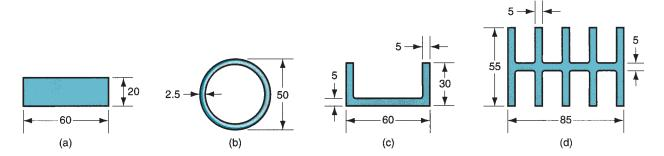
FIGURE P19.32 Cross-sectional shapes for Problem 19.32 (dimensions are in mm): (a) rectangular bar, (b) tube, (c) channel, and (d) cooling fins.
