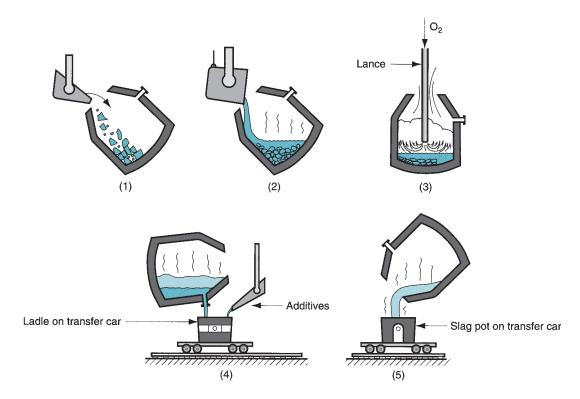
**FIGURE 6.8** BOF sequence during processing cycle: (1) charging of scrap and (2) pig iron; (3) blowing (Figure 6.7); (4) tapping the molten steel; and (5) pouring off the slag.
