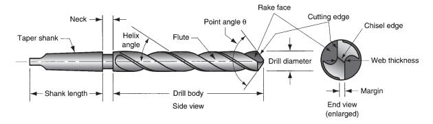
FIGURE 23.12 Standard geometry of a twist drill.
