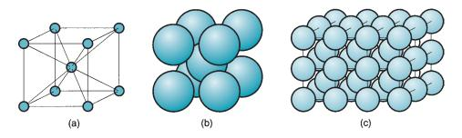
**FIGURE 2.7** Body-centered cubic (BCC) crystal structure: (a) unit cell, with atoms indicated as point locations in a three-dimensional axis system; (b) unit cell model showing closely packed atoms (sometimes called the hard-ball model); and (c) repeated pattern of the BCC structure.
