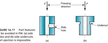
FIGURE 16.17 to be avoided in PM: (a) side holes and (b) side undercuts. Part ejection is impossible.
