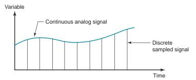
command signals are sent to actuators that operate the process. In this section, we discuss the hardware devices that enable this communication between the process and the controller. The devices include analog-to-digital converters, digital-to-analog converters, contact input/output interfaces, and pulse counters and generators.
