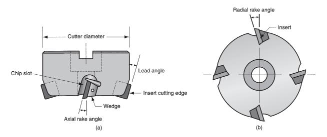
FIGURE 23.17 Tool geometry elements of a four-tooth face milling cutter: (a) side view and (b) bottom view.
