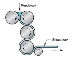
**FIGURE 13.17** A typical roll configuration in calendering.
