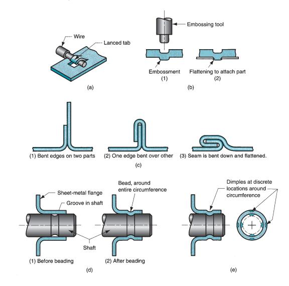
**FIGURE 32.18** Integral fasteners: (a) lanced tabs to attach wires or shafts to sheetmetal, (b) embossed protrusions, similar to riveting, (c) single-lock seaming, (d) beading, and (e) dimpling. Numbers in parentheses indicate sequence in (b), (c), and (d).
