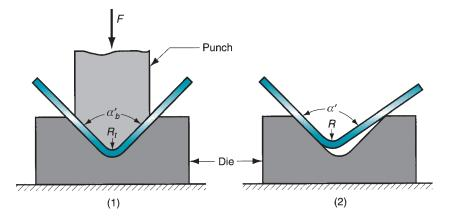
**FIGURE 20.13** Springback in bending shows itself as a decrease in bend angle and an increase in bend radius: (1) during the operation, the work is forced to take the radius  $R_t$  and included angle  $\alpha'$   $_t$  = determined by the bending tool (punch in V-bending); (2) after the punch is removed, the work springs back to radius R and included angle  $\alpha'$ . Symbol: F = applied bending force.
