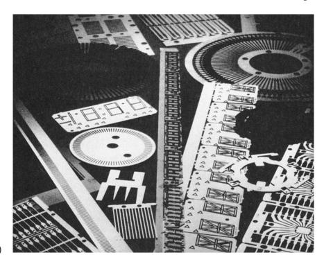
FIGURE 26.18 Parts made by chemical blanking. (Courtesy of Buckbee-Mears, St. Paul.)
