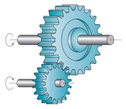
**FIGURE 22.38** Two meshing spur gears.
