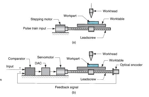
FIGURE 38.10 Two types of motion control in numerical control: (a) open loop and (b) closed loop.
