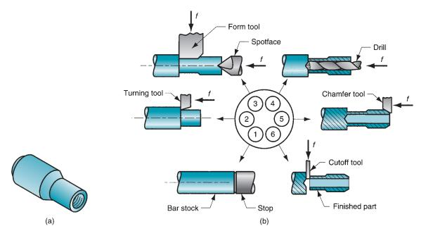
**FIGURE 22.9** (a) Type of part produced on a six-spindle automatic bar machine; and (b) sequence of operations to produce the part: (1) feed stock to stop, (2) turn main diameter, (3) form second diameter and spotface, (4) drill, (5) chamfer, and (6) cutoff.
