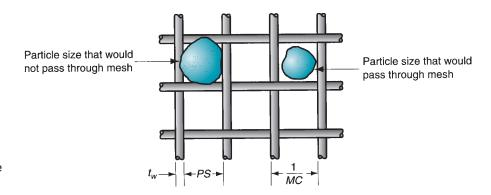
**FIGURE 16.2** Screen mesh for sorting particle sizes.
