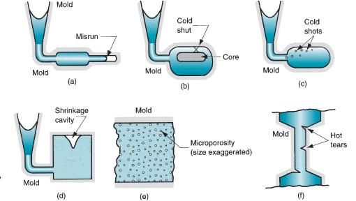
FIGURE 11.22 Some common defects in castings: (a) misrun, (b) cold shut, (c) cold shot, (d) shrinkage cavity, (e) microporosity, and (f) hot tearing.
