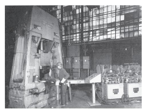
FIGURE 19.19 Drop forging hammer, fed by conveyor and heating units at the right of the scene. (Photo courtesy of Chambersburg Engineering Company, Chambersburg, Pennsylvania)
