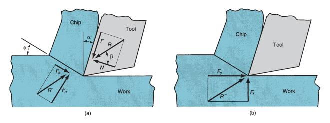
**FIGURE 21.10** Forces in metal cutting: (a) forces acting on the chip in orthogonal cutting, and (b) forces acting on the tool that can be measured.
