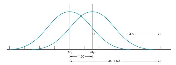
**FIGURE 42.3** Normal distribution shift by  $1.5\sigma$  from original mean and consideration of only one tail of the distribution (at right). Key:  $\mu_1 =$  mean of original distribution,  $\mu_2 =$  mean of shifted distribution,  $\sigma =$  standard distribution.
