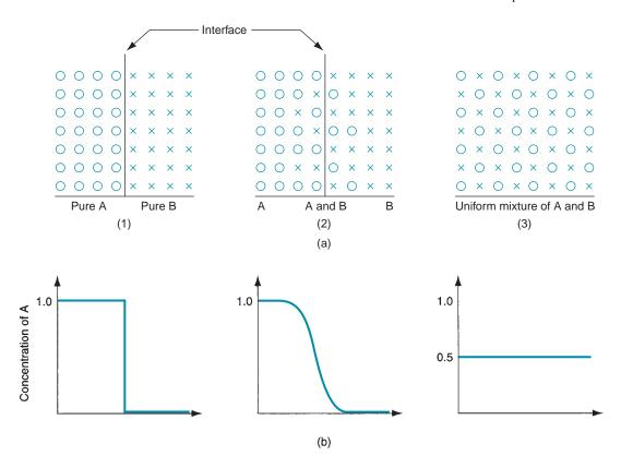
**FIGURE 4.2** Mass diffusion: (a) model of atoms in two solid blocks in contact: (1) at the start when two pieces are brought together, they each have their individual compositions; (2) after some time, an exchange of atoms has occurred; and (3) eventually, a condition of uniform concentration occurs. The concentration gradient dc/dx for metal A is plotted in (b) of the figure.
