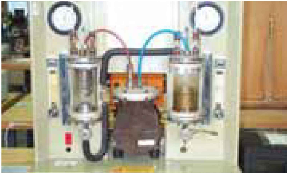
Refrigeration cycle machine.
