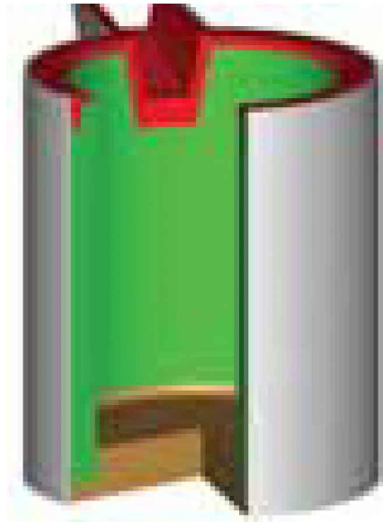
Rammed induction furnace.
