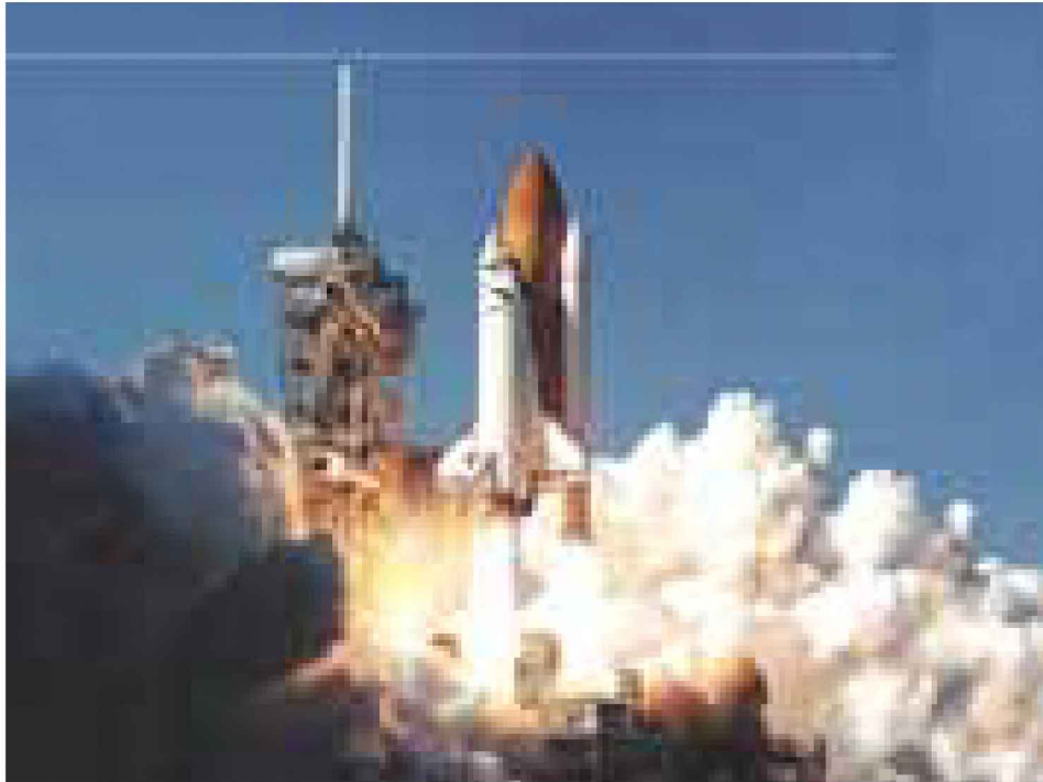
Space shuttle carries oxygen and hydrogen in tanks which hold the gases below -150^{\circ}\text{C}
