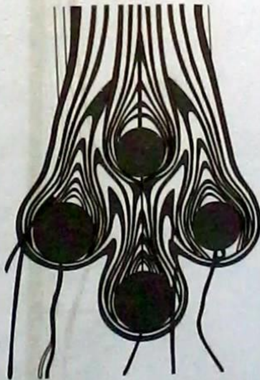
Fig. 5.10 Interferometer photograph showing the boundary layer interaction between four heated horizontal cylinders in natural convection
