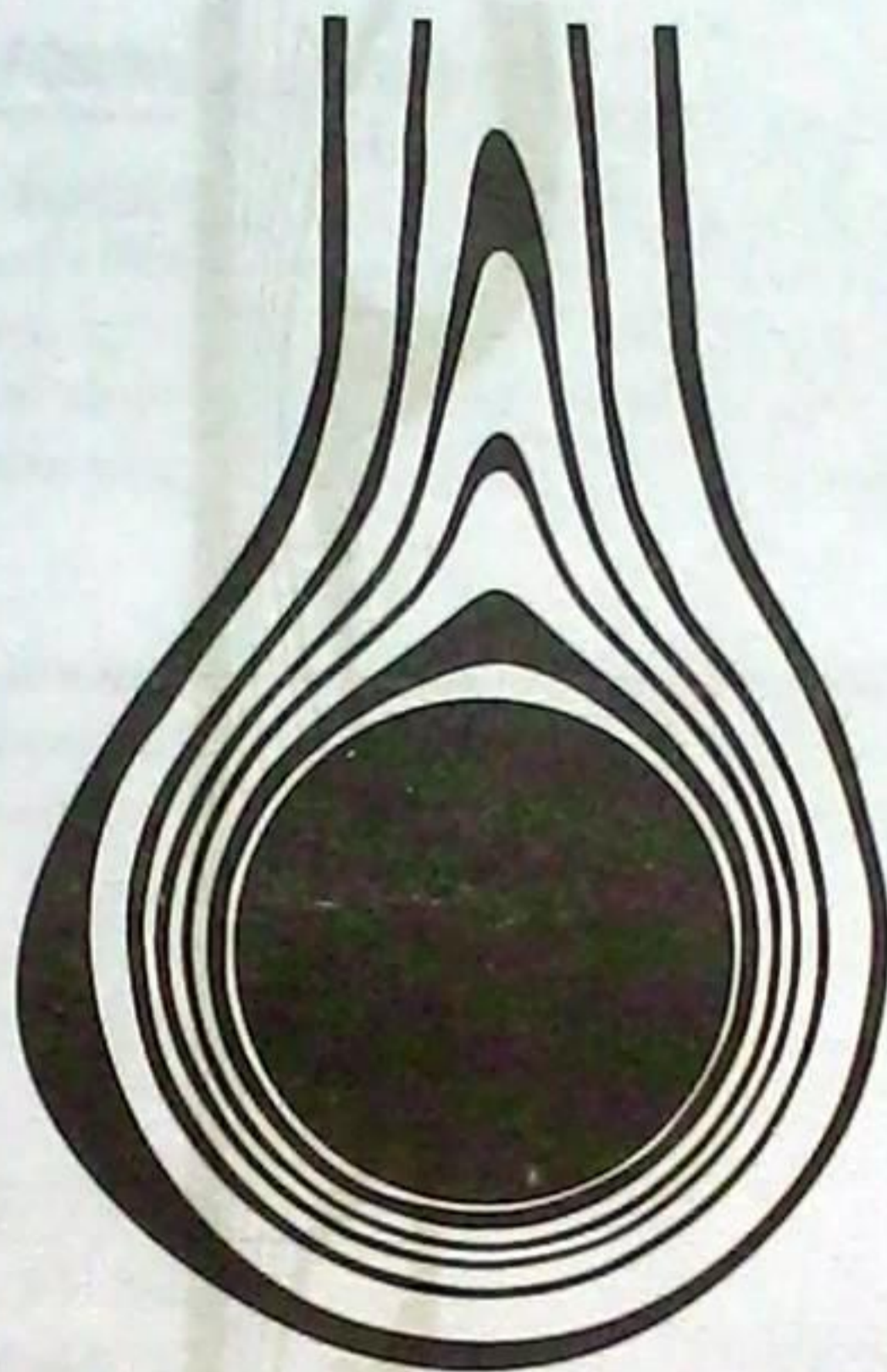
Fig. 5.9 Interferometer photograph showing lines of constant temperature around a heated horizontal cylinder in natural convection
