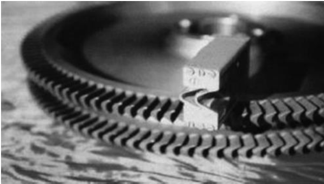
FIGURE 11.15 Profile of turbine blade by ECM.
