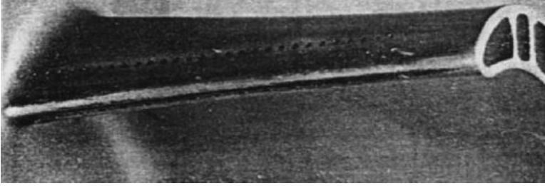
FIGURE 12.33 Electron beam–drilled holes in superalloy turbine blade.
