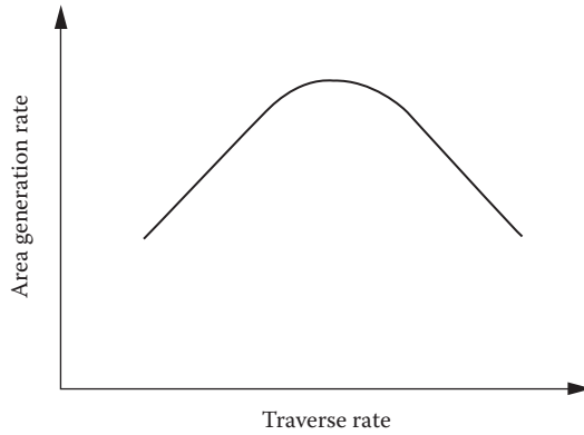
FIGURE 10.31 Relationship between traverse rate and area generation rate.
