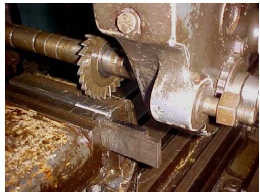
Fig. 4.5.23 Mounting of cutting tools on milling arbours.
