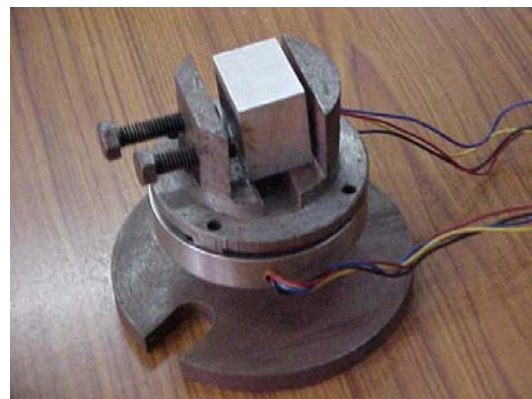
Fig. 10.12 A strain gauge type drilling dynamometer and its major components.
