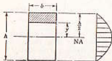
Figure 5-25 Shearing stress is distributed parabolically across a rectangular section.
