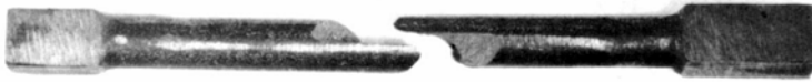
Figure 16.6 Failure in torsion of a circular bar of brittle cast iron, showing a tendency to tensile fracture across a helix on the surface of the specimen.
