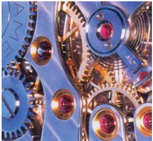
Gear trains inside a mechanical watch
