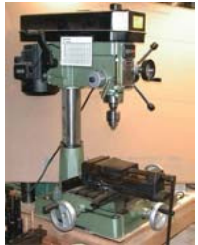
A drill press has a pointed tool which is used for boring holes in hard materials usually by rotating abrasion or repeated blows.
