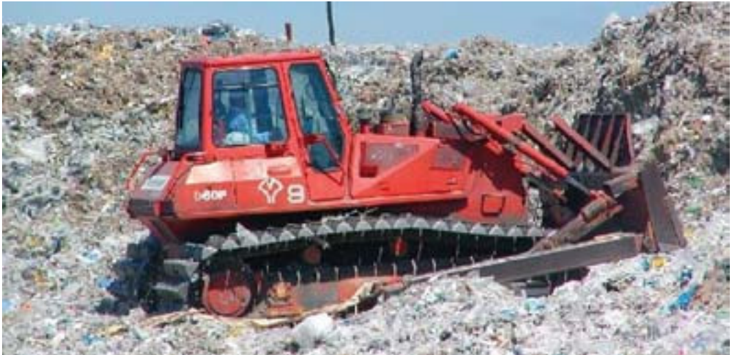
The chain-belt at the bottom of a bulldozer provides powerful grip, spreads weight and force on the ground, and allows to exert high force on the objects to be moved.
