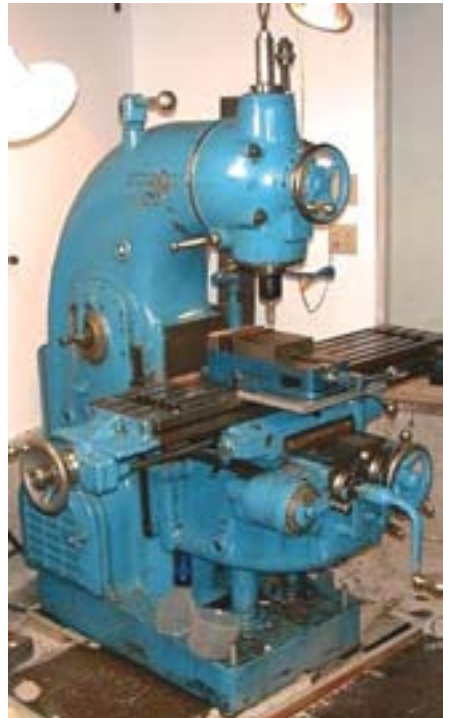
Milling machine is used for dressing surfaces by rotary cutters.
