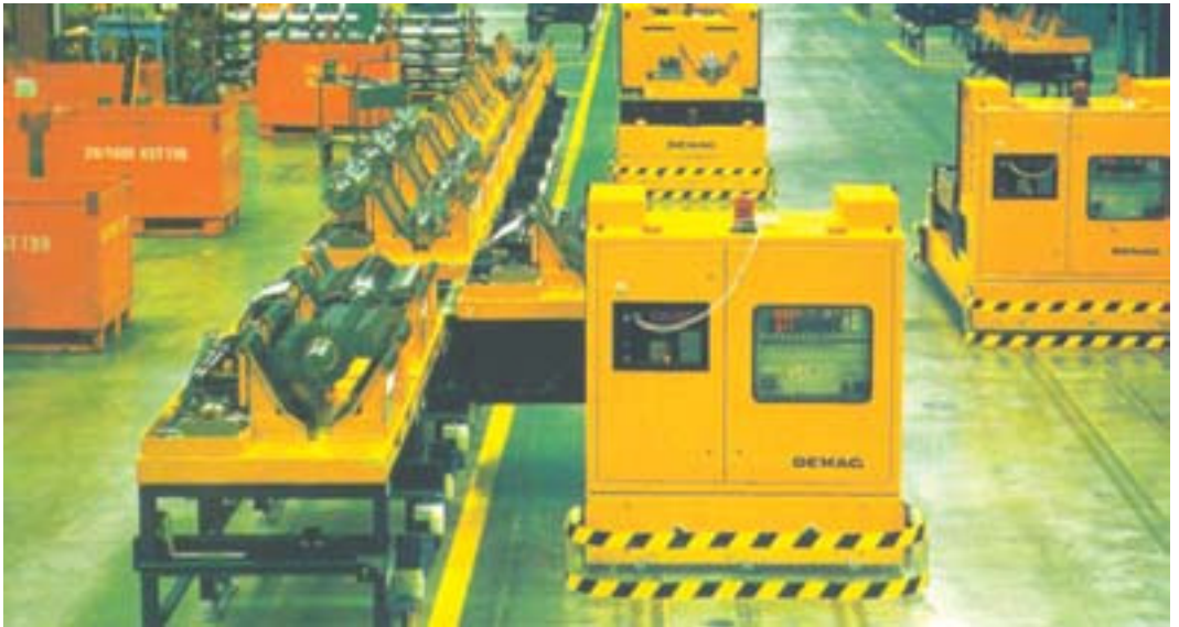
Automated Guided Vehicles, AGVs, operate in many factories. They ferry goods and materials along carefully marked routes. Many AGVs are guided by signals from electrical loops buried under factory floors.
