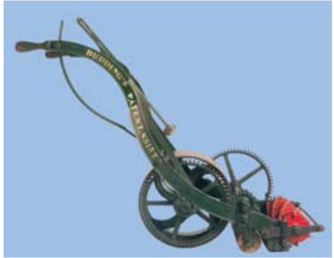
Lawn-mover is a combination of kinematic links.
