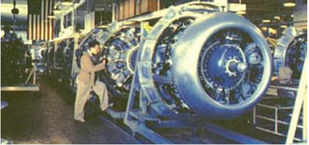
Aircraft engine is being assembled.
