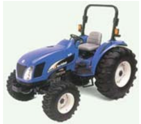
Tractors are specially made to move on rough terrain and exert high power at low speeds.
