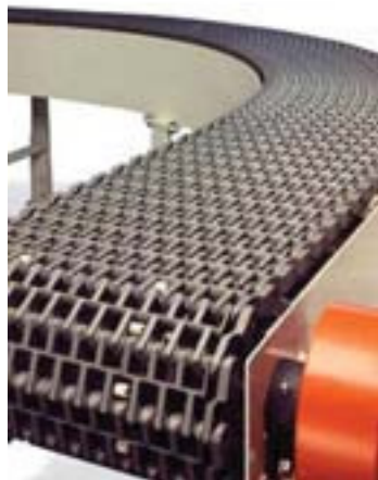
A belt-conveyor that can transport small components.
