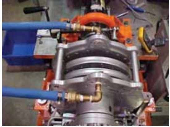
Dynamometers measure the power of the engines.
