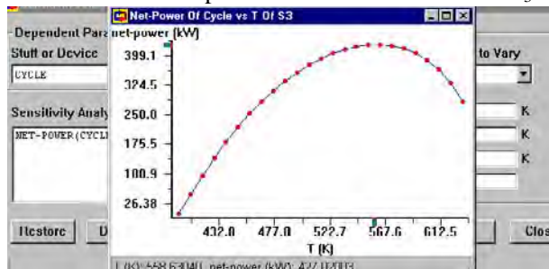
Figure E13.4.3. Endo-reversible cycle Sensitivity analysis.
