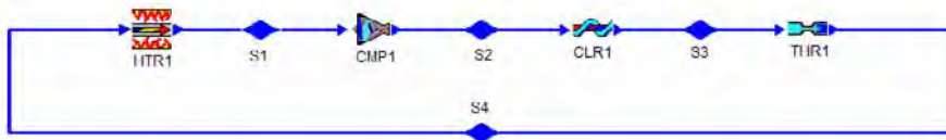
Figure 5.2.4.2. House Heat pump
