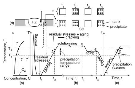
**Figure 16.10** Postweld heat treatment cracking: (a) phase diagram; (b) thermal cycles during welding and heat treating; (c) precipitation C curve; (d) weld cross-section; (e) changes in microstructure.
