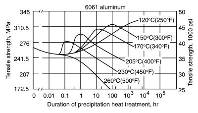
**Figure 15.6** Aging characteristics for 6061-T4 aluminum (9). Modified from *Metals Handbook*, vol. 2, 8th edition, American Society for Metals, 1964, p. 276.
