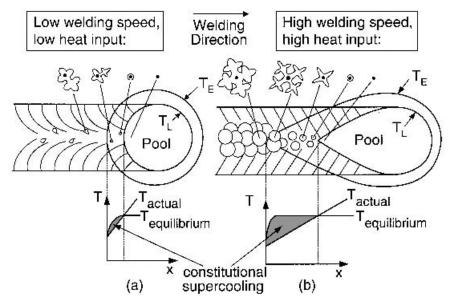
**Figure 7.21** Effect of welding parameters on heterogeneous nucleation: (a) low constitutional supercooling at low welding speed and heat input; (b) heterogeneous nucleation aided by high constitutional supercooling at high welding speed and heat input.
