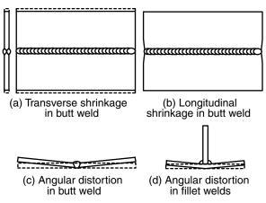
Figure 5.6 Distortion in welded structures. Modified from Welding Handbook (2).
