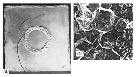
**Figure 16.11** Postweld heat treatment cracking. (a) Circular-patch specimen of Rene 41. From Prager and Shira (4). (b) Scanning electron micrograph showing intergranular cracking. Reprinted from McKeown (29). Courtesy of American Welding Society.
