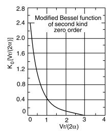
Figure 2.16 Modified Bessel function of second kind and zero order (26).
