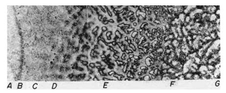
**Figure 17.8** HAZ microstructure of a stationary repair weld of an as-cast carbon steel. Fusion zone: A, B; HAZ: C–F; base metal: G. Reprinted from Aidun and Savage (12). Courtesy of American Welding Society.
