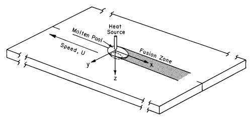
**Figure 2.14** Coordinate system (x, y, z) moving with heat source. From Kou and Le (24).
