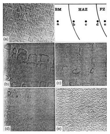
**Figure 16.6** Microstructure of Udimet 700 weld: (a) as-received material (magnification 10,000×); (b) initial solution of fine  $\gamma'$ ; (c) further solution of coarse  $\gamma'$ ; (d) advanced stage of solution of coarse  $\gamma'$ ; (e) weld metal containing fine  $\gamma'$ . (b-d). Magnification 15,000×. Reprinted from Owczarski and Sullivan (13). Courtesy of American Welding Society. Reduced to 84% in reproduction.
