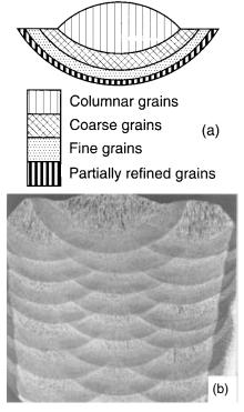
**Figure 17.5** Grain refining in multiple-pass welding: (a) single-pass weld; (b) microstructure of multiple-pass weld. Reprinted from Evans (10). Courtesy of American Welding Society.
