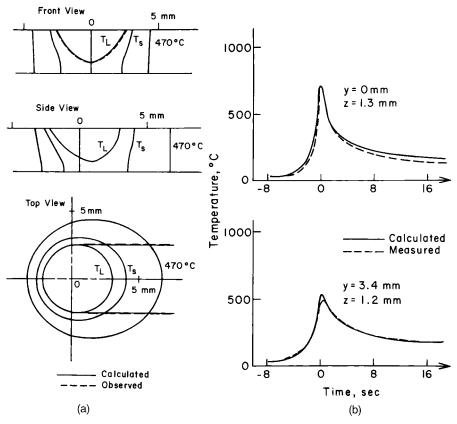
**Figure 2.20** Computer simulation of GTAW of 3.2-mm-thick 6061 aluminum, 110 A, 10 V, and  $4.23 \,\text{mm/s}$ : (a) fusion boundaries and isotherms; (b) thermal cycles. From Kou and Le (24).
