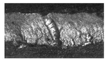
**Figure 3.25** Wormhole porosity in weld metal. From Jackson (55).
