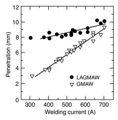
**Figure 1.31** Weld penetration in GMAW and laser-assisted GMAW using CO<sub>2</sub> laser at 5.7 kW. Reprinted from Hyatt et al. (24). Courtesy of American Welding Society.
