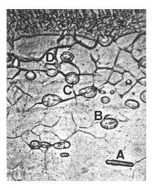
**Figure 12.6** PMZ of an electric resistance spot weld of 18-Ni maraging steel showing constitutional liquation. The fusion zone is at the top. Magnification 385×. Reprinted from Pepe and Savage (6). Courtesy of American Welding Society.
