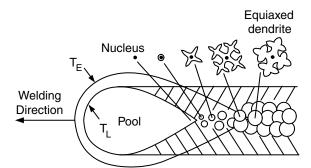
Figure 7.14 Heterogeneous nucleation and formation of equiaxed grains in weld metal.
