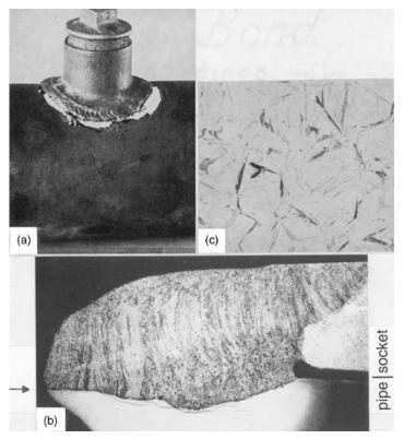
**Figure 17.35** Failure in a socket/pipe weldment: (a) fracture region (magnification  $0.4\times$ ); (b) underbead cracking (magnification  $7.5\times$ ); (c) martensitic microstructure in the cracked region (magnification  $370\times$ ). Reprinted, with permission, from Naumann (56).
