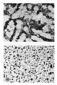
**Figure 17.7** Microstructure of a carbon steel: (a) as-cast condition; (b) after homogenization. Reprinted from Aidun and Savage (12). Courtesy of American Welding Society.
