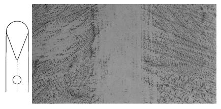
**Figure 9.19** Weld centerline austenite in an autogenous gas—tungsten arc weld of 309 stainless steel solidified as primary ferrite. From Kou and Le (9).
