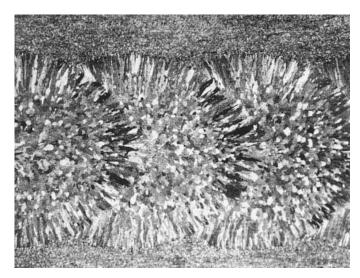
**Figure 7.29** Equiaxed grains in pulsed arc weld of 6061 aluminum (magnification 9×). From Kou and Le (44).
