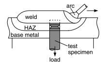
Figure 17.20 Implant test for hydrogen cracking.
