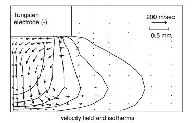
**Figure 4.7** Velocity and temperature fields in an arc produced by a tungsten electrode with a flat end. The isotherms from right to left are 11,000, 13,000, 15,000, 17,000, 19,000, and 21,000 K. Modified from Tsai and Kou (1).
