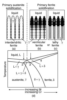
**Figure 9.2** Schematics showing solidification and postsolidification transformation in Fe–Cr–Ni welds: (a) interdendritic ferrite; (b) vermicular ferrite; (c) lathy ferrite; (d) vertical section of ternary-phase diagram at approximately 70% Fe.
