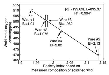
**Figure 3.22** Weld metal oxygen content in steel as a function of flux basicity in flux-core arc welding. Reprinted from Baune et al. (46). Courtesy of American Welding Society.
