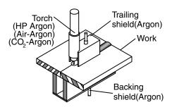
**Figure 3.2** Gas-tungsten arc welding of titanium with additional gas shielding. Reprinted from Harwig et al. (3). Courtesy of American Welding Society.
