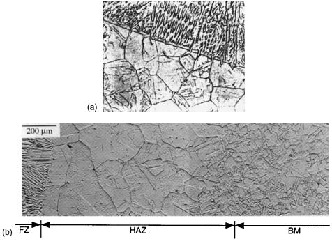
**Figure 12.9** Ghost GBs near fusion boundary of gas-tungsten arc welds: (a) 18-Ni maraging steel; magnification 125×. Reprinted from Pepe and Savage (6). Courtesy of American Welding Society. (b) Ni-base superalloy 690. Reprinted from Lee and Kuo (14).
