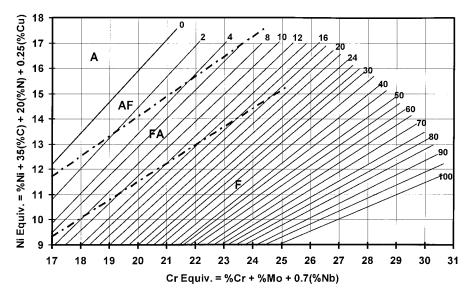
**Figure 9.11** WRC-1992 diagram for predicting weld ferrite content and solidification mode. Reprinted from Kotecki and Siewert (16). Courtesy of American Welding Society.
