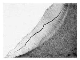
**Figure 17.18** Underbead crack in a low-alloy steel HAZ (magnification 8×). Reprinted from Bailey (27).
