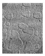
**Figure 16.7** HAZ of Udimet 700 showing reprecipitation of fine  $\gamma'$  in region where coarse  $\gamma'$  begins to dissolve. Magnification 16,000×. Reprinted from Owczarski and Sullivan (13). Courtesy of American Welding Society.
