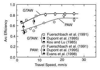
Figure 2.3 Arc efficiencies in GTAW and PAW.
