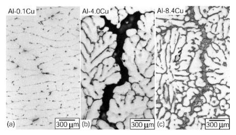
**Figure 11.14** Aluminum welds with three different levels of Cu:(a) almost no Cu;(b) 4% Cu;(c) 8% Cu.
