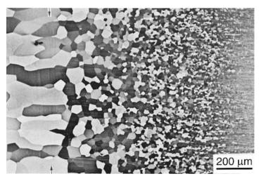
**Figure 14.7** Grain growth in electron beam weld of molybdenum, arrows indicating fusion boundary. Reprinted from Wadsworth et al. (9). Copyright 1983 with permission from Elsevier Science.
