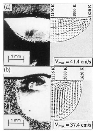
**Figure 4.21** Convection in stationary laser weld pools of steels with (a) 20 ppm sulfur and (b) 150 ppm sulfur. Reprinted from Pitscheneder et al. (36). Courtesy of American Welding Society.
