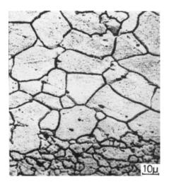
**Figure 18.16** Intergranular corrosion near fusion boundary of 347 stainless steel. From Ikawa et al. (18).
