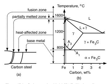
**Figure 17.1** Carbon steel weld: (a) HAZ; (b) phase diagram.
