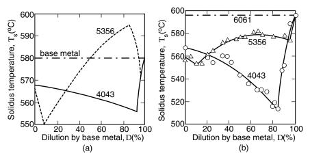
**Figure 13.11** Variation of weld metal solidus temperature with dilution: (a) in 6082 aluminum (5); (b) in 6061 aluminum (12). (a) from Gittos et al. (5) and (b) from Miyazaki et al. (12). Reprinted from *Welding Journal*, Courtesy of American Welding Society.
