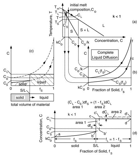
**Figure 6.4** Solute redistribution during solidification with complete diffusion in liquid and no diffusion in solid: (a) phase diagram; (b)  $C_L(f_s)$  and  $C_S(f_s)$ ; (c) composition profiles in solid and liquid; (d) conservation of solute.
