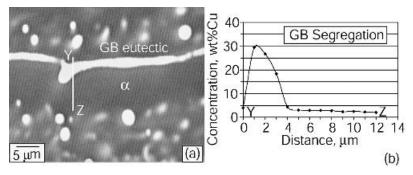
**Figure 12.14** Grain boundary segregation in PMZ of 2219 aluminum weld: (a) electron micrograph; (b) composition profile. Reprinted from Huang and Kou (2). Courtesy of American Welding Society.
