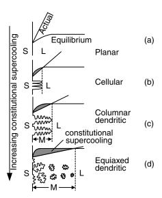
**Figure 6.11** Effect of constitutional supercooling on solidification mode: (*a*) planar; (*b*) cellular; (*c*) columnar dendritic; (*d*) equiaxed dendritic (S, L, and M denote solid, liquid, and mushy zone, respectively).
