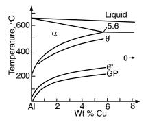
**Figure 15.2** Metastable solvus curves for GP,  $\theta''$ , and  $\theta'$  in Al–Cu phase diagram. From Hornbogeni (1) and Beton and Rollason (2).
