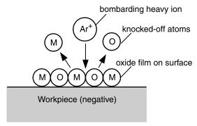
Figure 1.13 Surface cleaning action in GTAW with DC electrode positive.
