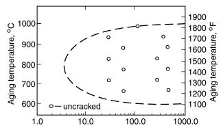
**Figure 16.14** Crack susceptibility C curve for a Rene 41 solution annealed before welding and crack test data (○) from a Rene 41 overaged before welding. Reprinted from Berry and Hughes (36). Courtesy of American Welding Society.
