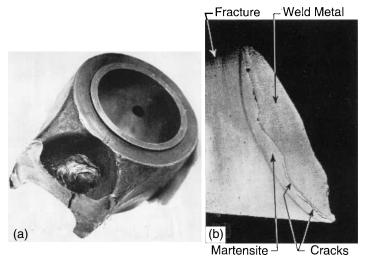
**Figure 17.36** Failure of an oil engine connecting rod: (a) top end of connecting rod showing fracture surface and weld deposit; (b) section through weld deposit showing underbead cracking (magnification  $3.5\times$ ). From Hutchings and Unterweiser (57).
