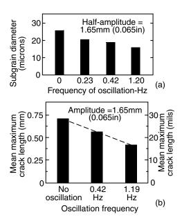
**Figure 8.18** Effect of magnetic arc oscillation on gas-tungsten arc welds of HY-80 steel: (a) refining of microstructure within grains; (b) solidification cracking. Modified from Tseng and Savage (17).
