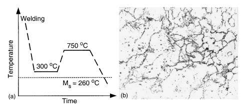
**Figure 18.26** Improper postweld heat treatment and resultant microstructure of a 12% Cr martensitic steel (magnification 500×). Reprinted, with permission, from Castro and De Cadenet (4). Copyright 1974 Cambridge University Press.
