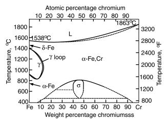
**Figure 18.1** Fe–Cr phase diagram (2).
