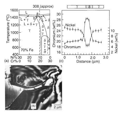
**Figure 10.3** Microsegregation in 308 stainless steel weld: (a) phase diagram; (b) TEM micrograph of a dendrite arm; (c) microsegregation across the arm. Reprinted from David et al. (10). Courtesy of American Welding Society.
