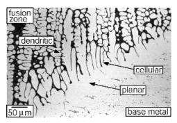
**Figure 8.7** Planar-to-cellular and cellular-to-dendritic transitions in 1100 Al welded with 4047 filler.
