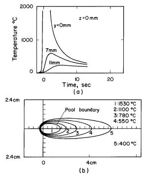
**Figure 2.19** Calculated results similar to those in Figure 2.18 but with welding speed of 6.2 mm/s and heat input of 5000 W.
