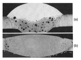
**Figure 10.16** Powder metallurgy Al–10Fe–5Ce alloy gas–tungsten arc welded with Al–5Si filler metal: (*a*) AC; (*b*) DCEN. Reprinted from Metzger (54). Courtesy of American Welding Society.
