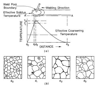
**Figure 12.8** Schematic representation of constitutional liquation and formation of ghost GB network. Reprinted from Pepe and Savage (6). Courtesy of American Welding Society.
