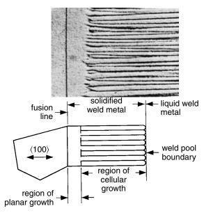
**Figure 8.6** Planar-to-cellular transition in an autogenous weld of Fe–49Ni. Modified from Savage et al. (2).
