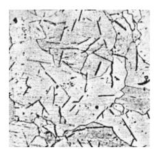
**Figure 3.6** Iron nitride in a ferrite matrix (×500). From Seferian (15).
