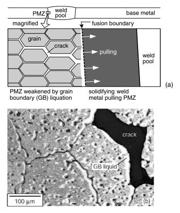
**Figure 13.5** Formation of PMZ cracking in a full-penetration aluminum weld: (a) schematic; (b) PMZ cracking in 6061 aluminum. From Huang and Kou (13).
