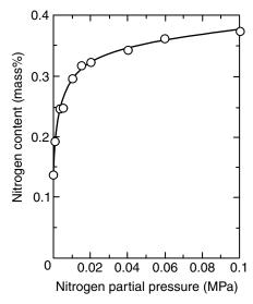
**Figure 3.5** Effect of nitrogen partial pressure in Ar–N<sub>2</sub> shielding gas on nitrogen content in welds of duplex stainless steel. Reprinted from Sato et al. (14).
