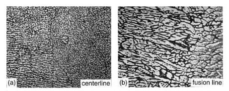
**Figure 8.11** Transverse cross-section of gas-tungsten arc weld in 6061 aluminum: (a) finer microstructure near centerline; (b) coarser microstructure near fusion line. Magnification 115×. Reprinted from Kou et al. (6). Courtesy of American Welding Society.
