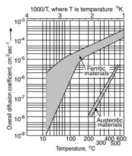
**Figure 17.17** Diffusion coefficient of hydrogen in ferritic and austenitic materials as a function of temperature. Modified from Coe (21).
