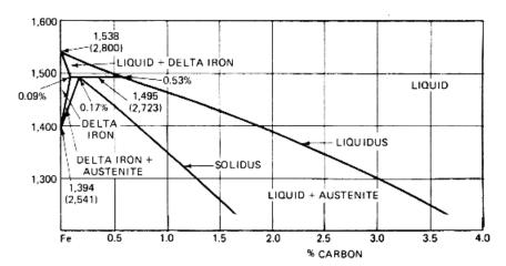
Figure 11.20 Iron-carbon phase diagram.
