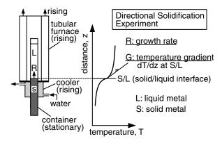
**Figure 6.2** Directional solidification experiment.
