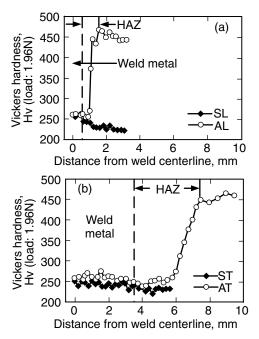
**Figure 16.8** Hardness profiles in Inconel 718 welds in as-welded condition: (a) laser welds; (b) gas-tungsten arc welds. S: solutionized; A: aged after solutionization; L: laser welded; T: gas-tungsten arc welded. Broken line indicates fusion line. From Hirose et al. (15).
