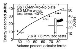
**Figure 9.29** Subsize Charpy V-notch toughness values as a function of volume fraction of acicular ferrite in submerged arc welds. Reprinted from Fleck et al. (49). Courtesy of American Welding Society.
