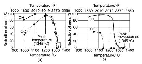
**Figure 13.4** Hot ductility response of Cabot alloy 214 with two different boron levels: (a) 0.0002 wt% B; (b) 0.003 wt% B. OH, testing done on heating to 1345°C; OC, on cooling from 1345°C. From Cieslak (6). Reprinted from *ASM Handbook*, vol. 6, ASM International.
