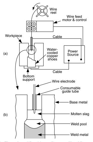
**Figure 1.22** Electroslag welding: (a) overall process; (b) welding area enlarged.
