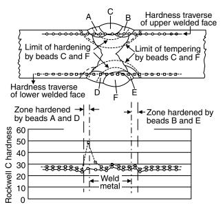
**Figure 17.13** Tempering bead technique for multiple-pass welding of a butt joint in a quenched-and-tempered alloy steel. Reprinted form Linnert (19). Courtesy of American Welding Society.
