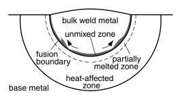
Figure 10.13 Zone of unmixed melted base metal along the fusion boundary.
