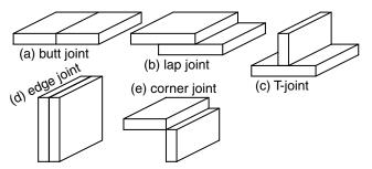
**Figure 1.4** Five basic types of weld joint designs.
