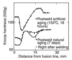
**Figure 15.14** HAZ hardness profiles in a 6061 aluminum gas—tungsten arc welded in T4 condition. From Kou and Le (11).
