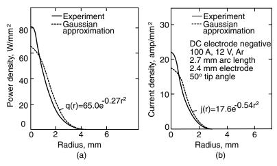
**Figure 4.8** Gas-tungsten welding arc: (*a*) power density distribution; (*b*) current density distribution. Reprinted from Lu and Kou (10). Courtesy of American Welding Society.
