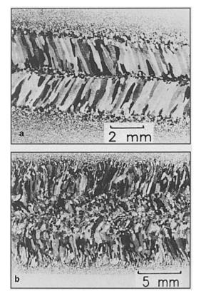
**Figure 7.27** Effect of electromagnetic pool stirring on grain structure in GTAW of 409 ferritic stainless steel: (a) without stirring; (b) with stirring. Reprinted from Villafuerte and Kerr (39). Courtesy of American Welding Society.
