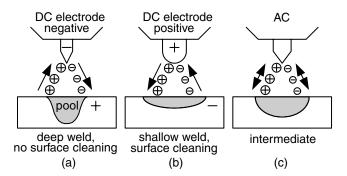
**Figure 1.12** Three different polarities in GTAW.
