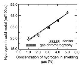
**Figure 3.12** Hydrogen content in gas-tungsten arc welds of 0.5Cr–0.5Mo steel as a function of volume percent of hydrogen in Ar–H<sub>2</sub> shielding gas. Reprinted from Albert et al. (23). Courtesy of American Welding Society.
