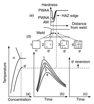
**Figure 15.8** Al-Cu alloy heat treated to contain  $\theta'$  before welding: (a) phase diagram; (b) thermal cycles; (c) reversion of  $\theta'$ ; (d) microstructure; (e) hardness distribution.  $\theta$  in base metal not shown.
