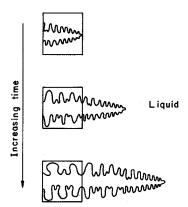
**Figure 6.18** Schematic showing dendritic growth of an alloy at a fixed position at various stages of solidification. Note that several smaller arms disappear while larger ones grow. Reprinted from Flemings (2).
