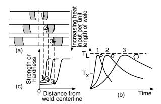
**Figure 14.11** Effect of heat input per unit length of weld on: (a) width of HAZ (shaded), (b) thermal cycles near fusion boundary, and (c) strength or hardness profiles.
