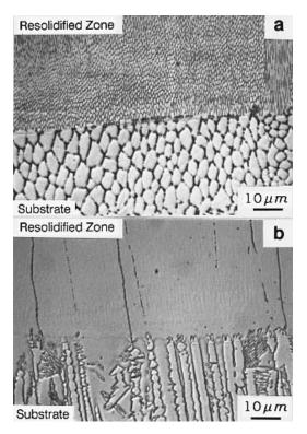
**Figure 9.17** Microstructure of the low-cooling-rate substrate  $(2 \times 10^3 \, ^{\circ}\text{C/s})$  and the high-cooling-rate electron beam weld at the top: (a) alloy 3 in Figure 9.15; (b) alloy 6. Reprinted from Elmer et al. (34).
