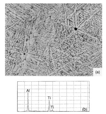
**Figure 7.15** Heterogeneous nuclei in GTAW of 6061 aluminum: (a) optical micrograph; (b) EDS analysis; (c) SEM image; (d) SEM image of  $TiB_2$  particles in a grain refiner for aluminum casting. (a, b) From Kou and Le (20). (d) Courtesy of Granger (21).
