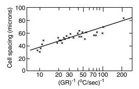
**Figure 6.19** Effect of *GR* on cell spacing in Sn–Pb alloys. Modified from Flemings (2) based on data from Plaskett and Winegard (28).
