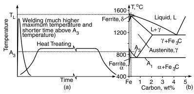
**Figure 17.2** Comparison between welding and heat treating of steel: (a) thermal processes; (b) Fe–C phase diagram.
