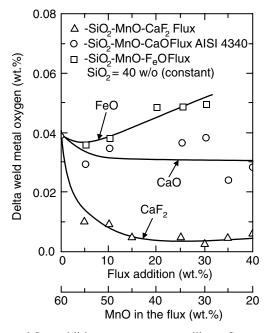
**Figure 3.18** Effect of flux additions to manganese silicate flux on extent of oxygen transfer to the weld metal in submerged arc welding of 4340 steel. Reprinted from Burck et al. (38). Courtesy of American Welding Society.
