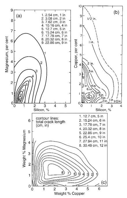
**Figure 11.26** Solidification cracking susceptibility of aluminum alloys: (*a*) Al–Mg–Si; (*b*) Al–Cu–Si (*c*) Al–Mg–Cu. (*a*, *b*) Modified from Jennings et al. (67). (*c*) Modified from Pumphrey and Moore (68).
