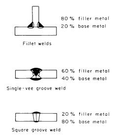
**Figure 11.25** Approximate dilution of three weld joints by base metal in aluminum welding. Reprinted from Dudas and Collins (40). Courtesy of American Welding Society.
