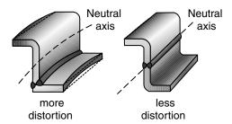
**Figure 5.10** Reducing distortion by placing welds around neutral axis. Modified from TWI (7).
