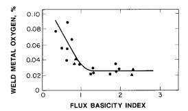
**Figure 3.21** Weld metal oxygen content in steel as a function of flux basicity in submerged arc welding. From Chai and Eagar (45).
