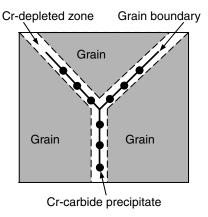
Figure 18.5 Grain boundary microstructure in sensitized austenitic stainless steel.
