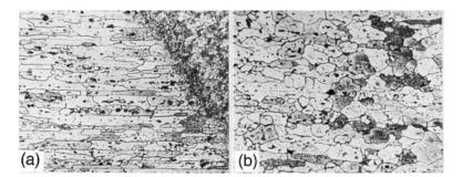
**Figure 14.13** Microstructure near fusion boundary of a work-hardened 2219-T37 aluminum: (a) electron beam weld; (b) gas-tungsten arc weld. Magnification 80×. Reprinted from *Metals Handbook* (12).
