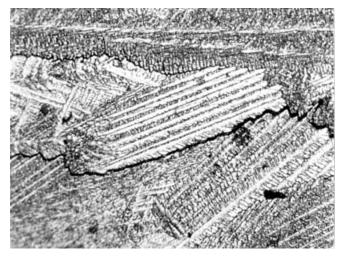
**Figure 11.2** Solidification cracking in an autogenous bead-on-plate weld of 7075 aluminum (magnification 140×). From Kou and Kanevsky (1).
