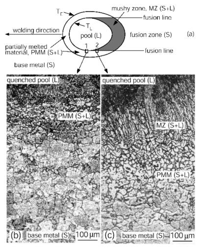
**Figure 7.11** Weld pool of 2219 aluminum quenched during GTAW: (a) overall view; (b) microstructure at position 1; (c) microstructure at position 2. Modified from Kou and Le (19). Courtesy of American Welding Society.
