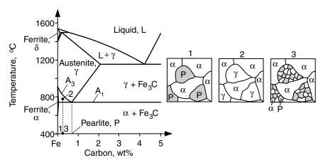
**Figure 17.4** Mechanism of partial grain refining in a carbon steel.
