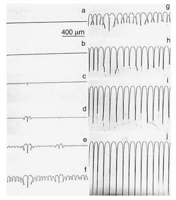
**Figure 6.12** Breakdown of a planar S/L interface during the solidification of pivalic acid–ethanol: (a) 0s, (b) 120s, (c) 210s, (d) 270s, (e) 294s, (f) 338s, (g) 378s, (h) 456s, (i) 576s, and (j) 656s. Reprinted from Liu and Kirkaldy (24). Copyright 1994 with permission from Elsevier Science.
