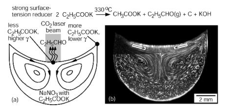
**Figure 4.18** Marangoni convection with an inward surface flow in a NaNO $_3$  pool containing 2 mol %  $C_2H_3COOK$  as a surface-active agent. Reprinted from Limmaneevitchitr and Kou (32). Courtesy of American Welding Society.
