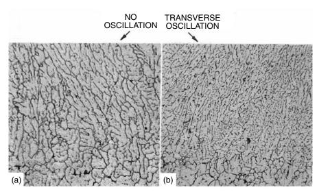
**Figure 8.15** Microstructures near fusion line of gas-tungsten arc welds of 2014 aluminum: (a) coarser dendrites in weld made without arc oscillation; (b) finer dendrites in weld made with transverse arc oscillation. Magnification 200×. Reprinted from Kou and Le (16). Courtesy of American Welding Society.
