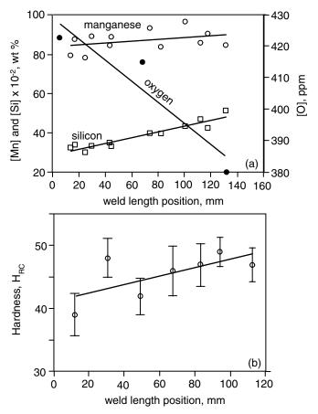
**Figure 3.10** Variations of weld metal along the length of a weld made with an E7018 electrode: (a) composition; (b) hardness. Reprinted from Bracarense and Liu (19). Courtesy of American Welding Society.
