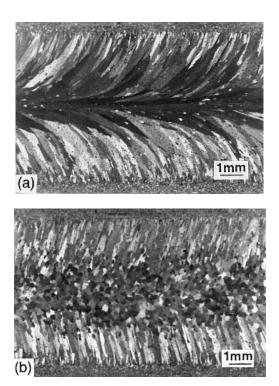
**Figure 7.19** Effect of welding parameters on grain structure in GTAW of 6061 aluminum: (a)  $70 \text{ A} \times 11 \text{ V}$  heat input and 5.1 mm/s welding speed; (b)  $120 \text{ A} \times 11 \text{ V}$  heat input and 12.7 mm/s welding speed. From Kou and Le (20).
