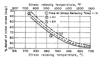
Figure 5.5 Effect of temperature and time on stress relief of steel welds. Reprinted from *Welding Handbook* (2). Courtesy of American Welding Society.
