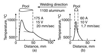
**Figure 7.20** Effect of welding parameters on temperature gradient at weld pool end of 1100 aluminum: (a) higher welding speed and heat input; (b) lower welding speed and heat input. From Kou and Le (27).
