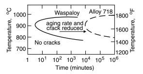
**Figure 16.13** Crack susceptibility C curves for Waspaloy and Inconel 718 welds. Reprinted, with permission, from Owczarski (l).
