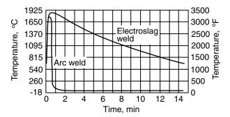
**Figure 2.24** Thermal cycles of electroslag and arc welds. Reprinted from Liu et al. (60).
