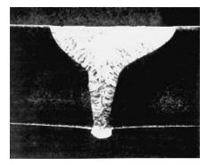
**Figure 1.16** A plasma arc weld made in 13-mm-thick 304 stainless steel with keyholing. From Lesnewich (8).
