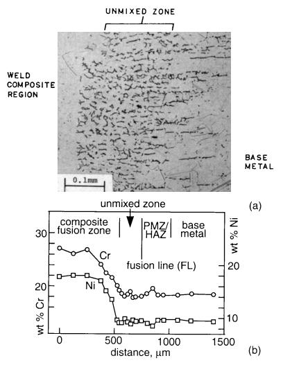
**Figure 10.12** Unmixed zone in a 304L stainless steel welded with a 310 filler metal: (a) microstructure; (b) composition profiles. Reprinted from Baeslack et al. (45). Courtesy of American Welding Society.
