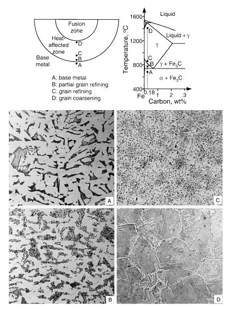
**Figure 17.3** HAZ microstructure of a gas-tungsten arc weld of 1018 steel (magnification 200×).
