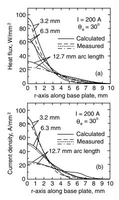
**Figure 4.9** Effect of arc length on gas—tungsten welding arcs: (a) power density distributions; (b) current density distributions. Modified from Lee and Na (6).
