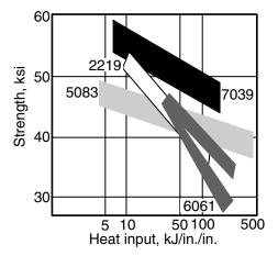
**Figure 1.2** Variation of weld strength with heat input per unit length of weld per unit thickness of workpiece. Reprinted from Mendez and Eagar (2).
