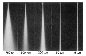
**Figure 1.26** Dispersion of electron beam at various ambient pressures (1). Reprinted from *Welding Handbook* (1). Courtesy of American Welding Society.
