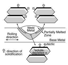
Figure 12.12 Directional solidification of GB liquid in PMZ.
