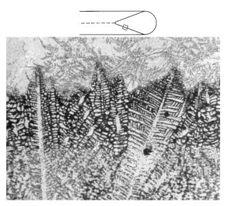
**Figure 9.5** Liquid-tin quenched solidification structure near the pool of an autogenous gas-tungsten arc weld of 309 stainless steel. Magnification 70×. Mixed-chloride etchant. Reprinted from Kou and Le (9).
