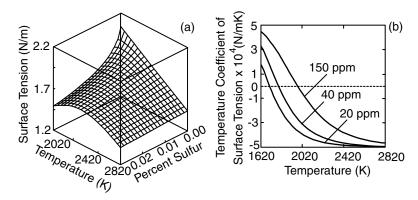
**Figure 4.20** Liquid iron with various levels of sulfur: (a) surface tension; (b) temperature coefficient of surface tension. Reprinted from Pitscheneder et al. (36). Courtesy of American Welding Society.
