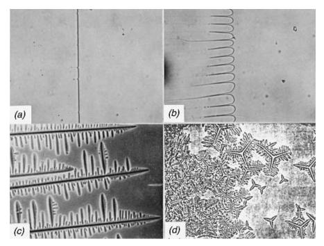
**Figure 6.8** Basic solidification modes (magnification  $67\times$ ): (a) planar solidification of carbon tetrabromide (5); (b) cellular solidification of carbon tetrabromide with a small amount of impurity (5); (c) columnar dendritic solidification of carbon tetrabromide with several percent impurity (5); (d) equiaxed dendritic solidification of cyclohexanol with impurity (6). From *Solidification* (5), pp. 132–134, with permission.
