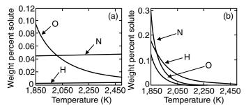
**Figure 3.3** Equilibrium concentration of nitrogen, oxygen, and hydrogen in liquid iron as a function of temperature: (a)  $N_2(g)$  with  $p_{N_2} = 1$  atm,  $O_2(g)$  with  $p_{O_2} = 10^{-9}$  atm,  $H_2(g)$  with  $p_{H_2} = 1$  atm; (b) N(g) with  $p_N = 10^{-6}$  atm, O(g) with  $p_O = 10^{-8}$  atm, O(g) with O(g) w
