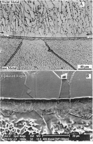
**Figure 7.6** Fusion boundary microstructure in 409 ferritic stainless steel (bcc) welded with Monel filler wire (fcc): (a) optical micrograph; (b) scanning electron micrograph. White arrows: fusion boundary; dark arrows: new grains nucleated along fusion boundary. Reprinted from Nelson et al. (11). Courtesy of American Welding Society.
