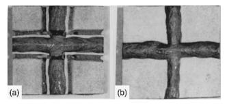
**Figure 18.12** Welds in austenitic stainless steels: (a) weld decay in 304 stainless steel; (b) no weld decay in 321 stainless steel. From Linnert (16).
