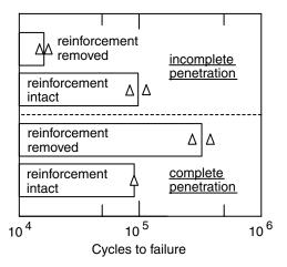
**Figure 5.22** Effect of weld reinforcement and penetration on fatigue life of transverse butt welds of 5456 aluminum. Reprinted from Nordmark et al. (20). Courtesy of American Welding Society.
