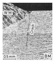
**Figure 5.18** Fatigue crack originating from weld toe of gas-metal arc weld of carbon steel. Reprinted from Itoh (15). Courtesy of American Welding Society.
