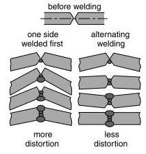
**Figure 5.9** Reducing angular distortion by using double-V joint and welding alternately on either side of joint. Modified from TWI (7).
