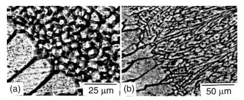
**Figure 7.31** Effect of gravity on grain structure in GTAW of 2090 Al–Li–Cu alloy: (a) 1g; (b) 10g and with equiaxed zone (EQZ) near the fusion boundary eliminated. Reprinted from Aidun and Dean (48). Courtesy of American Welding Society.
