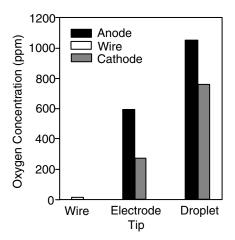
**Figure 3.27** Oxygen contents of the welding wire, melted electrode tips, and detached droplets for both electrode-positive and electrode-negative polarities. Reprinted from Kim et al. (58). Courtesy of American Welding Society.
