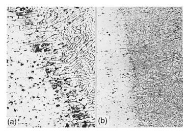
**Figure 8.12** Autogenous welds of 6061 aluminum: (a) coarser solidification structure in gas—tungsten arc weld: (b) finer solidification structure in electron beam weld. Reprinted from *Metals Handbook* (10).
