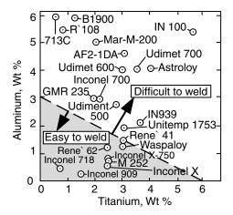
**Figure 16.12** Effect of Al and Ti contents on postweld heat treatment cracking. Modified from Kelly (30).
