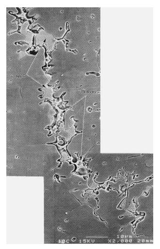
**Figure 11.17** Scanning electron micrographs showing morphology of  $\gamma$ NbC and  $\gamma$  Laves constituents in solidification cracks of a Nb-bearing superalloy. Reprinted from DuPont et al. (34).
