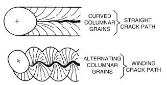
**Figure 11.32** Schematic sketches showing effect of arc oscillation on solidification cracking. From Kou and Le (87).
