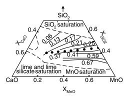
**Figure 3.20** Activity of MnO in CaO–MnO–SiO<sub>2</sub> melts at 1500°C. Reprinted from Burck et al. (38). Courtesy of American Welding Society.
