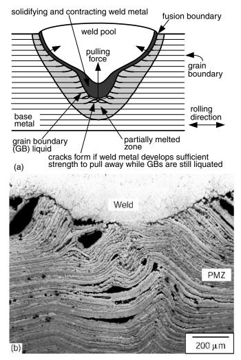
**Figure 13.7** Weld metal pulling and tearing PMZ: (a) schematic sketch; (b) 7075 aluminum welded with filler 1100. From Huang and Kou (13).
