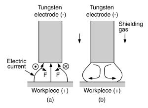
**Figure 4.5** Arc produced by a tungsten electrode with a flat end: (a) Lorentz force (F); (b) fluid flow.
