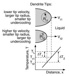
Figure 10.4 Dendrite tip undercooling.
