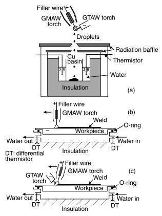
**Figure 2.5** Calorimeter for measuring heat inputs in GMAW: (a) metal droplets; (b) total heat input; (c) combined heat inputs from arc and metal droplets. Reprinted from Lu and Kou (10, 11). Courtesy of American Welding Society.
