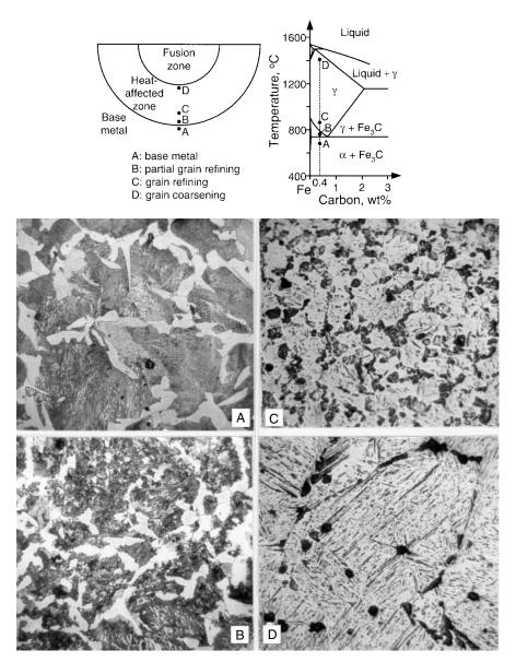
**Figure 17.9** HAZ microstructure of a gas-tungsten arc weld of 1040 steel (magnification 400×).
