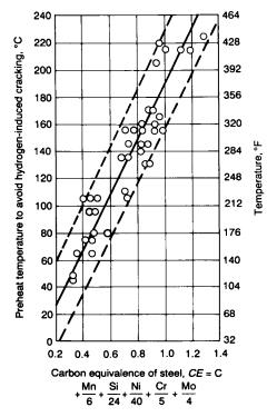
**Figure 17.24** Effect of carbon equivalent on preheat requirement to prevent hydrogen cracking. Reprinted from Lesnewich (34).
