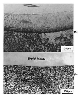
**Figure 10.14** Carbon steel side of weld metal in a weld between a carbon steel and an austenitic stainless steel made with a Ni-based filler metal: (a) martensite along fusion boundary; (b) martensite avoided by preheating and controlling interpass temperature. Reprinted from Omar (43). Courtesy of American Welding Society.
