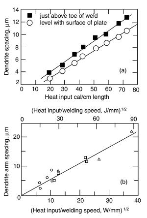
**Figure 8.14** Effect of heat input per unit length of weld on dendrite arm spacing. (a) For Al–Mg–Mn alloy. From Jordan and Coleman (13). (b) For 2014 Al–Cu alloy. Modified from Lanzafame and Kattamis (14). Courtesy of American Welding Society.
