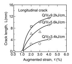
**Figure 13.13** Effect of heat input on liquation cracking in Varestraint testing of 6061 aluminum welded with 5356 filler metal. Modified from Miyazaki et al. (12). Courtesy of American Welding Society.
