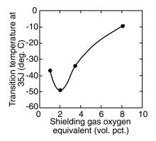
**Figure 9.30** Weld metal Charpy V-notch toughness expressed as transition temperature as a function of shielding gas oxygen equivalent. Reprinted from Onsoien et al. (45). Courtesy of American Welding Society.
