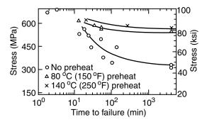
**Figure 17.23** Effect of preheating on hydrogen cracking of a high-strength steel. Reprinted from Gedeon and Eagar (26). Courtesy of American Welding Society.
