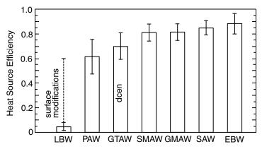
Figure 2.7 Heat source efficiencies in several welding processes.
