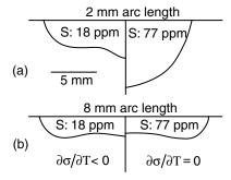
**Figure 4.23** Stationary GTA welds in 304 stainless steels with 18 ppm sulfur and 77 ppm sulfur made with an arc length of (a) 2 mm and (b) 8 mm. Modified from Matsunawa et al. (39).
