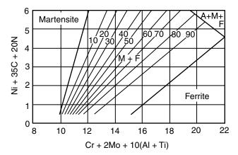
**Figure 9.13** Ferritic–martensitic stainless steel constitution diagram containing a boundary for austenite formation and with iso-ferrite lines in volume percent of ferrite. Reprinted from Balmforth and Lippold (23).
