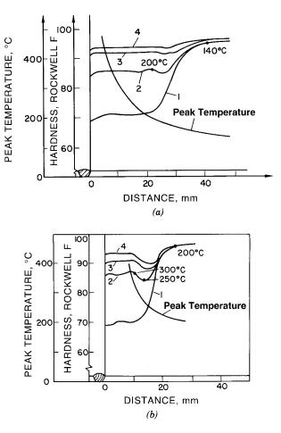
**Figure 15.19** HAZ hardness profiles in Al–4.5Zn–1.2Mg alloy: (*a*) naturally aged before welding (1:3 hour, 2:4 days, 3:30 days, 4:90 days); (*b*) artificially aged at 130°C for 1 h before welding. From Mizuno (23).
