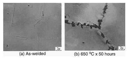
**Figure 18.15** Transmission electron micrographs near fusion boundary of 347 stainless steel. From Ikawa et al. (18).
