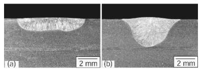
**Figure 4.15** YAG laser welds in two 304 stainless steels with (a) 40 ppm sulfur and (b) 140 ppm sulfur. From Limmaneevichitr and Kou (27).
