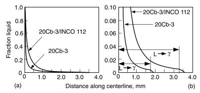
**Figure 11.16** Fraction liquid as a function of distance within the mushy zone of 20Cb-3 and 20Cb-3–INCO 112 composite (a) and enlarged (b). Reprinted from DuPont (35). Courtesy of American Welding Society.
