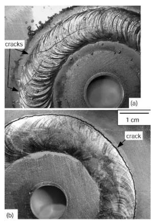
**Figure 13.3** Cracking in circular-patch welds: (a) 6061 aluminum made with a 1100 filler wire; (b) 2219 aluminum (outside) welded to 1100 aluminum (inside) with a 1100 filler wire. From Huang and Kou (13).
