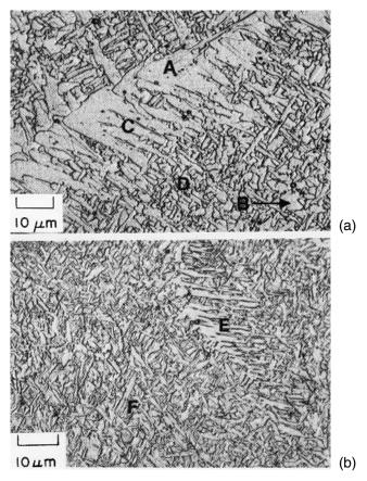
**Figure 9.22** Micrographs showing typical weld metal microstructures in low-carbon steels: A, grain boundary ferrite; B, polygonal ferrite; C, Widmanstatten ferrite; D, acicular ferrite; E, upper bainite; F, lower bainite. Reprinted from Grong and Matlock (46).
