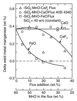
**Figure 3.19** Effect of flux additions to manganese silicate flux on extent of manganese transfer to the weld metal in submerged arc welding of 4340 steel. Reprinted from Burck et al. (38). Courtesy of American Welding Society.
