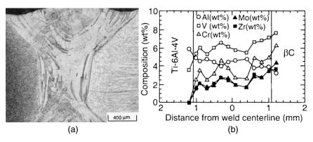
**Figure 10.15** Macrosegregation in a laser beam weld between Ti–6Al–4V and Ti–3Al–8V–6Cr–4Mo–4Zr (βC): (*a*) transverse cross section; (*b*) composition profiles. Reprinted from Liu et al. (53). Courtesy of American Welding Society.
