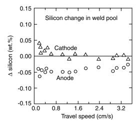
**Figure 3.28** Gain or loss of weld metal silicon due to reactions in weld pool for electrode-positive and electrode-negative polarities as a function of welding speed. Reprinted from Kim et al. (58). Courtesy of American Welding Society.
