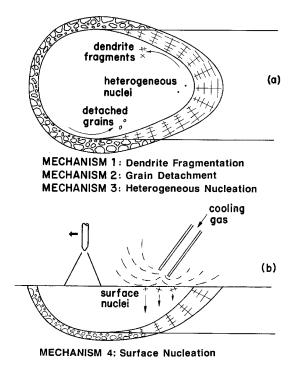
**Figure 7.13** Nucleation mechanisms during welding: (a) top view; (b) side view. Reprinted from Kou and Le (19). Courtesy of American Welding Society.
