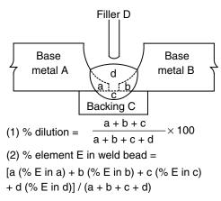
**Figure 10.17** Filler metal dilution and composition in dissimilar-metal welding. Reprinted from Estes and Turner (55). Courtesy of American Welding Society.
