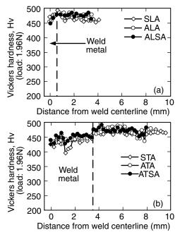
**Figure 16.9** Hardness profiles in Inconel 718 welds after postweld heat treating: (a) laser welds; (b) gas—tungsten arc welds. S: solutionized; A: aged after solutionization; L: laser welded; T: gas—tungsten arc welded. Broken line indicates fusion line. From Hirose et al. (15).
