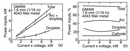
**Figure 2.6** Power inputs during GMAW of aluminum: (a) measured results; (b) breakdown of total power input. Reprinted from Lu and Kou (10). Courtesy of American Welding Society.
