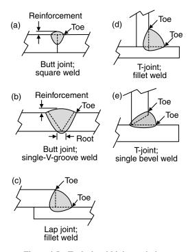
**Figure 1.5** Typical weld joint variations.
