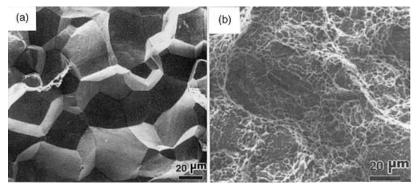
**Figure 17.28** SEM micrographs of fracture surfaces of a 2.4Cr–1.5W–0.2V ferritic steel: (a) single-pass sample; (b) multiple-pass sample. Reprinted from Nawrocki et al. (36, 45). Courtesy of American Welding Society.
