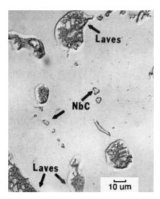
**Figure 12.7** PMZ of Inconel 718 weld showing constitutional liquation due to Laves eutectic reaction. Reprinted from Kelly (13).
