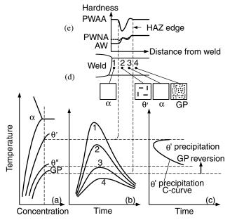
**Figure 15.13** Al–Cu alloy heat treated to contain GP zones before welding: (a) phase diagram; (b) thermal cycles; (c) precipitation C curves; (d) microstructure; (e) hardness distribution.  $\theta$  in base metal not shown.
