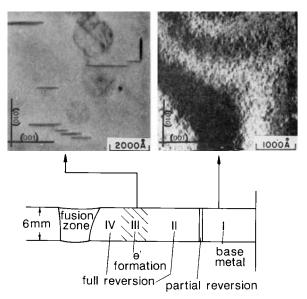
**Figure 15.11** Transmission electron micrographs of a 2219 aluminum aged to contain GP zones before welding. From Dumolt et al. (5).
