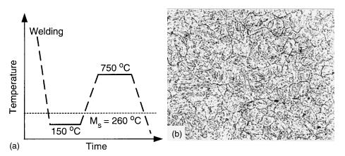
**Figure 18.25** Proper postweld heat treatment and resultant microstructure of a 12% Cr martensitic steel (magnification 500×). Reprinted, with permission, from Castro and De Cadenet (4). Copyright 1974 Cambridge University Press.
