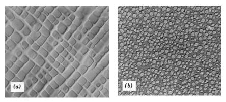
**Figure 16.2**  $\gamma'$  in Ni-base alloys: (a) cubical  $\gamma'$  in IN-100 (magnification 13,625×); (b) spherical and cooling  $\gamma'$  in U500 (magnification 5450×). From Decker and Sims (6).
