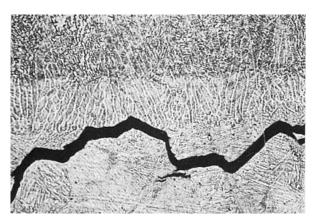
**Figure 13.9** Hydrogen-induced cracking in the PMZ of HY-80 steel. Reprinted from Savage et al. (22). Courtesy of American Welding Society.
