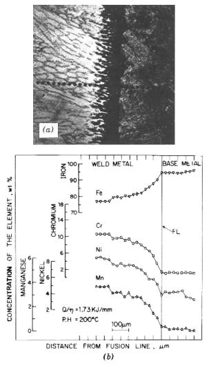
**Figure 10.11** Fusion boundary of a low-alloy steel welded with an austenitic stainless steel electrode: (a) microstructure (magnification  $55\times$ ); (b) segregation. Reprinted from Ornath et al. (46). Courtesy of American Welding Society.
