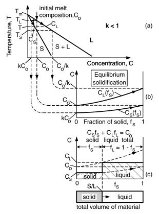
**Figure 6.3** Solute redistribution during solidification with complete diffusion in solid and liquid: (a) phase diagram; (b)  $C_L(f_s)$  and  $C_S(f_s)$ ; (c) composition profiles in solid and liquid.
