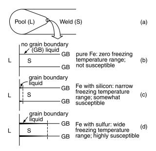
**Figure 11.9** Effect of impurities on grain boundary liquid of weld metal: (a) weld metal near pool; (b) no liquid in pure Fe; (c) some liquid with a small amount of Si; (d) much more liquid with a small amount of sulfur.
