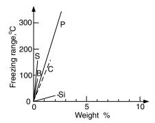
**Figure 11.8** Effect of alloying elements on the solidification temperature range of carbon and low-alloy steels. Modified from *Principles and Technology of the Fusion Welding of Metals* (30).
