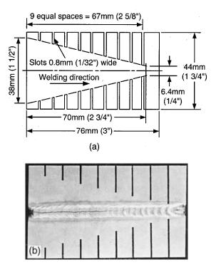
**Figure 11.4** Houldcroft test: (a) design (11); (b) cracking in an aluminum alloy specimen. Reprinted from Liptax and Baysinger (12). Courtesy of American Welding Society.
