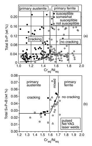
**Figure 11.19** Solidification crack susceptibility of austenitic stainless steels: (a) arc welds; (b) laser welds. (a) From Takalo et al. (44). (b) Reprinted from Lienert (45).
