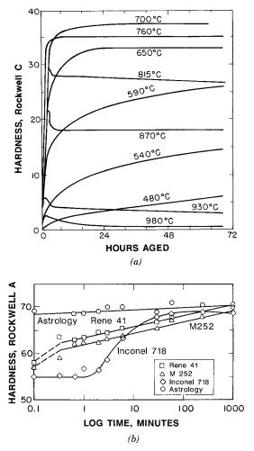
**Figure 16.4** Aging characteristics of Ni-base alloys. (a) Inconel X-750. From Eiselstein (11). (b) Some other Ni-base alloys. Reprinted from Wilson and Burchfield (12). Courtesy of American Welding Society.
