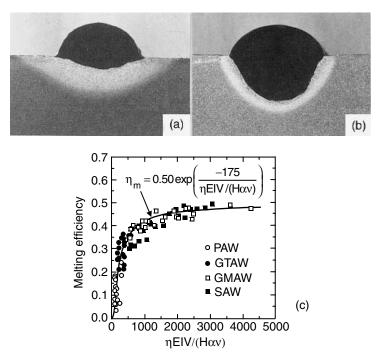
**Figure 2.9** Melting efficiency: (a) lower at lower heat input and welding speed; (b) higher at higher heat input and welding speed; (c) variation with dimensionless parameter  $\eta EIV/H\alpha\nu$ . Reprinted from DuPont and Marder (7). Courtesy of American Welding Society.
