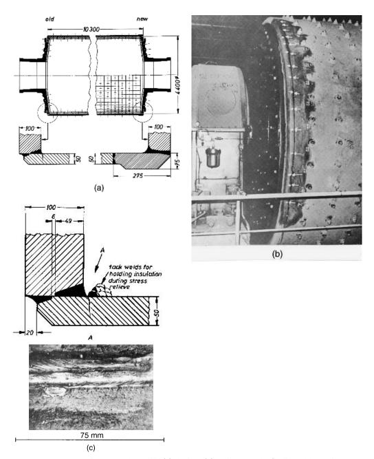
**Figure 5.24** Failure of a ball mill: (a) design; (b) fatigue cracks (indicated by white arrows); (c) origin of fatigue cracks. From Wallner (22).
