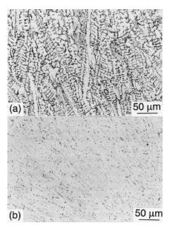
**Figure 9.20** Effect of thermal cycles on ferrite content in 316 stainless steel weld: (a) as welded; (b) subjected to thermal cycle of  $1250^{\circ}$ C peak temperature three times after welding. Reprinted from Chen and Chou (40).
