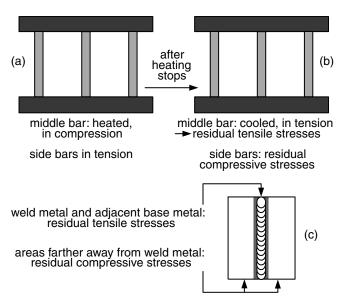
**Figure 5.1** Thermally induced stresses: (a) during heating; (b) during cooling; (c) residual stresses in weld.
