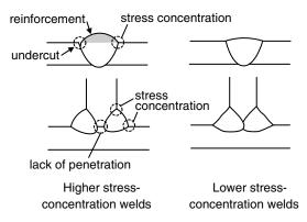
Figure 5.21 Stress raisers in butt and T-welds and their corrections.
