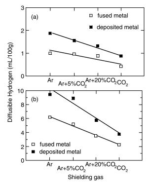
**Figure 3.14** Effect of shielding gases on weld metal hydrogen content: (a) GMAW; (b) FCAW. Reprinted from Mirza and Gee (22).
