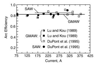
**Figure 2.4** Arc efficiencies in GMAW and SAW.
