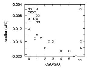
**Figure 3.23** Desulfurization of high-strength, low-alloy steel welds as a function of basicity index CaO/SiO<sub>2</sub> of CaF<sub>2</sub>–CaO–SiO<sub>2</sub> type flux. Reprinted from Dallam et al. (47). Courtesy of American Welding Society.
