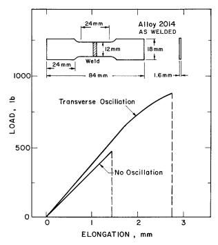
**Figure 8.16** Tensile testing of two gas–tungsten arc welds of 2014 aluminum made without arc oscillation and with transverse arc oscillation. From Kou and Le (16).
