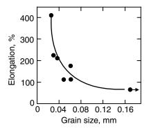
**Figure 7.23** Effect of grain size on weld metal ductility of a Cr–Ni iron base alloy at 925°C. Modified from Petersen (31).
