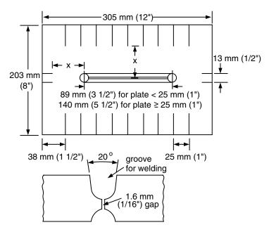
**Figure 17.22** Lehigh restraint specimen. Reprinted from Stout et al. (30). Courtesy of American Welding Society.
