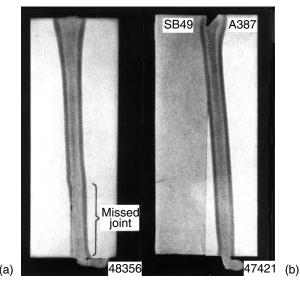
**Figure 1.28** Missed joints in electron beam welds in 150-mm-thick steels: (a) 2.25Cr–1Mo steel with a transverse flux density of 3.5 G parallel to joint plane; (b) SB (C–Mn) steel and A387 (2.25Cr–1Mo) steel. Reprinted from Blakeley and Sanderson (17). Courtesy of American Welding Society.
