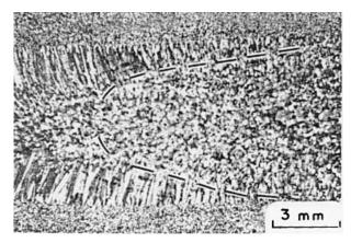
**Figure 7.26** Widening of equiaxed zone in GTAW of alloy Al–2.5Mg–0.011Ti by magnetic stirring (at dotted line). Reprinted from Pearce and Kerr (32).
