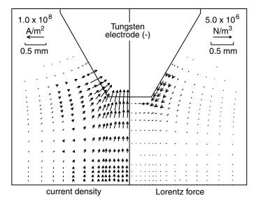
**Figure 4.3** Current density field (left) and Lorentz force field (right) in an arc produced by a tungsten electrode with a  $60^{\circ}$  tip angle. Modified from Tsai and Kou (1).
