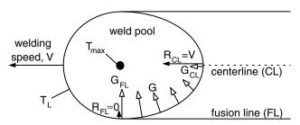
**Figure 8.4** Variations in temperature gradient G and growth rate R along pool boundary.
