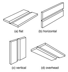
Figure 1.6 Four welding positions.
