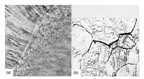
**Figure 17.25** Reheat cracking in a CrMoV steel: (a) macrostructure (magnification  $\times 35$ ); (b) microstructure (magnification  $\times 1000$ ). The cracks are along the prior austenite grain boundaries of the bainitic structure. From Bailey (27).
