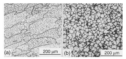
**Figure 7.24** Effect of inoculation on grain structure in GTAW of 2090 Al–Li–Cu alloy: (a) 2319 Al–Cu filler metal; (b) 2319 Al–Cu filler metal inoculated with 0.38% Ti. Reprinted from Sundaresan et al. (35).
