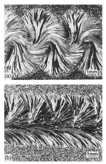
**Figure 7.30** Grain structures in oscillated arc welds of aluminum alloys. (a) For alloy 2014 with transverse arc oscillation. From Kou and Le (14). (b) For alloy 5052 with circular arc oscillation. From Kou and Le (15).
