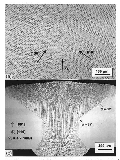
**Figure 8.9** Electron beam weld of single crystal of pure Fe–15Cr–15Ni made in a [110] direction on a (001) surface: (a) top cross section; (b) transverse cross section. Reprinted from Rappaz et al. (5).
