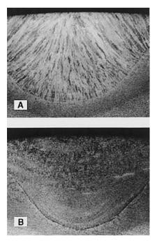
**Figure 7.22** Effect of inoculation on grain structure in submerged arc welds of C–Mn steel (magnification 6×): (a) without inoculation; (b) inoculation with titanium. Reprinted from Heintze and McPherson (30). Courtesy of American Welding Society.
