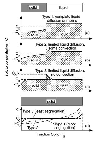
**Figure 6.7** Solute redistributions in the absence of solid diffusion: (a) type 1; (b) type 2; (c) type 3; (d) resultant segregation profiles.
