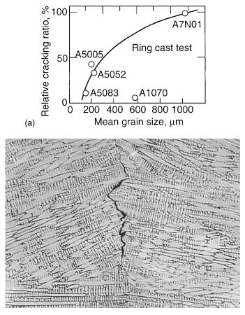
**Figure 11.23** Effect of grain structure on solidification cracking: (a) aluminum alloys; (b) centerline cracking in a coarse-grain 310 stainless steel weld. (a) From Nakata and Matsuda (16). (b) From Kou and Le (65).
