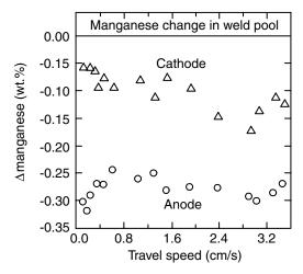
**Figure 3.29** Loss of weld metal manganese due to reactions in weld pool for electrode-positive and electrode-negative polarities as a function of welding speed. Reprinted from Kim et al. (58). Courtesy of American Welding Society.
