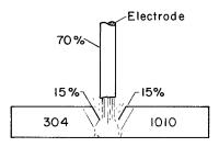
Figure 11.30 Welding 304 stainless steel to 1010 carbon steel.
