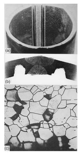
**Figure 18.27** Failure of a 304 stainless steel pipe (10 cm diameter): (a) section from failed pipe; (b) transverse cross section of seam weld; (c) microstructure of weld decay area. Reprinted from *Welding Handbook* (24). Courtesy of American Welding Society.
