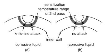
**Figure 18.17** Dual-pass weld of stabilized austenitic stainless steel: (a) knife-line attack; (b) no attack. Modified from *Principle and Technology of the Fusion Welding of Metals* (8).
