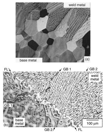
**Figure 7.4** Epitaxial growth. (a) Near the fusion boundary of electron beam weld of C103 alloy (magnification  $400\times$ ). Reprinted from O'Brien (9). Courtesy of American Welding Society. (b) Near the fusion boundary of as-cast Al-4.5Cu welded with 4043 filler (Al-5Si).
