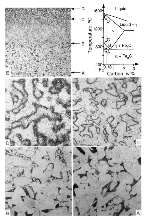
**Figure 17.6** HAZ microstructure of 1018 steel produced by a high-power  $CO_2$  laser. Magnification of (A)–(D) 415× and of (E) 65×. From Kou et al. (11).
