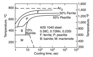
Figure 17.10 Continuous cooling transformation diagram for 1040 steel. Modified from *Atlas of Isothermal Transformation and Cooling Transformation Diagrams* (13).
