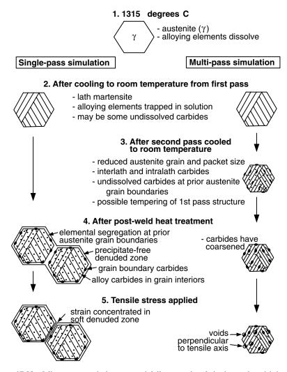
**Figure 17.29** Microstructural changes and failure mode of single- and multiple-pass samples of a 2.4Cr–1.5W–0.2V ferritic steel. Modified from Nawrocki et al. (45). Courtesy of American Welding Society.
