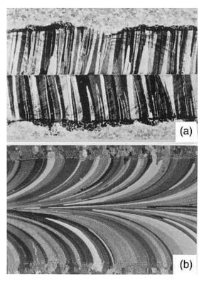
**Figure 7.9** Gas-tungsten arc welds of 99.96% aluminum: (a) 1000 mm/min welding speed; (b) 250 mm/min welding speed. From Arata et al. (13).
