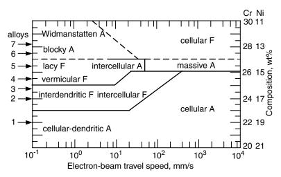
**Figure 9.16** Electron beam travel speed (cooling rate) versus composition map of microstructural morphologies of the seven alloys in Figure 9.15 (A and F denote austenite and ferrite, respectively). The solid lines indicate the regions of the four primary solidification modes, while the dashed lines represent the different morphologies resulting from postsolidification transformation from ferrite to austenite. Modified from Elmer et al. (33).
