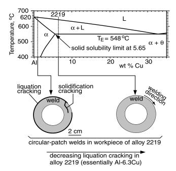
**Figure 13.6** Effect of weld metal composition on PMZ cracking in 2219 aluminum. From Huang and Kou (13).
