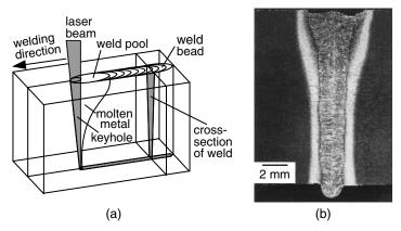
**Figure 1.30** Laser beam welding with  $CO_2$  laser: (a) process; (b) weld in 13-mm-thick A633 steel. (b) Courtesy of E.A. Metzbower.
