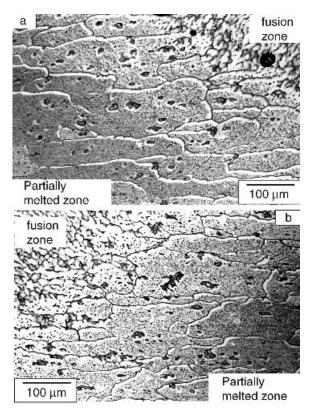
**Figure 12.2** PMZ microstructure of gas—metal arc weld in 2219 aluminum made with 2319 aluminum filler wire: (a) left of weld; (b) right of weld. Reprinted from Huang and Kou (1). Courtesy of American Welding Society.
