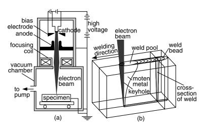
**Figure 1.25** Electron beam welding: (a) process; (b) keyhole. Modified from Arata (15).
