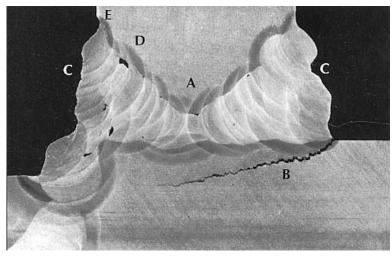
**Figure 10.8** Multipass weld with slag inclusions (D) and other defects, including lack of fusion (A), lamellar tearing (B), poor profile (C), and undercut (E). Reprinted from Lochhead and Rodgers (33). Courtesy of American Welding Society.
