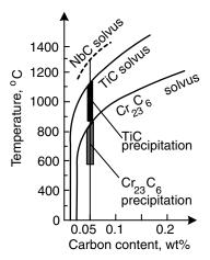
**Figure 18.7** Solvus curves for Cr<sub>23</sub>C<sub>6</sub> and TiC in 304 stainless steel. Modified from *Principle and Technology of the Fusion Welding of Metals* (8).
