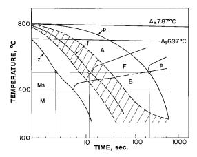
**Figure 17.12** CCT curves for A514 steel. From Inagaki et al. (18).
