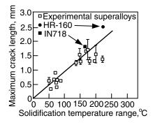
**Figure 11.11** Maximum crack length as a function of solidification temperature range for Nb-bearing superalloys and two other materials. Reprinted from DuPont et al. (18). Courtesy of American Welding Society.
