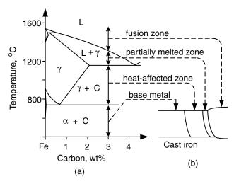
Figure 12.17 PMZ in a cast iron.
