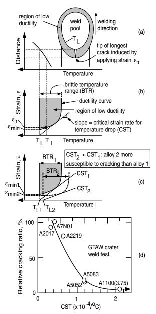
**Figure 11.18** Ductility of solidifying weld metal: (a) temperature distribution (temperature increases from right to left); (b) ductility curve; (c) ductility curves with different crack susceptibility; (d) effect of CST on cracking. (d) From Nakata and Matsuda (16).
