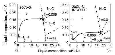
**Figure 11.12** Solidification paths (solid lines) of Nb-stabilized austenitic stainless steels: (*a*) 20Cb-3; (*b*) 20Cb-3–INCO 112 composite. Reprinted from DuPont (35). Courtesy of American Welding Society.
