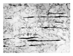
**Figure 17.31** Microstructure of a lamellar-tearing susceptible steel. From Dickinson and Nichols (51).
