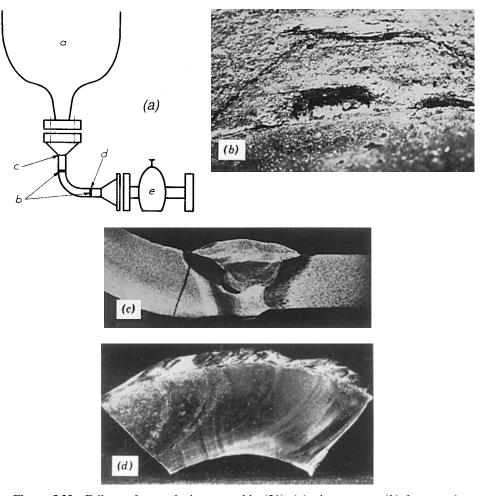
**Figure 5.23** Failure of a steel pipe assembly (21): (a) pipe system; (b) fracture A caused by craters at position c; (c) fracture B at weld at position d; (d) surface of fracture B.
