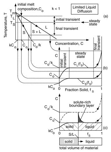
**Figure 6.5** Solute redistribution during solidification with limited diffusion in liquid and no diffusion in solid: (a) phase diagram; (b)  $C_L(f_s)$  and  $C_S(f_s)$ ; (c) composition profiles in solid and liquid.
