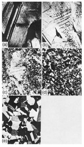
**Figure 14.2** Deformation and recrystallization structures of  $\alpha$ -brass: (a) 33% cold reduction; (b) short anneal at 580°C; (c) longer anneal; (d) completely recrystallized; (e) grain growth. From Burke (3).
