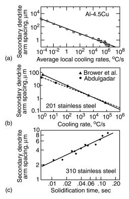
**Figure 6.17** Effect of cooling rate or solidification time on dendrite arm spacing: (a) For Al–4.5Cu. From Munitz (25), (b) For 201 stainless steel. From Paul and DebRoy (26). (c) For 310 stainless steel. From Kou and Le (27).
