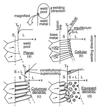
**Figure 8.1** Effect of constitutional supercooling on solidification mode during welding: (a) planar; (b) cellular; (c) columnar dendritic; (d) equiaxed dendritic. Constitutional supercooling increases from (a) through (d).
