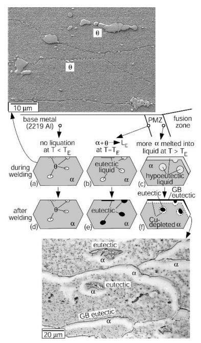
**Figure 12.5** Microstructure evolution in PMZ of 2219 aluminum with SEM image of the base metal on the top and optical micrograph of the PMZ at the bottom. Reprinted from Huang and Kou (1). Courtesy of American Welding Society.
