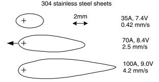
**Figure 2.21** Weld pool shapes in GTAW of 304 stainless steel sheets. Courtesy of Smolik (56).
