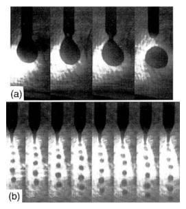
**Figure 1.19** Metal transfer during GMAW of steel with Ar–2%  $O_2$  shielding: (a) globular transfer at 180 A and 29 V shown at every  $3 \times 10^{-3}$  s; (b) spray transfer at 320 A and 29 V shown at every  $2.5 \times 10^{-4}$  s. Reprinted from Jones et al. (11). Courtesy of American Welding Society.
