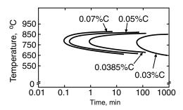
**Figure 18.10** Effect of carbon content on isothermal precipitation of Cr<sub>23</sub>C<sub>6</sub> in 304 stainless steel. From Ikawa et al. (14).
