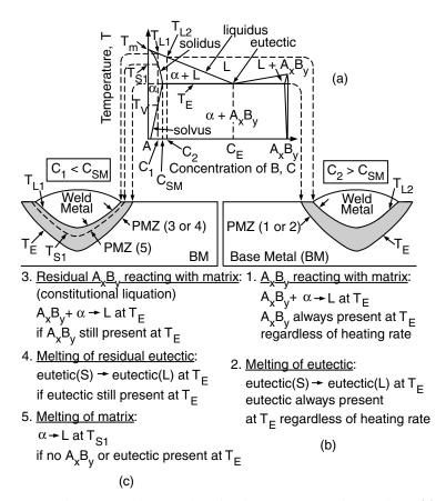
**Figure 12.4** Five mechanisms for liquation in PMZ of aluminum alloys: (a) phase diagram; (b) two mechanisms for an alloy beyond the solid solubility limit  $(C_{SM})$ ; (c) three mechanisms for an alloy within the solid solubility limit.
