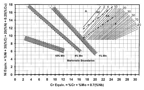
**Figure 9.12** WRC-1992 diagram with martensite boundaries for 1, 4, and 10% Mn. Reprinted from Kotecki (20). Courtesy of American Welding Society.
