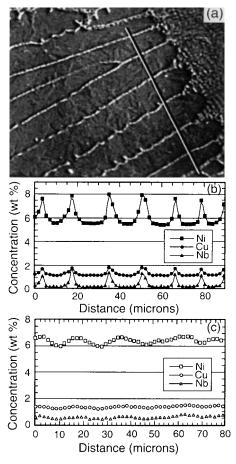
**Figure 10.1** Microsegregation across columnar dendrites near quenched weld pool in a martensitic stainless steel: (a, b) near growth front; (c) 400  $\mu$ m behind. Reprinted from Brooks and Garrison (8). Courtesy of American Welding Society.
