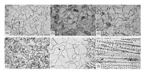
**Figure 14.6** Microstructure across the weld of a work-hardened 304 stainless steel: (a) before work hardening; (b) base metal; (c) carbide precipitation at grain boundaries; (d) recrystallization; (e) grain growth next to fusion boundary; (f) fusion zone. Magnification 137×. Reprinted from  $Metals\ Handbook\ (8)$ .
