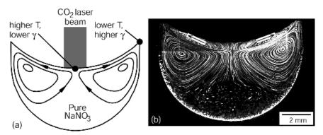
**Figure 4.17** Marangoni convection with an outward surface flow in a NaNO<sub>3</sub> pool. Reprinted from Limmaneevichitr and Kou (28). Courtesy of American Welding Society.
