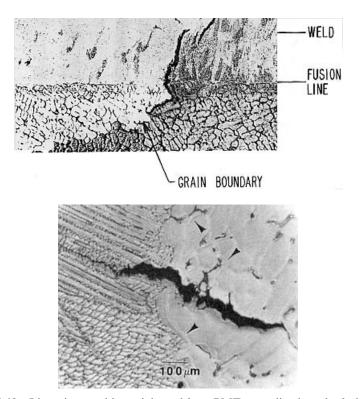
**Figure 13.19** Liquation cracking originated from PMZ extending into the fusion zone. (a) Cast 304 stainless steel. Reprinted from Apblett (35). Courtesy of American Welding Society. (b) Cast corrosion-resistant austenitic stainless steel. Reprinted from Cieslak (36).
