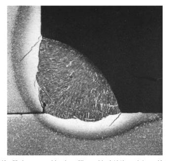
**Figure 17.19** Hydrogen cracking in a fillet weld of 1040 steel (magnification 4.5×). Courtesy of Buehler U.K., Ltd., Coventry, United Kingdom.
