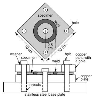
Figure 13.2 Schematic sketch of a circular-patch test.
