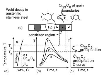
**Figure 18.8** Sensitization in austenitic stainless steel: (a) phase diagram; (b) thermal cycle; (c) precipitation curve; (d) microstructure.
