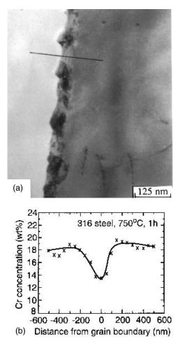
**Figure 18.4** Chromium carbide precipitation at a grain boundary in 316 stainless steel: (a) TEM micrograph; (b) Cr concentration profile across grain boundary. From Magula et al. (6).
