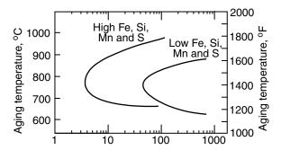
**Figure 16.17** Effect of composition on postweld heat treatment cracking of Rene 41. Reprinted from Berry and Hughes (36). Courtesy of American Welding Society.
