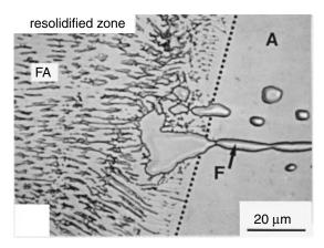
**Figure 7.5** Epitaxial growth of austenite (A) and ferrite (F) from the fusion line of an austenitic stainless steel containing both phases. From Elmer et al. (10).
