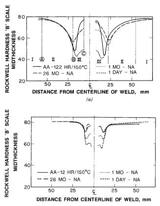
**Figure 15.21** HAZ hardness profiles in 3-cm-thick artificially aged 7039 aluminum: (a) 4 passes, continuous welding; (b) 16 passes,  $150^{\circ}$ C interpass temperature. Reprinted from Kelsey (24). Courtesy of American Welding Society.
