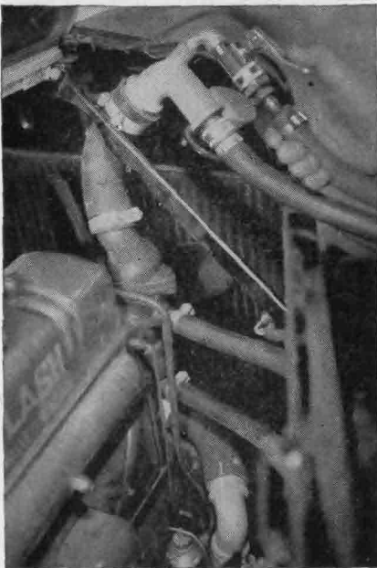
FIG. 14-9. Reverse flushing of radiator. (Kent-Moore Organization, Inc.)
