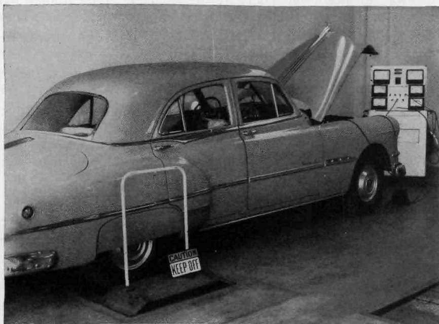
FIG. 8-6. Automobile in place on chassis dynamometer. Rear wheels drive the dynamometer rollers, and instruments on test panel indicate car speed, engine power output, engine speed, engine intake-manifold vacuum, air-fuel ratio, etc. (Clayton Manufacturing Company)
