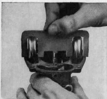
FIG. 10-8. Checking float-height adjustment. (Chevrolet Motor Division of General Motors Corporation)
