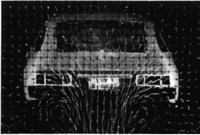
Fig.16.2 Wake behind an automobile (tuft grid method) in water, flow velocity 1 m/s, length 530 mm (scale 1: 8), Re = 5 \times 10^5
