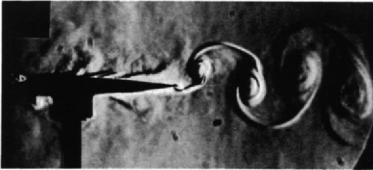
Fig.16.12 Flow at bottom dead point of vertically vibrating wing (Schlieren method) in air, flow velocity 5 m/s, chord length 100 mm, Re = 3 \times 10^4 , vibration frequency 90 Hz, single amplitude 4 mm
