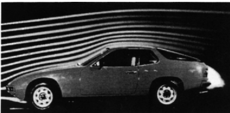
Fig.16.6 Flow around an automobile (smoke method)
