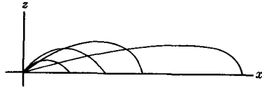
FIG. 3-29. Trajectories for maximum range for projectiles with various muzzle velocities.
