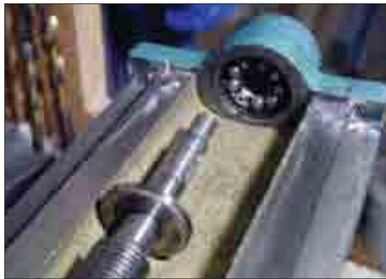
Lead screw supported by collar bearing.
