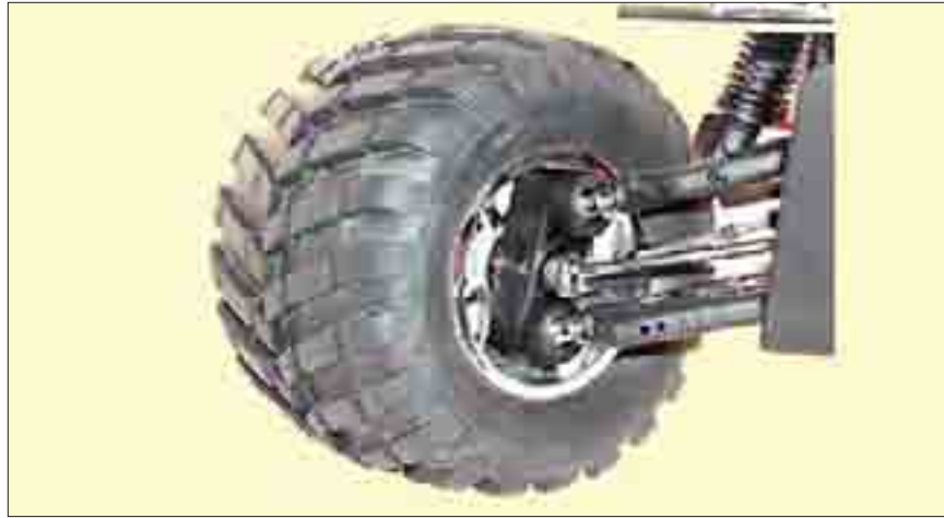
Truck suspension system : Front Pivot ball suspension soaks up the bumps and provides unmatched adjustability. Chrome 8 mm CVA joints give added strength.
