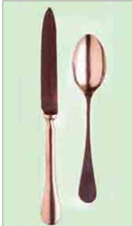
Stainless steel was invented in 1913 by British metallurgist Harry Brearley (1871-1948). He made a steel containing 13 per cent chromium. The new alloy proved to be highly resistant to corrosion: chromium reacts with oxygen in the air to form a tough, protective film which renews itself if the metal is scratched.
