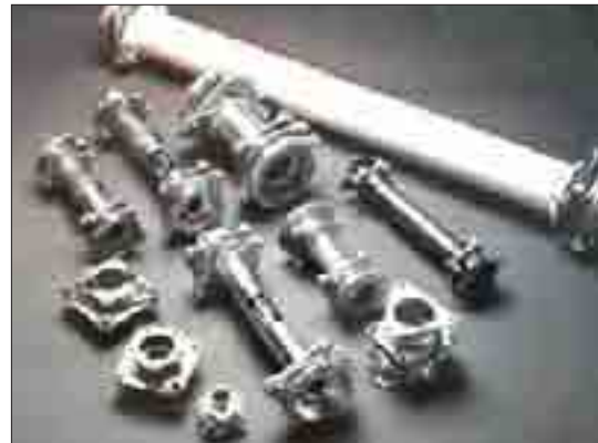
Helicopter driveline couplings.
