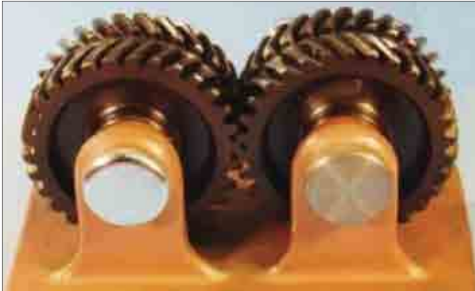
The picture shows double helical gears which are also called herringbone gears.
