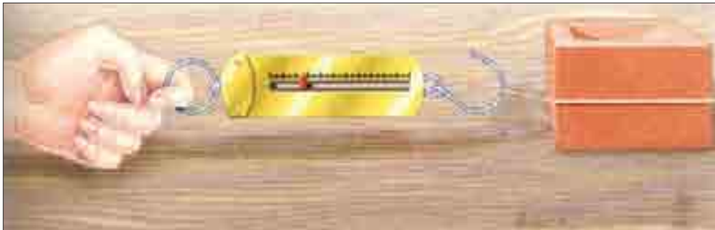
The pointer of this spring gauge shows the tension in the hook as the brick is pulled along.
