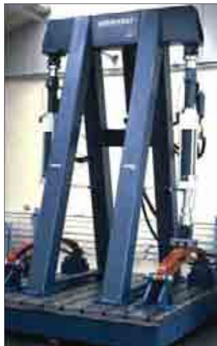
Leaf spring fatigue testing system.
