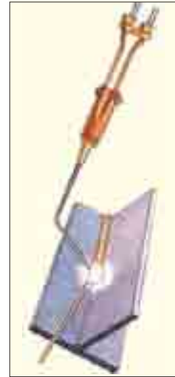
Soldering is done by melting a metal which melts at a lower temperature than the metal that is soldered.
