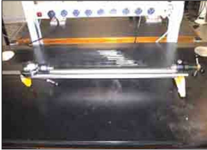
This equipment is used to determine the crippling load for axially loaded long struts.
