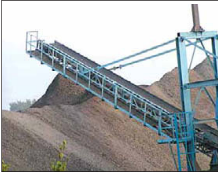
In the above conveyor belt is used to transport material as well as to drive the rollers
