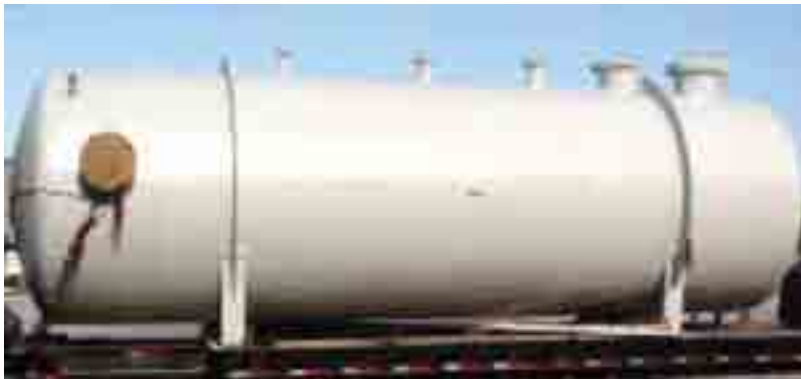
This vessel holds oil at high pressure.
