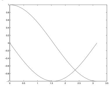
Notice that y not only contains the solution  $z_1(t)$  but also its derivative  $(z_2(t))$ . The exact solution here is  $\cos t$  (and consequently its derivative is  $-\sin t$ ). This technique can be used equally for non-autonomous systems (that is involving t explicitly). At this stage we will not consider all the options which are available to use when using these methods: however we merely mention that using the ode routines one can set the absolute and relative errors.
