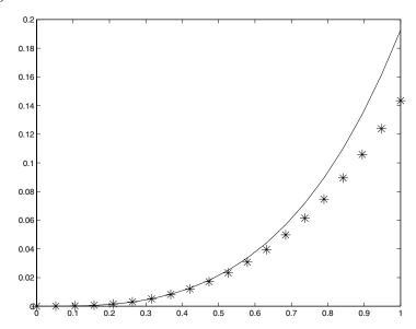
The numerical solution does reasonably initially: however as t increases the solution diverges.
