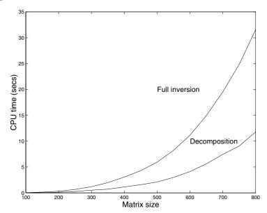
where the upper curve is the method using the construction of the inverse. In fact both of these curves grow like the size of the matrix to the power 3, but the lower one has a smaller constant of proportionality. Matrix inversion (and multiplication) is very expensive and any symmetry or special properties of a
