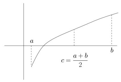
This must either be positive or negative (or if we are very lucky zero). In which case f(c) will have the same sign as either f(a) or f(b). The new interval can then be defined as c and whichever end of the previous interval represents a change in sign of the function.
