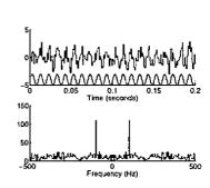
The top trace in the top plot is the noisy data, and the bottom trace is the original pure sinusoid. The lower plot clearly shows the frequency at 100 Hz.
