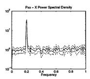
The frequency scale is normalised to the Nyquist frequency. The middle line is the PSD estimate and the two dashed lines are the 95% confidence intervals. Typing help spectrum reveals that there are many parameters that you can adjust when calculating the power spectrum. MATLAB's spectrum function uses the Welch method of PSD estimation, which divides a long signal into a number of smaller blocks, calculates
