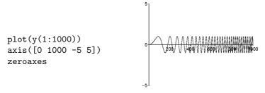
The frequency content of this signal as a function of time can be calculated using the specgram function. This function uses the Short Time Fourier Transform (STFT) technique. The STFT chops up the signal into a series of short segments and calculates the FFT of each segment. Each FFT becomes the estimate of the frequency content at that time. For our example we can get a quick display by typing:
