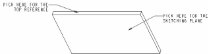
Figure 13 Orientation references for sketching the slot feature.
