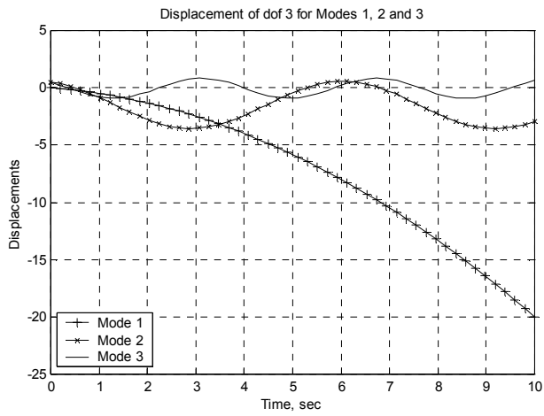
Figure 9.7: Displacements of mass 3 for all three modes of vibration.
