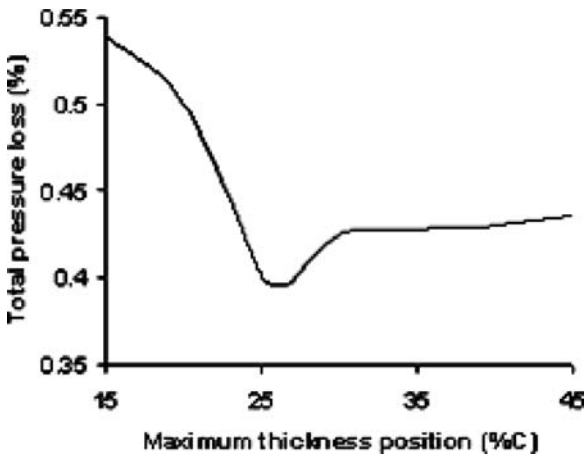
Figure 9: Total pressure losses and maximum thickness location.
