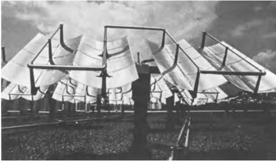
Fig. 56. Front view of a double axis tracking collector
