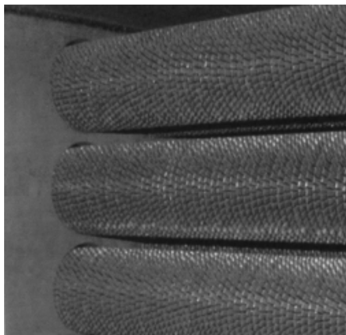
Figure 9-40. Finned tube economizer
