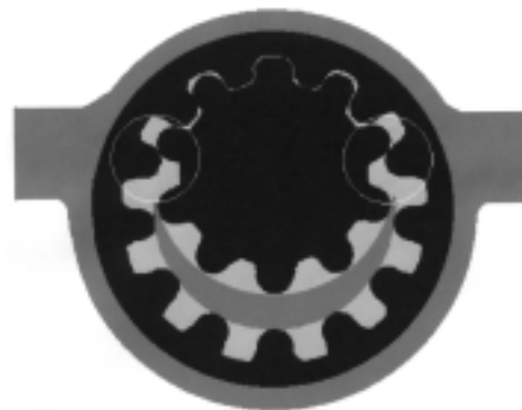
Figure 9-82. Crescent gear pump
