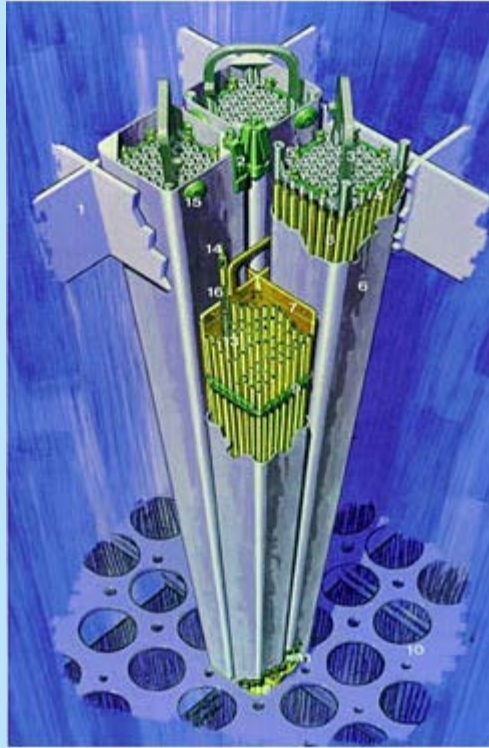
Fig.7 BWR/6 Fuel assemblies & control rod module
