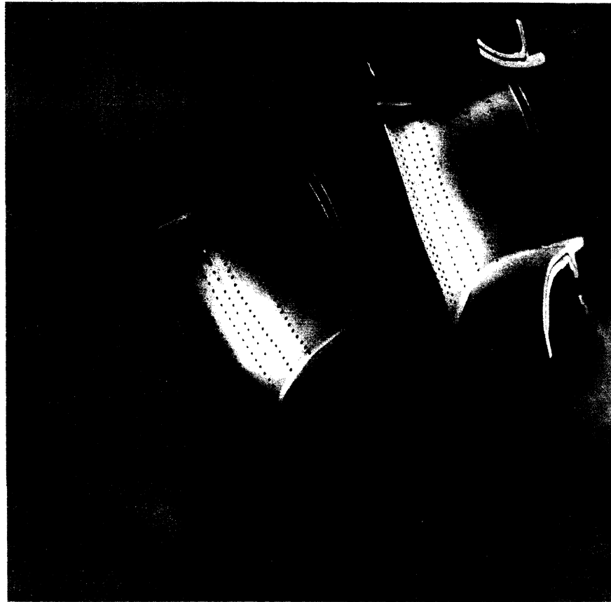
Figure 8.17 Film Cooling on a Rolls-Royce nozzle inlet guide (courtesy of Rolls-Royce).
