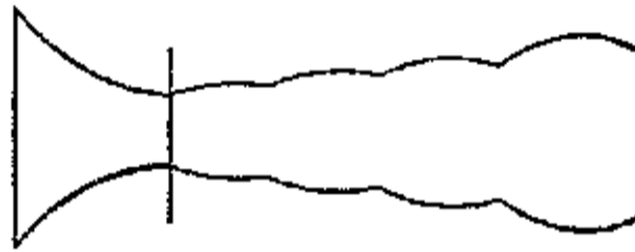
FIG. 20. Shape of jet discharged from a converging nozzle with subcritical back pressure.
