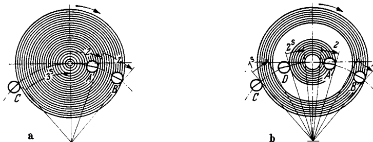
FIG. 248. Surfacing with a turret head of the type (Fig. 246). a—Surfacing over a large diameter. The tools A and B are roughing one half (1 and 2) each of the surface and tool C comes out to complete finishing operations (3). b—Surfacing of two separate concentric annular faces. The tools A and B are roughing the two faces (1 and 2) simultaneously, and the tools C and D are afterwards finishing the same faces (1' and 2') simultaneously.
