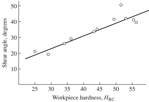
Fig. 17.62 Variation of shear angle versus workpiece hardness for tests of Figs. 17.60 and 17.61. (after Matsumoto et al., 1984)
