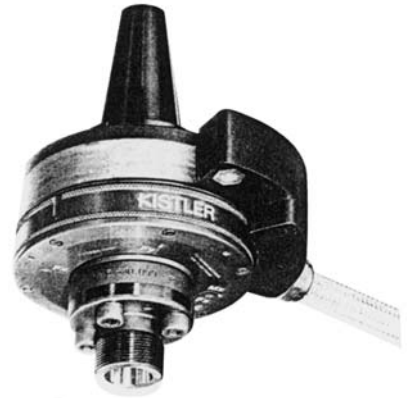
Fig. 7.32 Rotating quartz four-component dynamometer with transfer of data by telemetry. [Specifications: maximum speed, 10,000 rpm; range for F_z , -4.5 to +4.5 \text{ klb} ( -20 to 20 \text{ kN} ); range for M_z , -147.5 to +147.5 \text{ lb-ft} ( -200 to 200 \text{ Nm} ); threshold for <0.9 \text{ lb} ( <4 \text{ N} ); nat. freq. 1 \text{ kHz} ; weight 11 \text{ lb} ( 5 \text{ kg} ).] (after Kistler Instrument Corp.)
