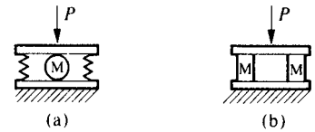
Fig. 7.11 Schematic views showing two types of dynamometers.
